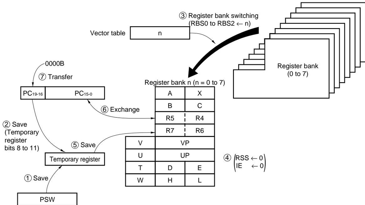
The RETCS instruction is used to return from an interrupt that uses the context switching function. The RETCS instruction must specify the start address of the interrupt service program to be executed when that interrupt is acknowledged next. This interrupt service program start address must be in the base area.
