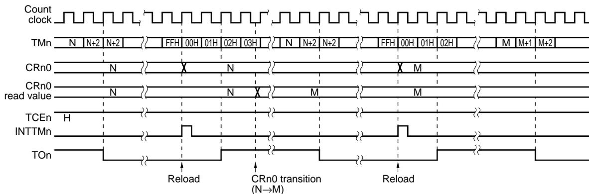
(c) When the CRn0 value changes from N to M during two clocks (00H, 01H) immediately after TMn overflows
