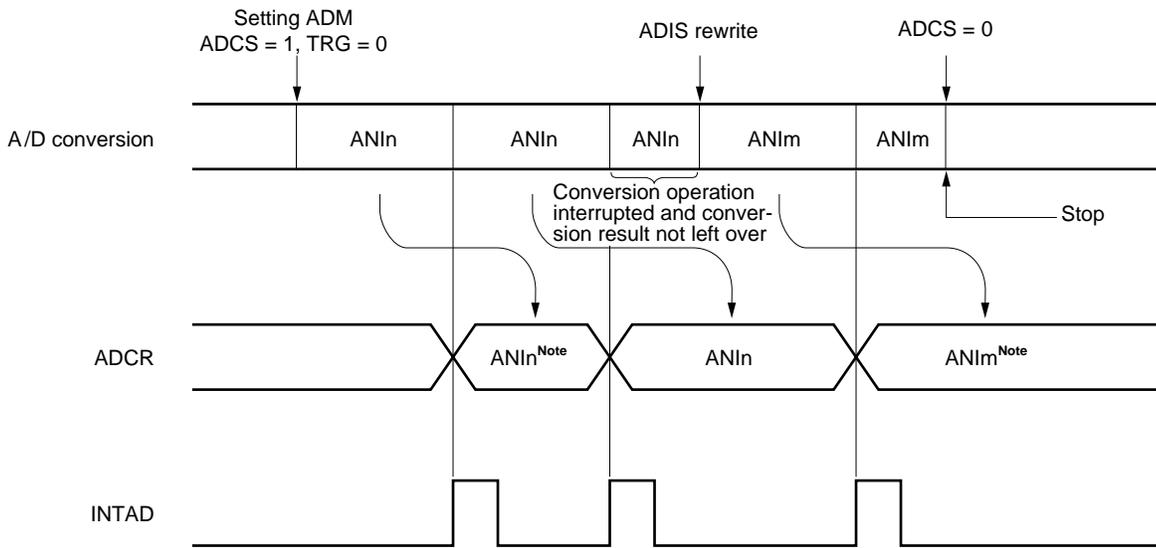
**Note** If bit 0 (ADCE) of the A/D converter mode register is not set to 1, the value of the first A/D conversion is undefined immediately after A/D conversion starts. Poll the A/D conversion end interrupt request (INTAD) and take measures such as discarding the first A/D conversion result.
