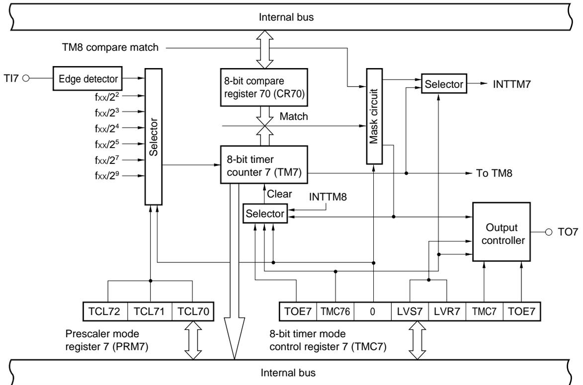
Figure 11-1. Block Diagram of 8-Bit Timer/Event Counter 7, 8 (2/2)
