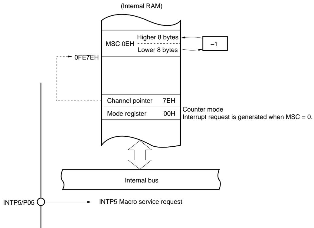
**Remark** The internal RAM addresses in the figure above are the values when the LOCATION 0H instruction is executed. When the LOCATION 0FH instruction is executed, 0F0000H should be added to the values in the figure.
