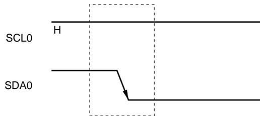
The start condition is output when bit 1 (STT0) of the I<sup>2</sup>C bus control register (IICC0) is set to 1 in the stop condition detection state (SPD0: when bit 0 in the I<sup>2</sup>C bus status register (IICS0) = 1). In addition, when the start condition is detected, bit 1 (STD0) in IICS0 is set to 1.
