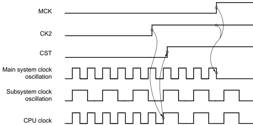
**(b) Operation when MCK is set during main system clock operation**
