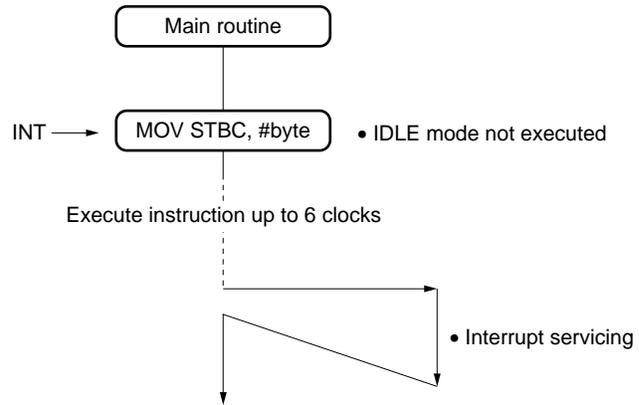
**(1) Releasing the IDLE mode by NMI input**
