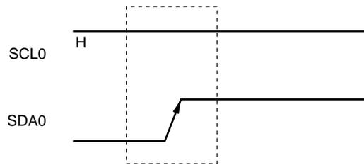
The stop condition is generated when bit 0 (SPT0) of the I<sup>2</sup>C bus control register (IICC0) is set to 1. And when the stop condition is detected, if bit 0 (SPD0) in the I<sup>2</sup>C bus status register (IICS0) is set to 1 and bit 4 (SPIE0) of IICC0 is also set to 1, INTIIC0 is generated.
