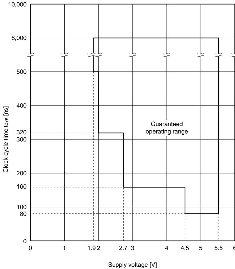
**Caution** The operating voltage of the  $\mu$ PD78F4216A and 78F4216AY rank K, E is  $2.7\text{ V} \leq V_{DD} \leq 5.5\text{ V}$ .
