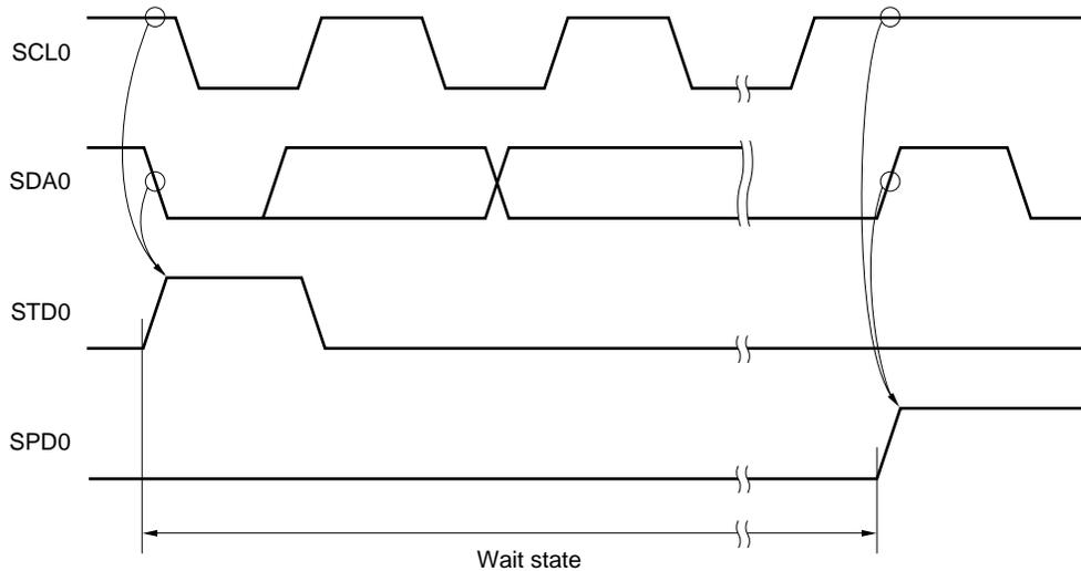
Figure 19-17 shows the communication reservation procedure.
