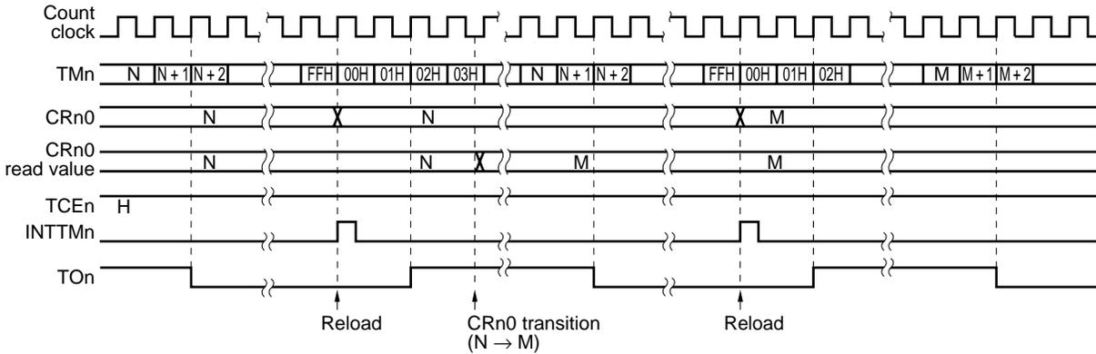
(c) When the CRn0 value changes from N to M during two clocks (00H, 01H) immediately after TMn overflows
