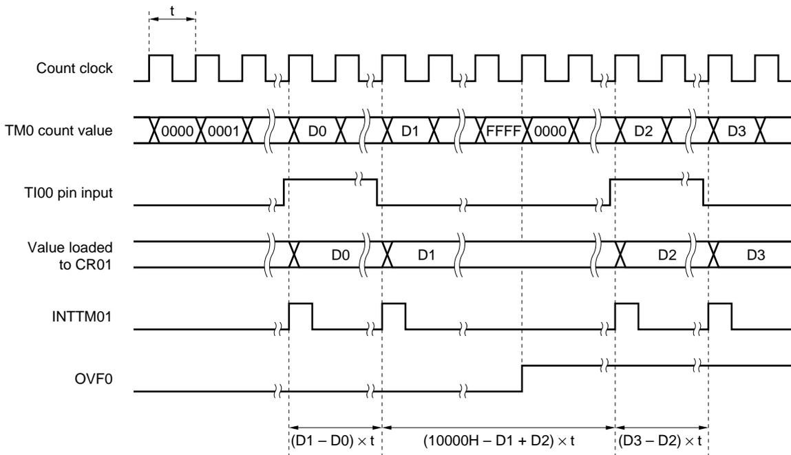
**Caution** For simplification purposes, delay due to noise elimination is not taken into consideration in the capture operation by TI00 pin input and in the interrupt request generation timing in the above figure. For a more accurate picture, refer to Figure 8-14 CR01 Capture Operation with Rising Edge Specified.
