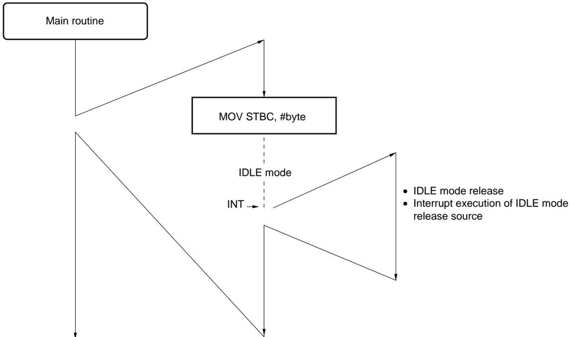
Figure 25-9. Operation After IDLE Mode Release (3/3)
