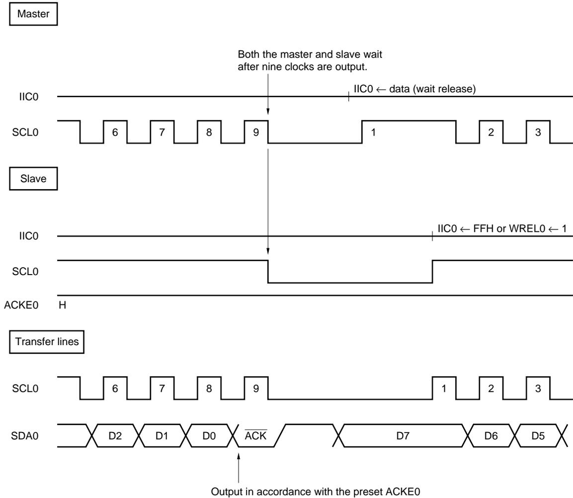
**Remark** ACKE0: Bit 2 in the I<sup>2</sup>C bus control register (IICC0)
