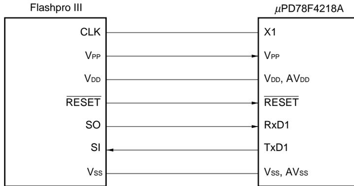
**Caution** Connect the V<sub>PP</sub> pin directly to V<sub>SS</sub> or pull down. For the pull-down connection, use of resistors with a resistance between 470 Ω and 10 kΩ is recommended.
