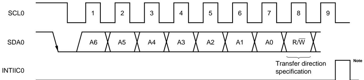
**Note** When data other than base address or extended code is received during slave operation, INTIIC0 is not generated.
