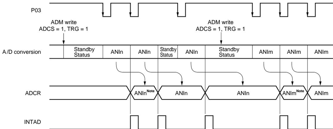
**Note** If bit 0 (ADCE) of the A/D converter mode register is not set to 1, the value of the first A/D conversion is undefined immediately after A/D conversion starts. Poll the A/D conversion end interrupt request (INTAD) and take measures such as discarding the first A/D conversion result.
