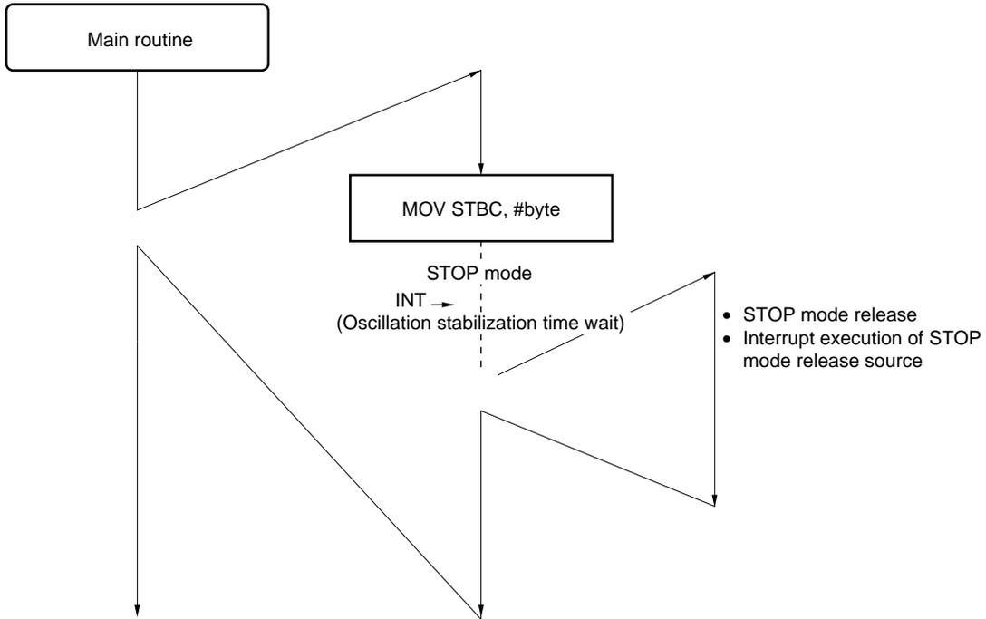
Figure 25-6. Operation After STOP Mode Release (3/3)
