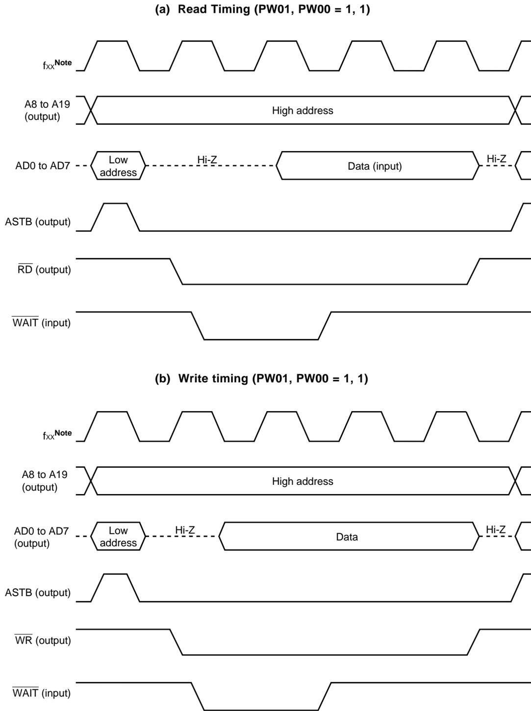
**Note** fxx: Main system clock frequency. This signal is only in the  $\mu$ PD784218A.
