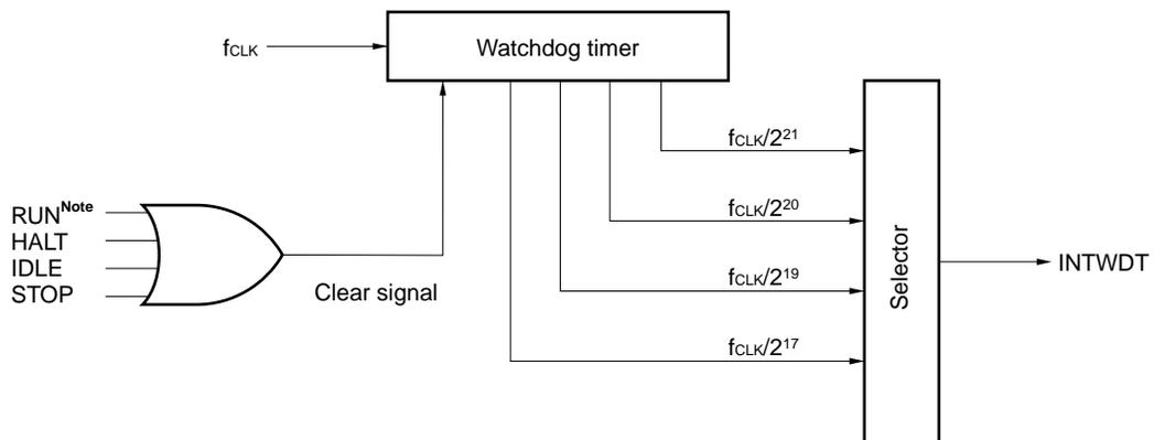
**Note** Write 1 to bit 7 (RUN) of the watchdog timer mode register (WDM).
