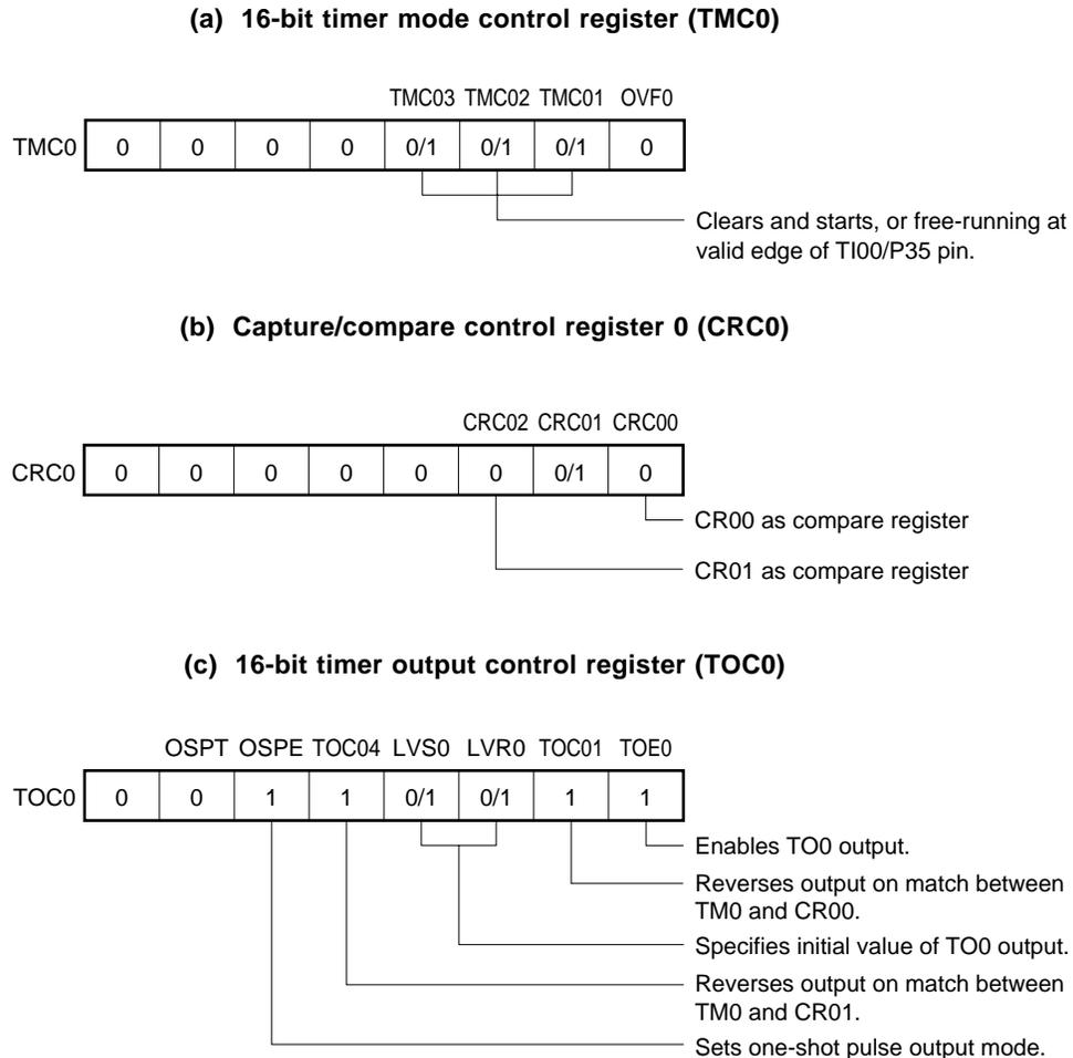
**Remark** 0/1: When these bits are reset to 0 or set to 1, the other functions can be used along with the one-shot pulse output function. For details, refer to **Figures 8-2, 8-3, and 8-4**.
