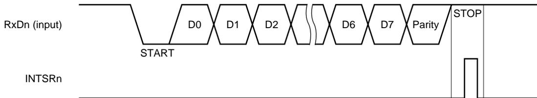
**Caution** Even when a receive error occurs, be sure to read the receive buffer register (RXBn). If RXBn is not read, an overrun error will occur during reception of the next data, and the reception error status will continue indefinitely.
