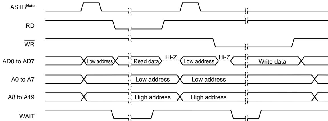
**Note** In the separate bus mode, the address strobe does not have to be used. However, the address strobe is output from the ASTB/P67 pin.
