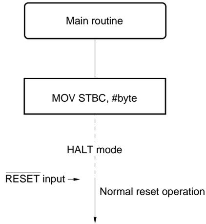
Figure 25-5. Operation After HALT Mode Release (2/4)
