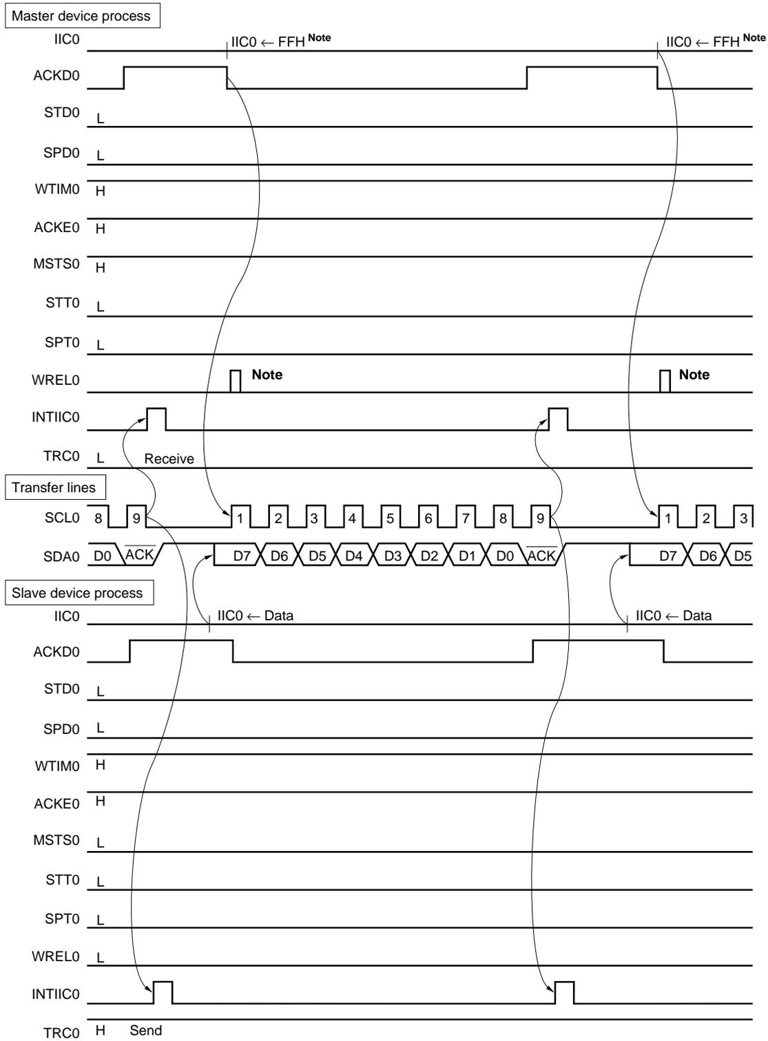
**Note** Release the slave wait by either IIC0 ← FFH or setting WRELO.
