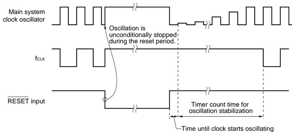
To prevent erroneous operation caused by noise, a noise eliminator based on an analog delay is incorporated at the  $\overline{\text{RESET}}$  input pin.
