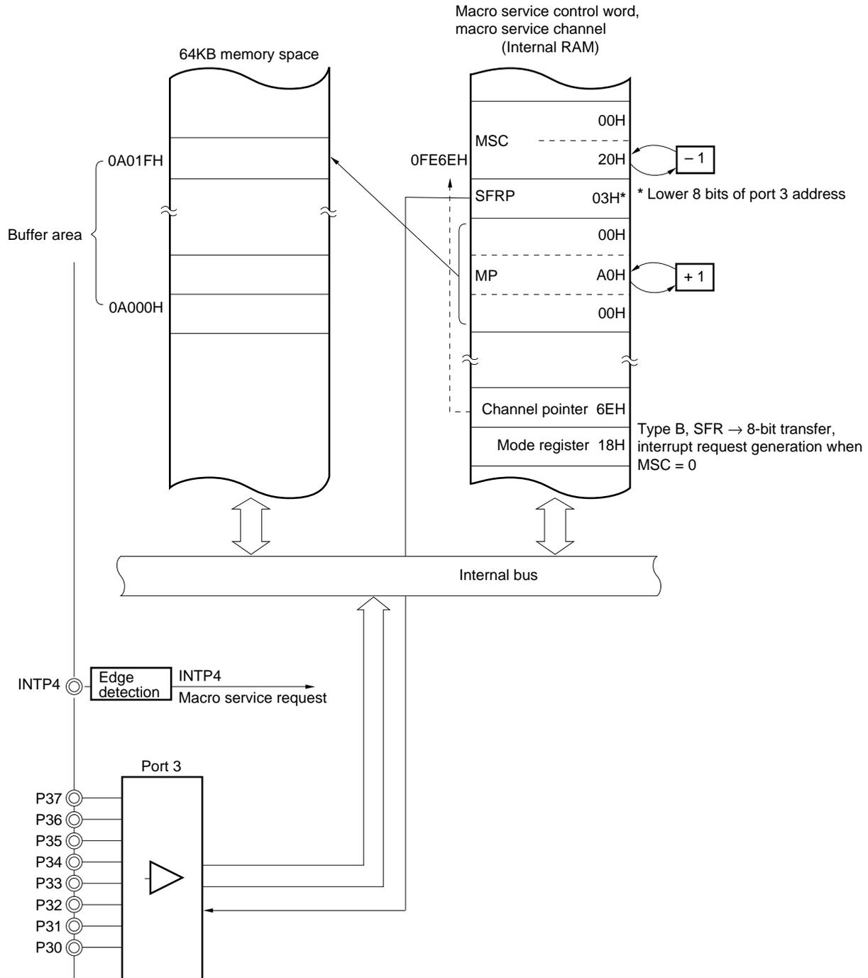
**Remark** Macro service channel addresses in the figure are the values when the LOCATION 0H instruction is executed. When the LOCATION 0FH instruction is executed, 0F0000H should be added to the values in the figure.
