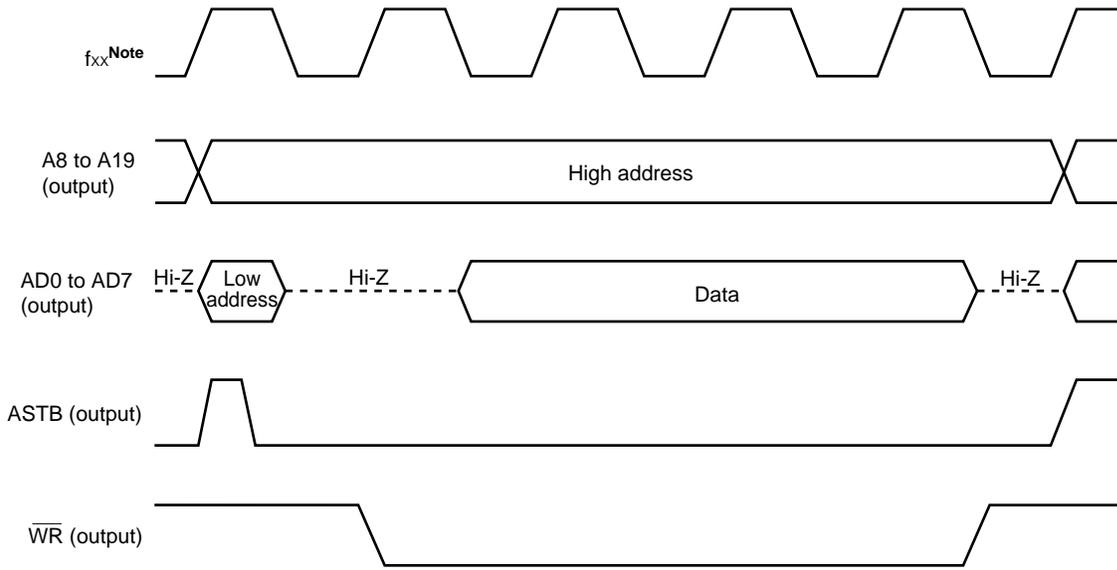
**Note** f<sub>xx</sub>: Main system clock frequency. This signal is only in the  $\mu$ PD784218A.
