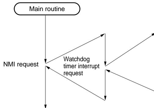
Figure 23-10. Non-Maskable Interrupt Request Acknowledgement Operations (2/2)
