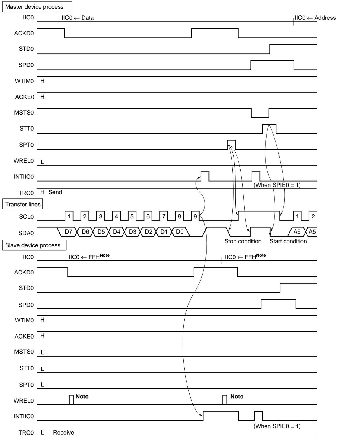
**Note** Release the slave wait by either IIC0 ← FFH or setting WRELO.
