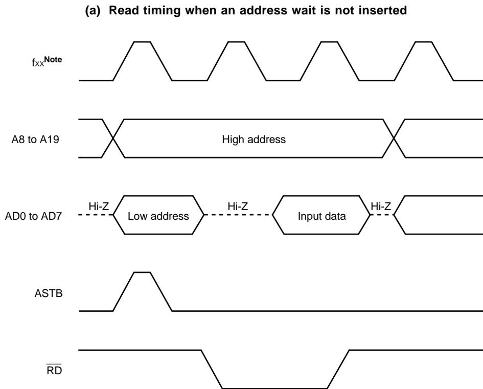
**Note**  $f_{xx}$ : Main system clock frequency. This signal is only in the  $\mu$ PD784218A.
