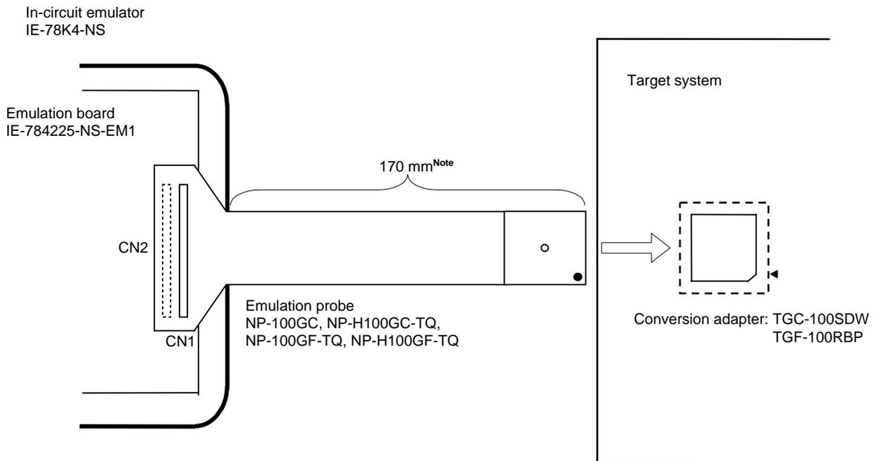
**Note** Distance when the NP-100GC or NP-100GF-TQ is used. When the NP-H100GC-TQ or NP-H100GF-TQ is used, the distance is 370 mm.
