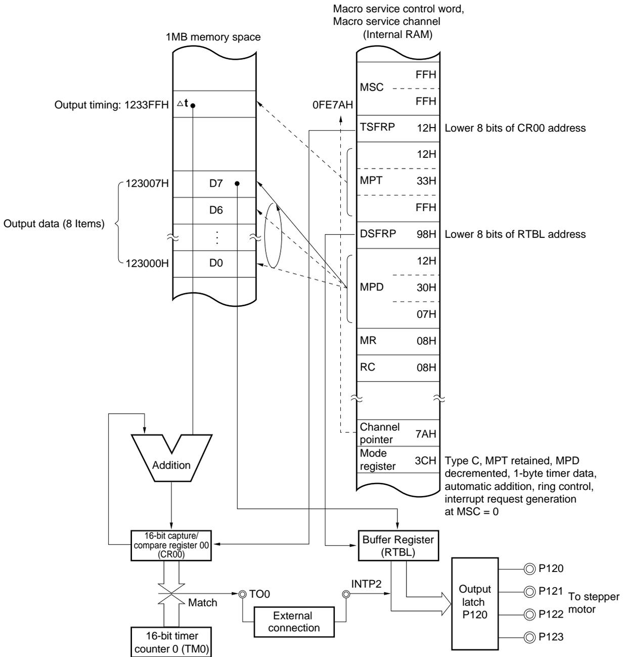
**Remark** Internal RAM addresses in the figure are the values when the LOCATION 0H instruction is executed. When the LOCATION 0FH instruction is executed, 0F0000H should be added to the values in the figure.
