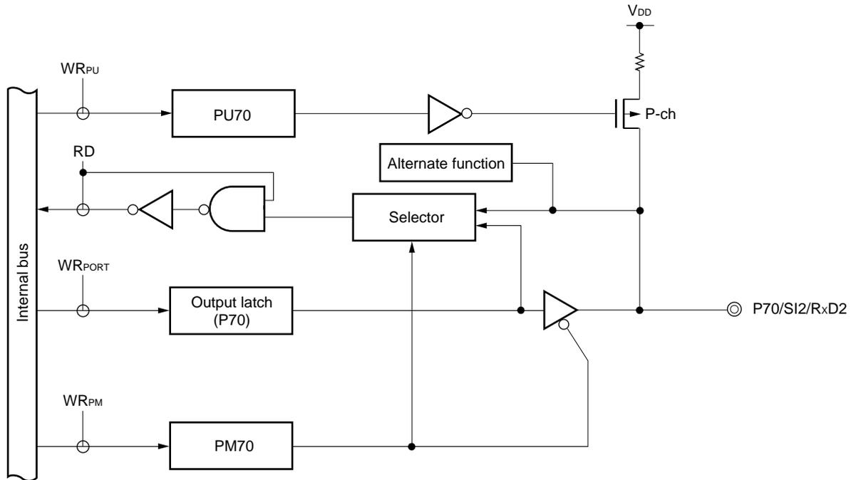
PU: Pull-up resistor option register
