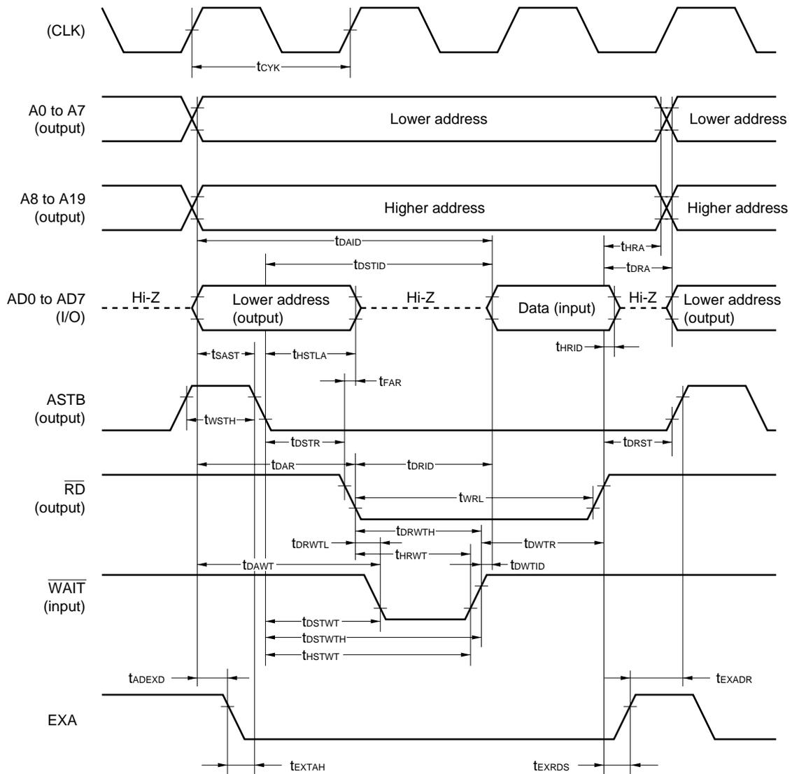
**Remark** The signal is output from pins A0 to A7 when P80 to P87 are unused.
