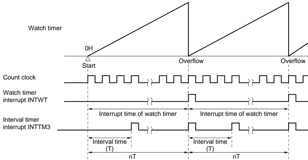
**Caution** When enabling operation of the watch timer mode control register (WTM), watch timer, and 5-bit counter, the time until the first watch timer interrupt request (INTWT) is generated is not exactly the same time as set by bits 4 to 6 of WTM (WTM4 to WTM6). This is because the 5-bit counter starts counting 1 cycle after 9-bit prescaler output. Following the first INTWT generation, the INTWT signal is generated at the set interval time.
