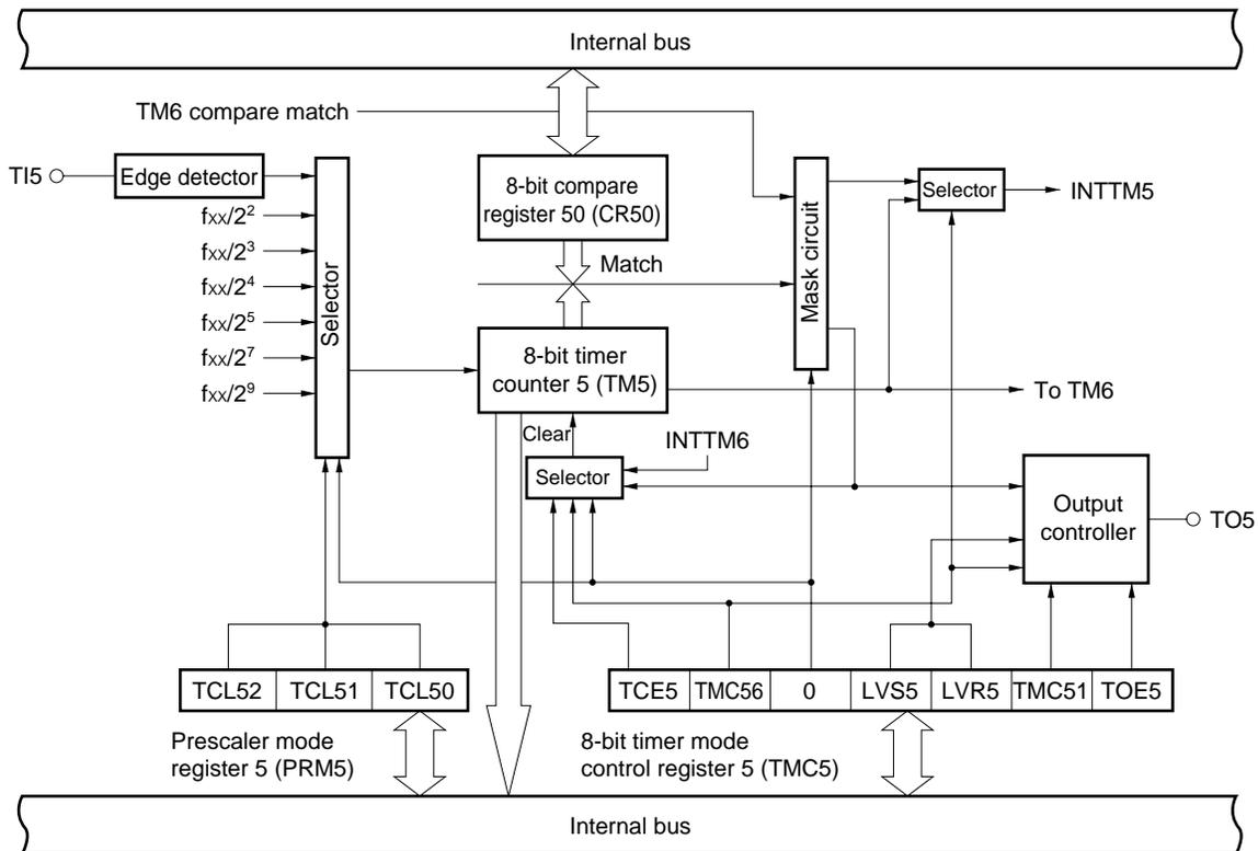
Figure 10-1. Block Diagram of 8-Bit Timer/Event Counter 5, 6 (2/2)
