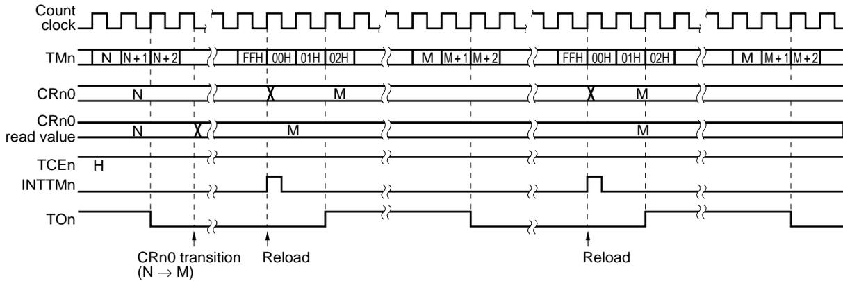
(b) When the CRn0 value changes from N to M after TMn overflows
