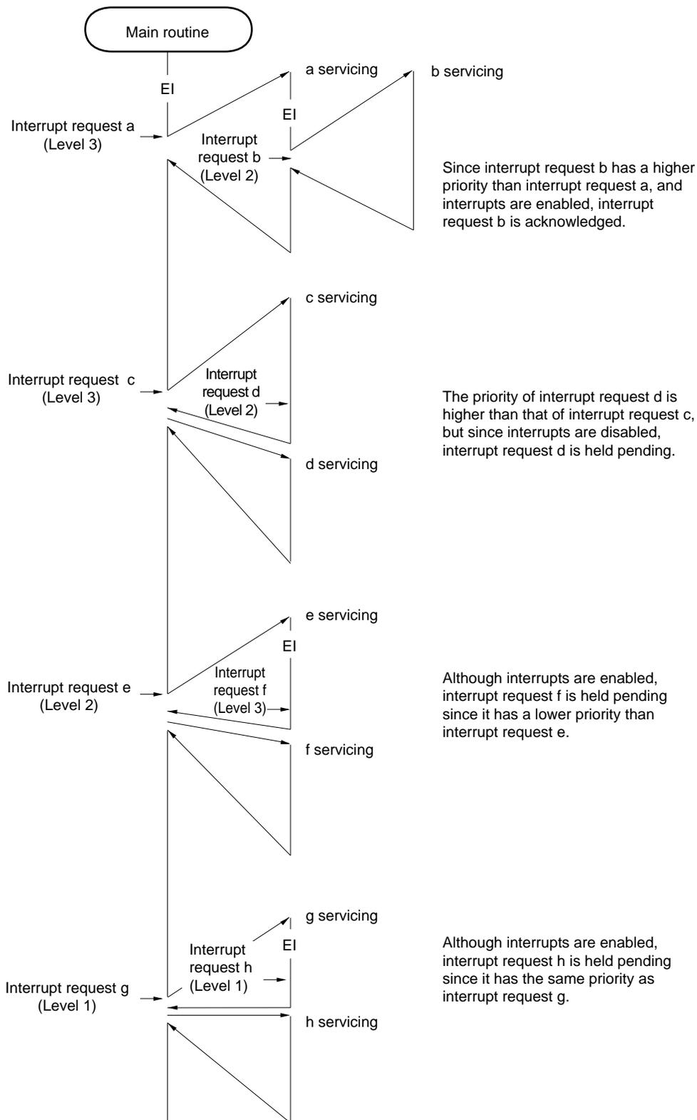
Figure 23-14. Examples of Servicing When Another Interrupt Request Is Generated During Interrupt Service (2/3)
