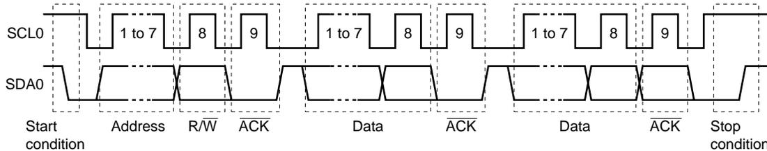
The master outputs the start condition, slave address, and stop condition.
