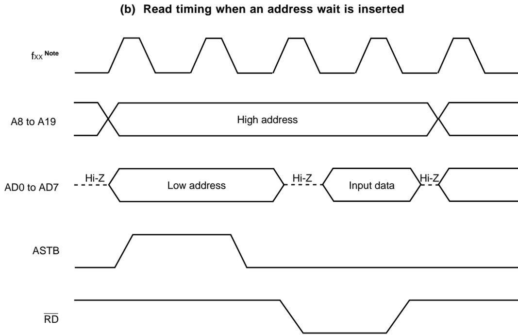
**Note** fxx: Main system clock frequency. This signal is only in the  $\mu$ PD784218A.
