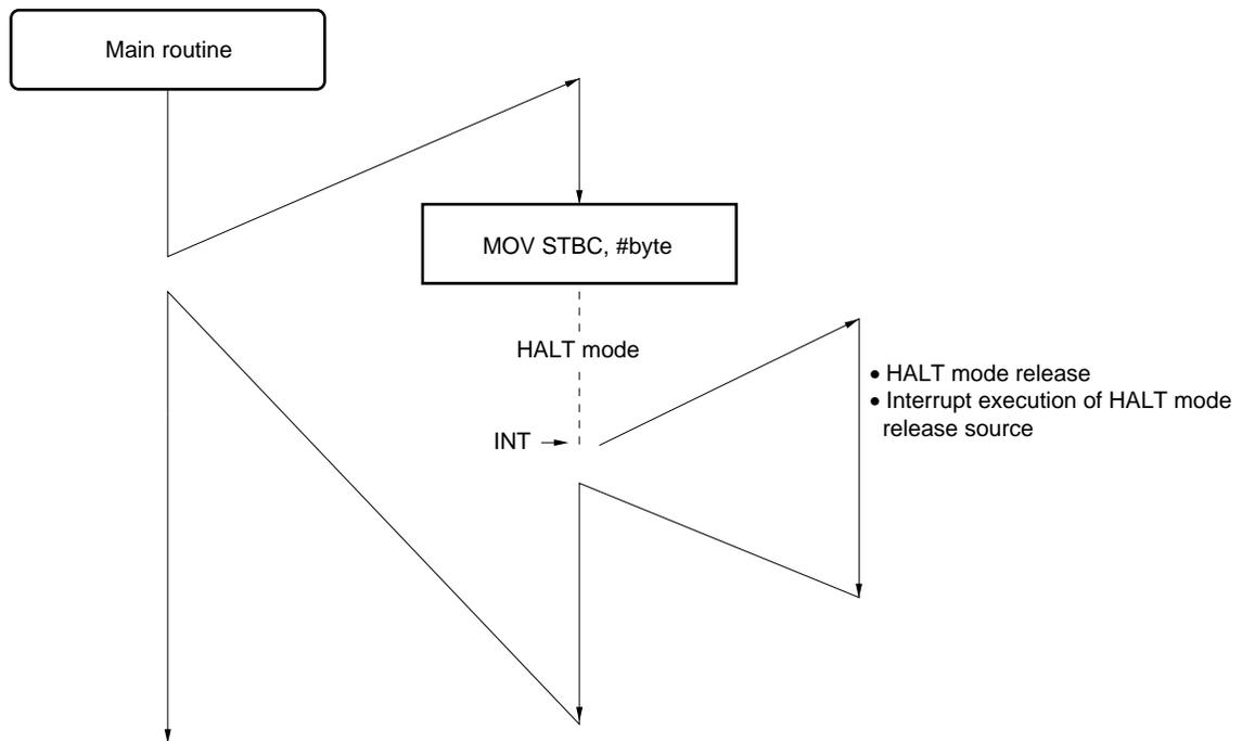
Figure 25-5. Operation After HALT Mode Release (3/4)
