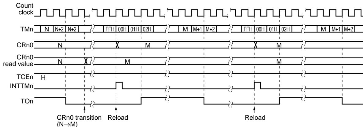
(b) When the CRn0 value changes from N to M after TMn overflows
