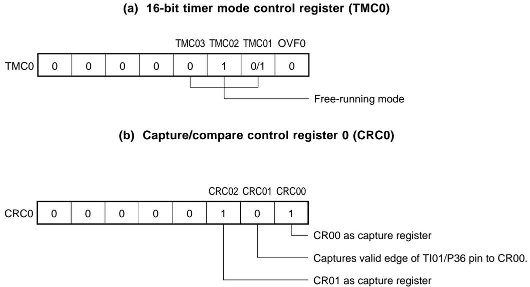
**Remark** 0/1: When these bits are reset to 0 or set to 1, the other functions can be used along with the pulse width measurement function. For details, refer to **Figures 8-2** and **8-3**.
