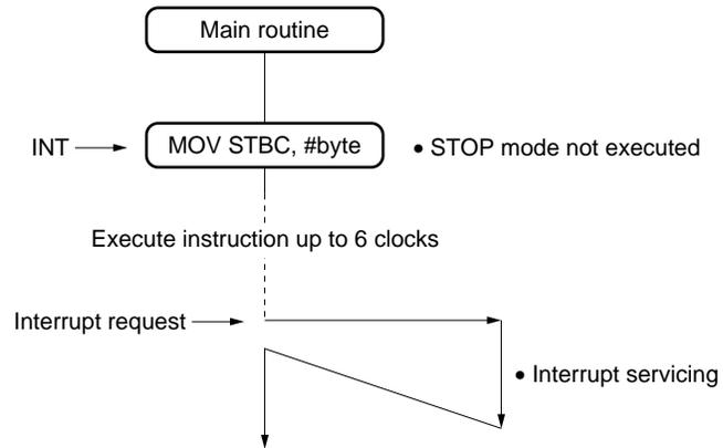
**(1) Releasing the STOP mode by NMI input**
