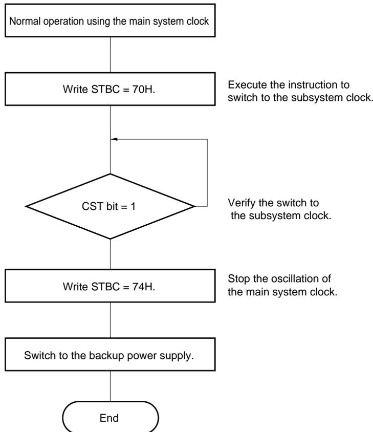
Figure 25-12. Setting Timing for Subsystem Clock Operation
