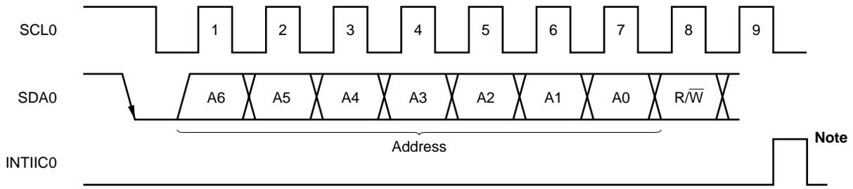
**Note** When data other than base address or extended code was received during slave operation, INTIIC0 is not generated.
