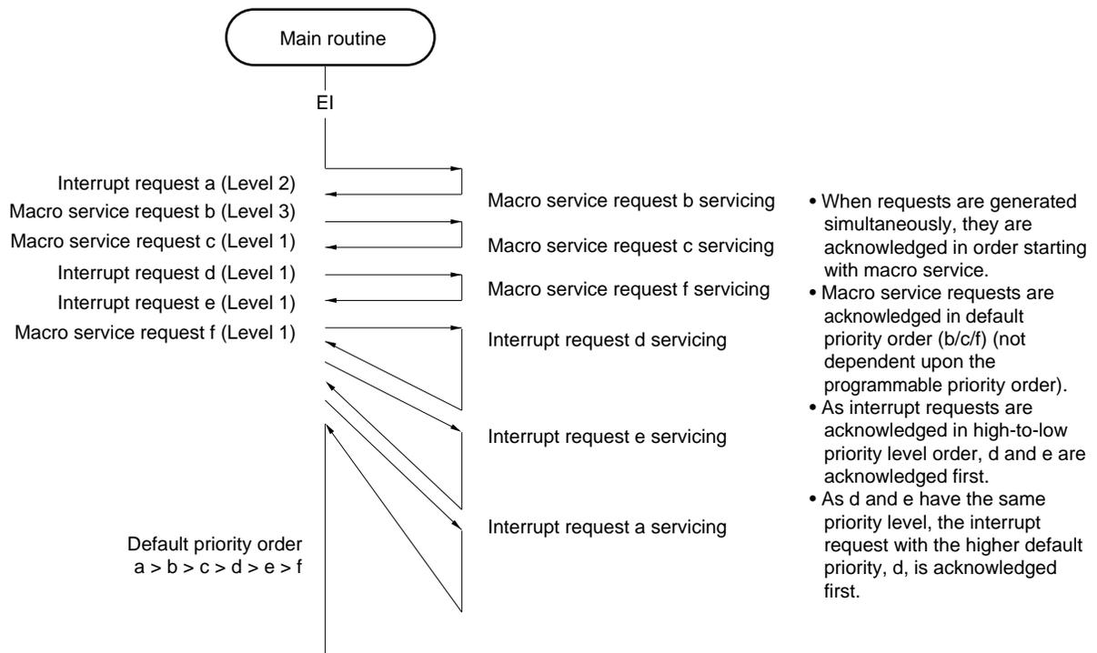
**Remark** “a” to “f” in the figure above are arbitrary names used to differentiate between the interrupt requests and macro service requests.
