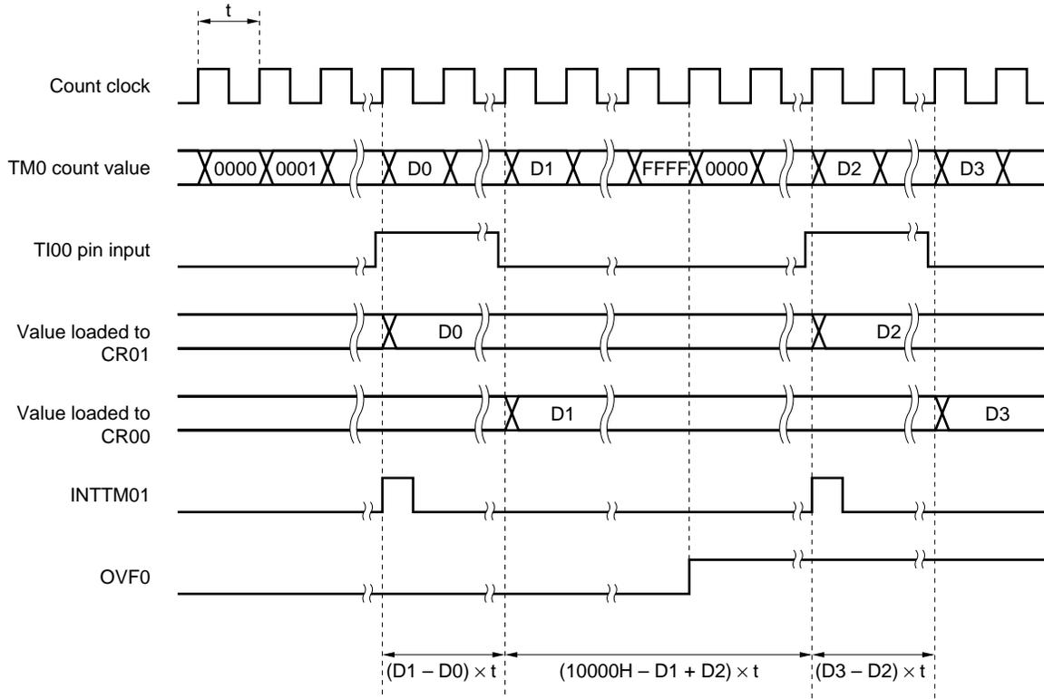
**Caution** For simplification purposes, delay due to noise elimination is not taken into consideration in the capture operation by TIO0 pin input and in the interrupt request generation timing in the above figure. For a more accurate picture, refer to Figure 8-14 CR01 Capture Operation with Rising Edge Specified.
