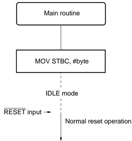
Figure 25-9. Operation After IDLE Mode Release (2/3)
