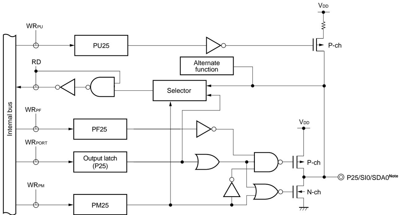
**Note** The SDA0 pin applies only to the  $\mu$ PD784216AY, 784218AY Subseries.
