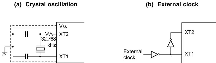
**Cautions 1.** When using a main system clock oscillator and a subsystem clock oscillator, carry out wiring in the broken line area in Figures 4-6 and 4-7 to prevent any effects from wiring capacities.
