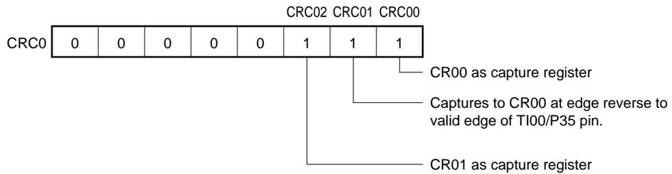
**Remark** 0/1: When these bits are reset to 0 or set to 1, the other functions can be used along with the pulse width measurement function. For details, refer to **Figures 8-2** and **8-3**.
