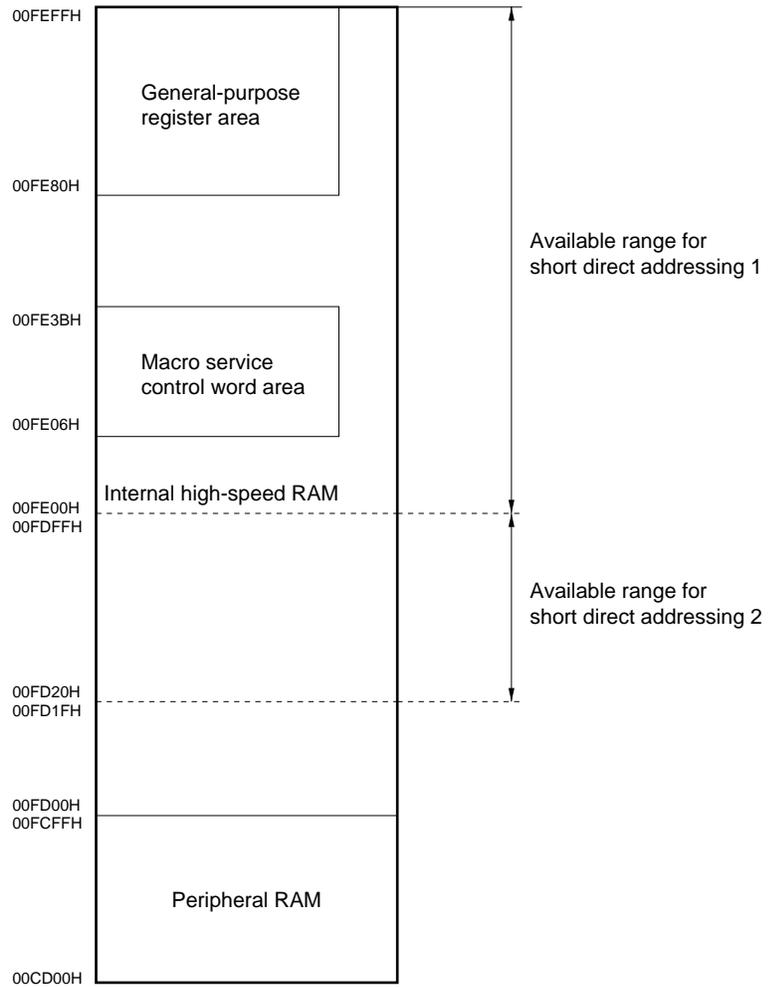
**Remark** The addresses in the figure are the values when the LOCATION 0H instruction is executed. When the LOCATION 0FH instruction is executed, 0F0000H is added to the above values.
