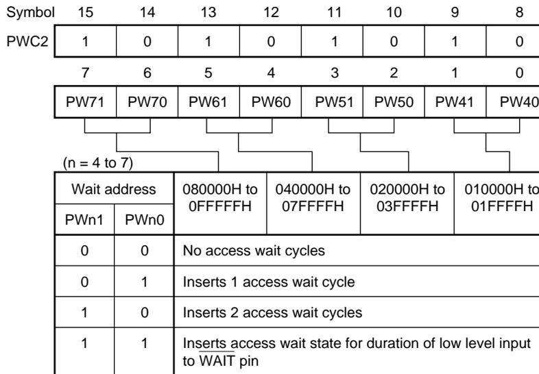
**Remark** Insertion of wait cycles is controlled on the entire address space (except the peripheral RAM area).
