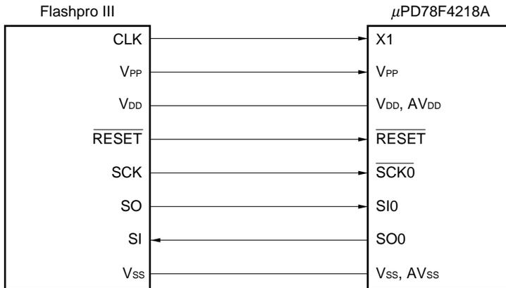
**Figure 28-3. Connection of Flashpro III in 3-Wire Serial I/O Mode (When Using Handshake)**
