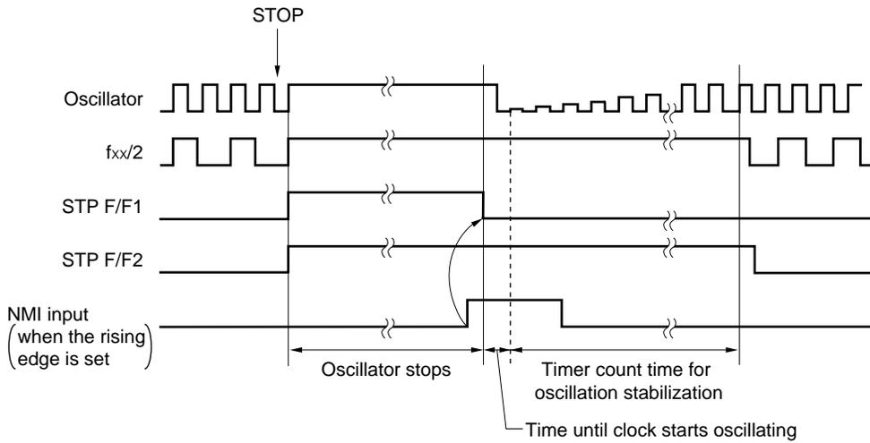
**(2) Releasing the STOP mode by INTP0 to INTP6 input, watch timer interrupt, and key return interrupt**
