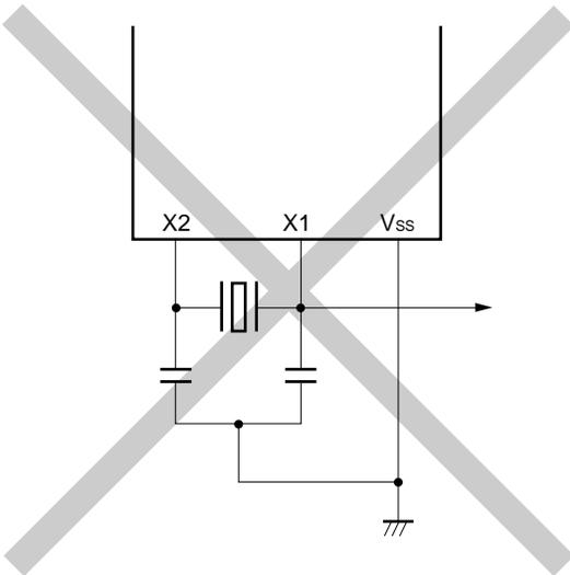
**Remark** When using a subsystem clock, replace X1 and X2 with XT1 and XT2, respectively. Also, insert resistors in series on the XT2 side.
