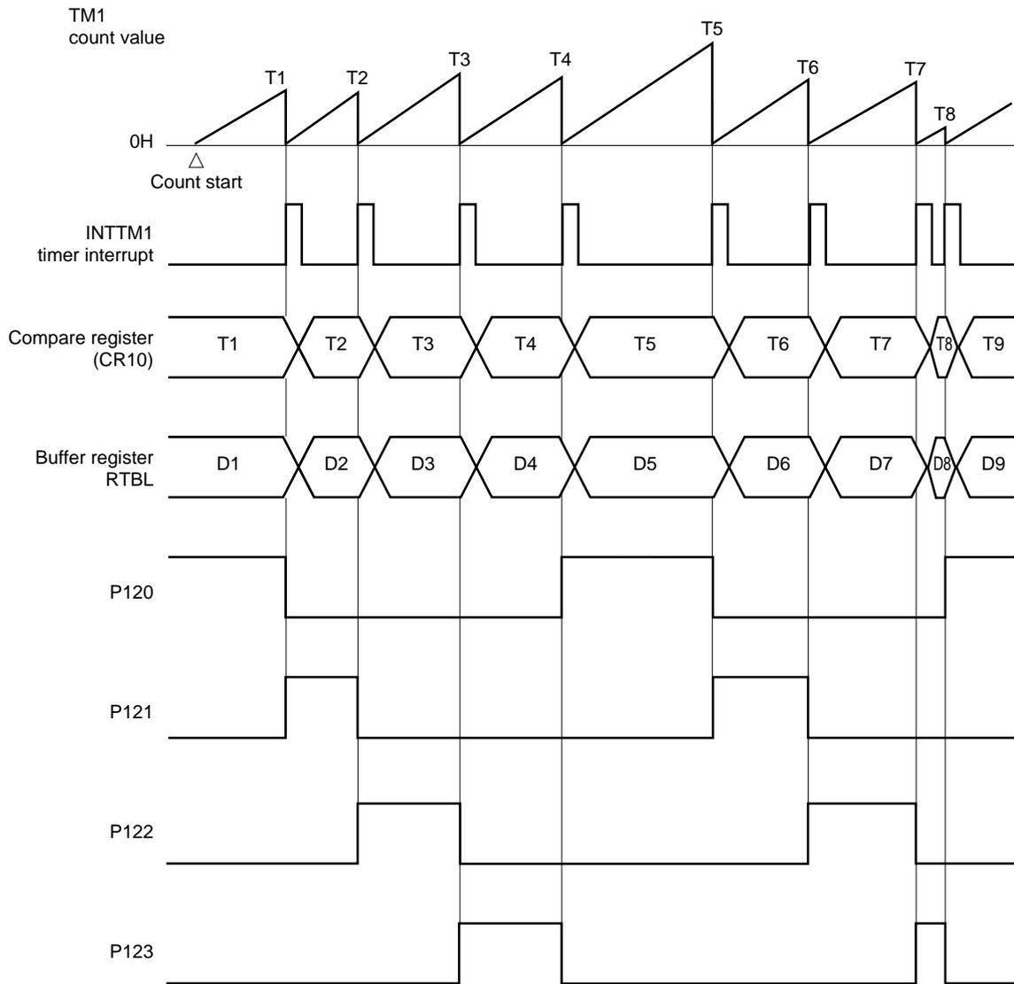
**(b) Examples of use of automatic addition control and ring control****(i) Automatic addition control**
