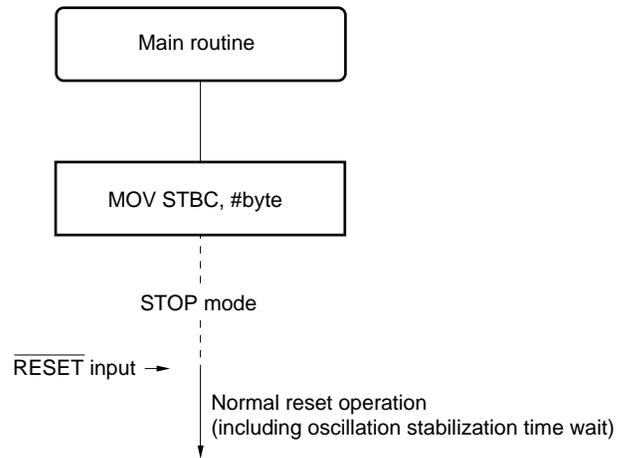
Figure 25-6. Operation After STOP Mode Release (2/3)
