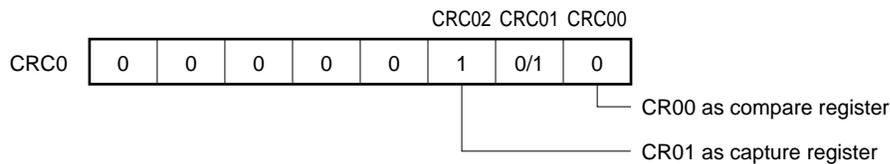
**Remark** 0/1: When these bits are reset to 0 or set to 1, the other functions can be used along with the pulse width measurement function. For details, refer to **Figures 8-2** and **8-3**.
