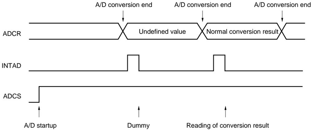
**(10) Reading A/D conversion result register (ADCR)**
