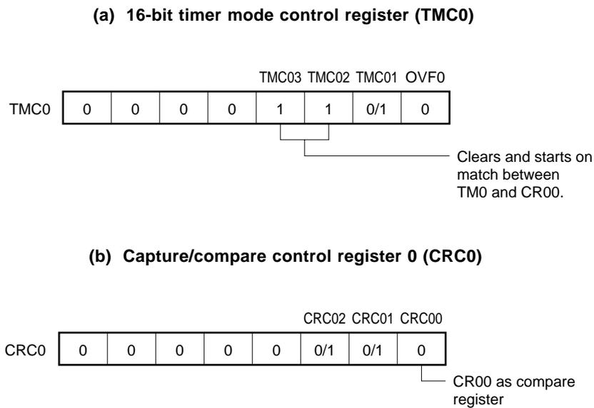
**Remark** 0/1: When these bits are reset to 0 or set to 1, the other functions can be used along with the interval timer function. For details, refer to **Figures 8-2** and **8-3**.
