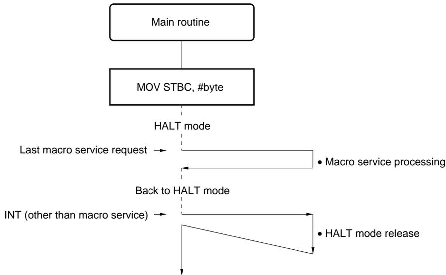
Figure 25-5. Operation After HALT Mode Release (4/4)
