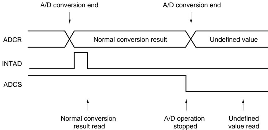
**Figure 14-13. Conversion Result Read Timing (When Conversion Result Is Normal)**
