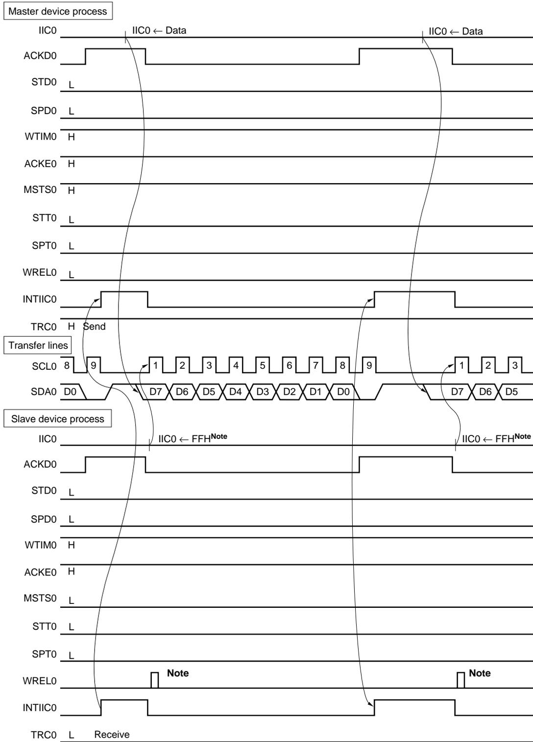
**Note** Release the slave wait by either IIC0 ← FFH or setting WREL0.
