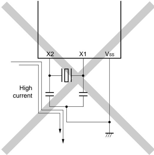
(d) Current flows through the ground line of the oscillator (potential at points A, B, and C fluctuate)
