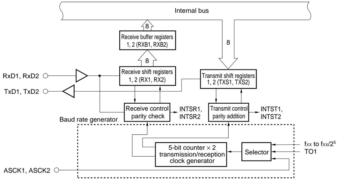
**(1) Transmit shift registers (TXS1, TXS2)**
