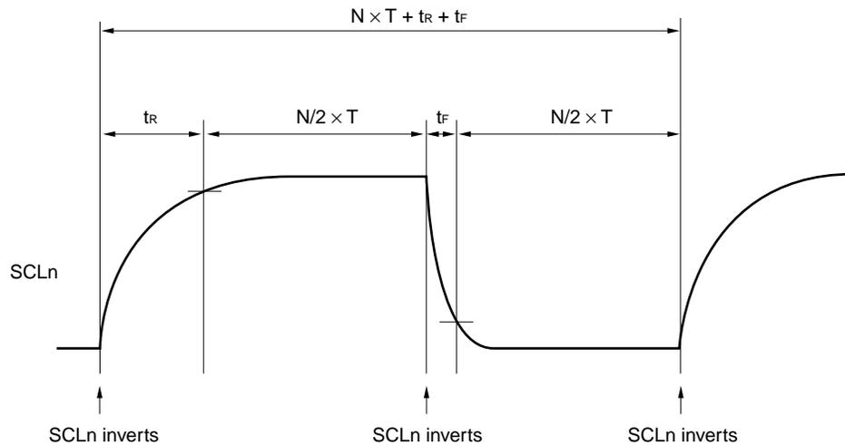
$$\text{IIC clock frequency: } f_{\text{SCL}} = 1/(N \times T + t_r + t_f)$$
