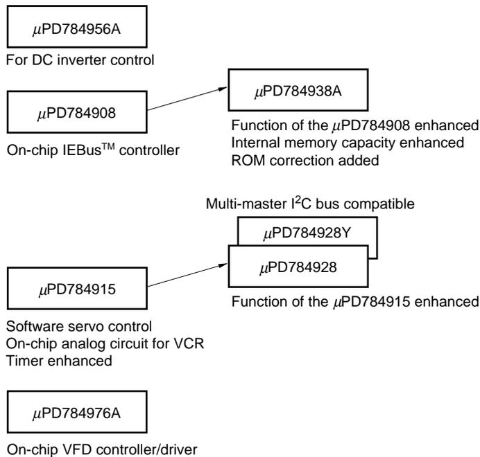
**Remark** VFD (Vacuum Fluorescent Display) is referred to as FIP™ (Fluorescent Indicator Panel) in some documents, but the functions of the two are the same.
