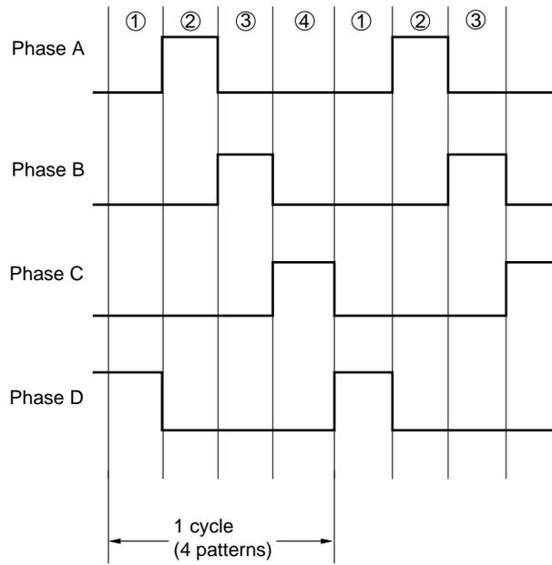
Figure 23-35. 1-2-Phase Excitation of 4-Phase Stepping Motor
