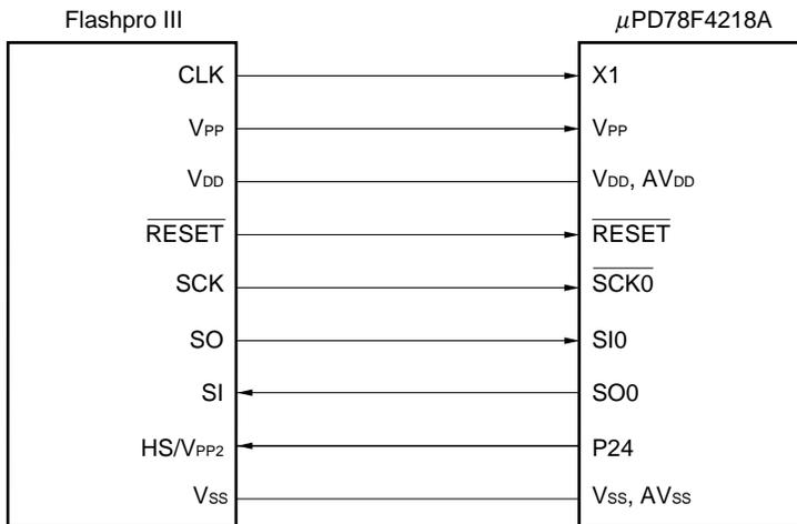
**Figure 28-4. Connection of Flashpro III in UART Mode
