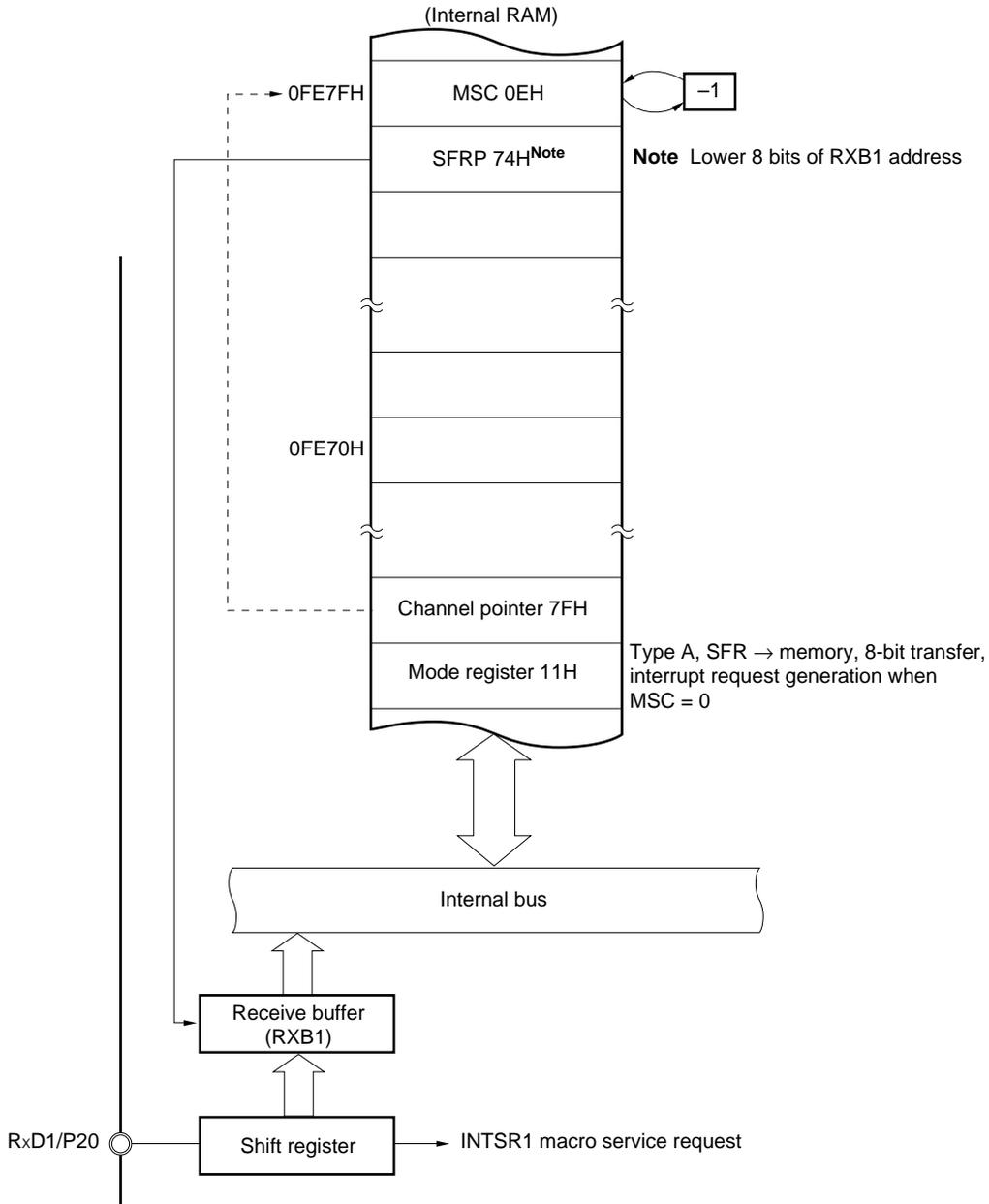
**Remark** Addresses in the figure are the values when the LOCATION 0H instruction is executed. When the LOCATION 0FH instruction is executed, 0F0000H should be added to the values in the figure.
