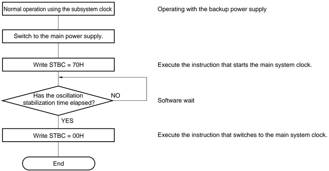
Figure 25-14. Timing for Restoring Main System Clock Operation
