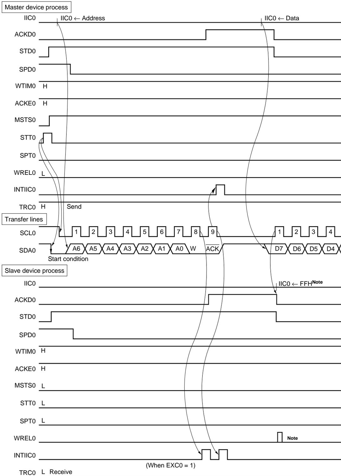
**Note** Release the slave wait by either IIC0 ← FFH or setting WRELO.
