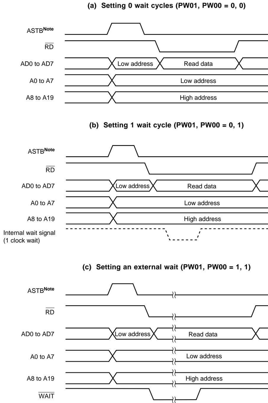
**Note** In the separate bus mode, the address strobe does not have to be used. However, the address strobe is output from the ASTB/P67 pin.
