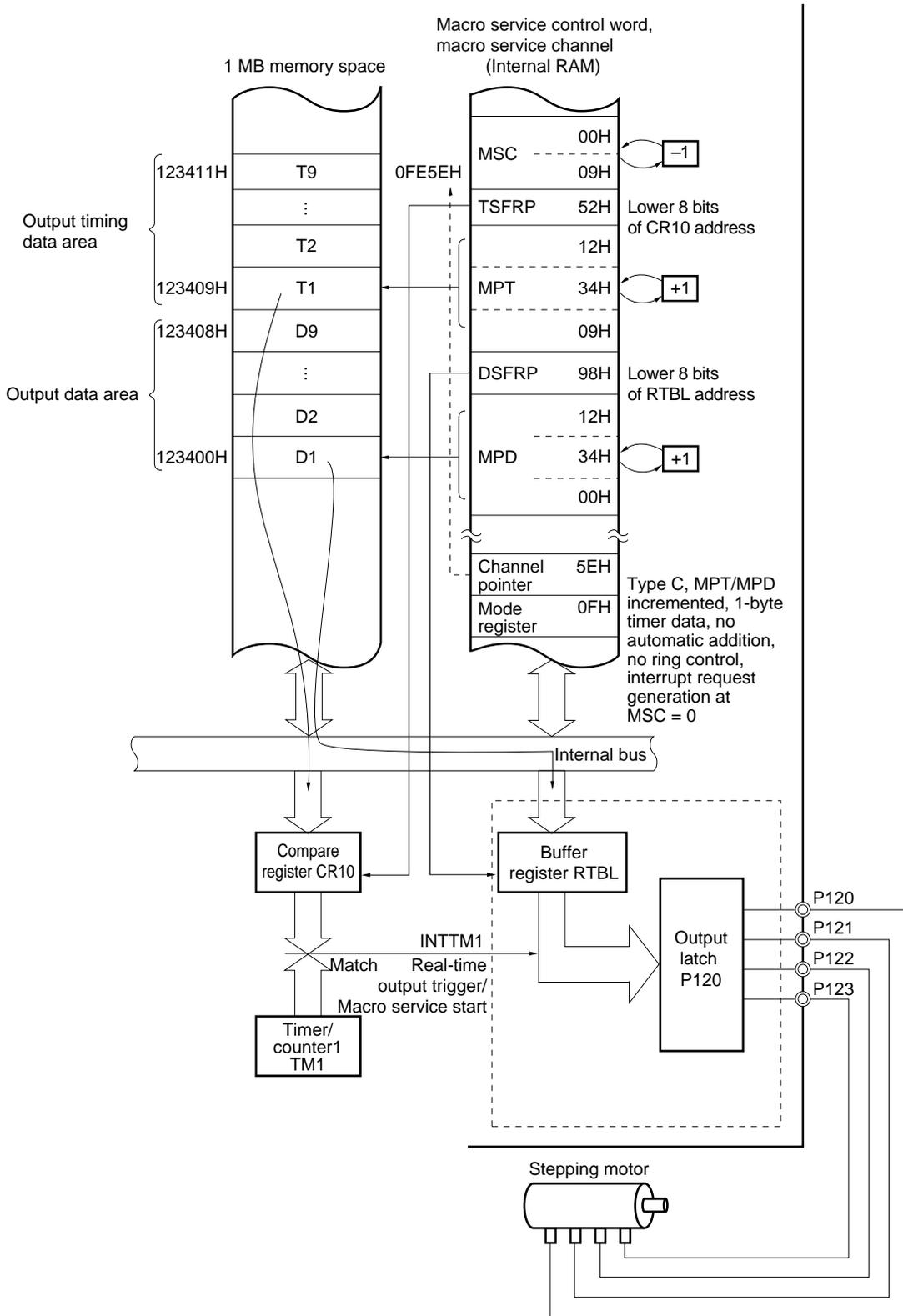
**Remark** Internal RAM addresses in the figure are the values when the LOCATION 0H instruction is executed. When the LOCATION 0FH instruction is executed, 0F0000H should be added to the values in the figure.
