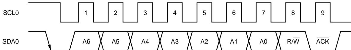
When receiving the base address, the automatic output of the acknowledge is synchronized to the falling edge of the eighth clock of SCL0 regardless of the ACEK0 value. When receiving at an address other than the base address, the acknowledge signal is not output.
