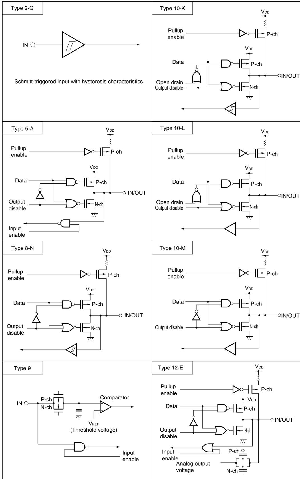
Figure 2-1. Pin I/O Circuit (2/2)
