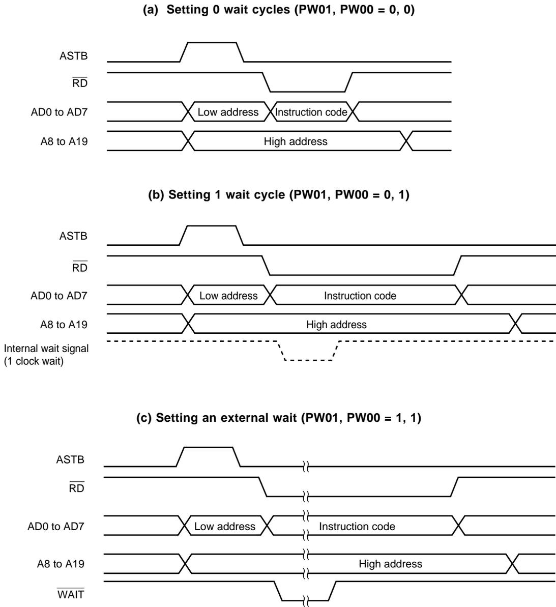
Figure 24-10. Read Timing for External Memory in Multiplexed Bus Mode
