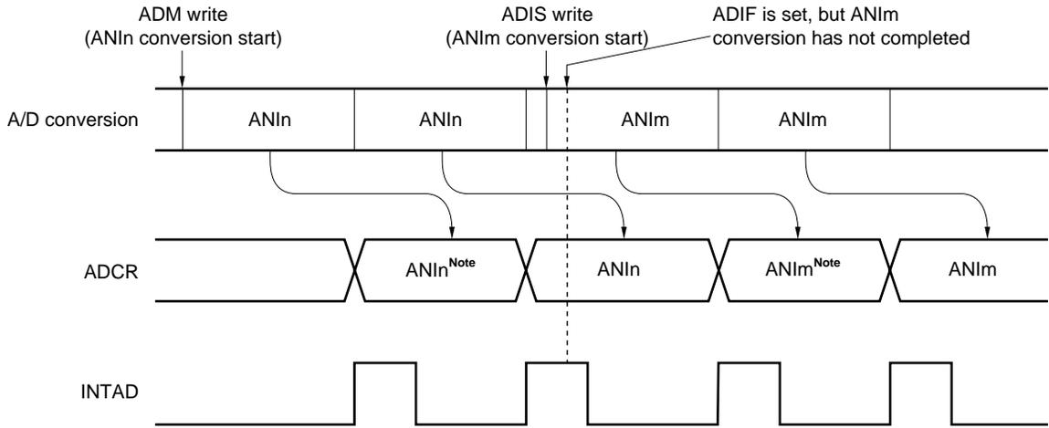
**Note** If bit 0 (ADCE) of the A/D converter mode register is not set to 1, the value of the first A/D conversion is undefined immediately after A/D conversion starts. Poll the A/D conversion end interrupt request (INTAD) and take measures such as discarding the first A/D conversion result.
