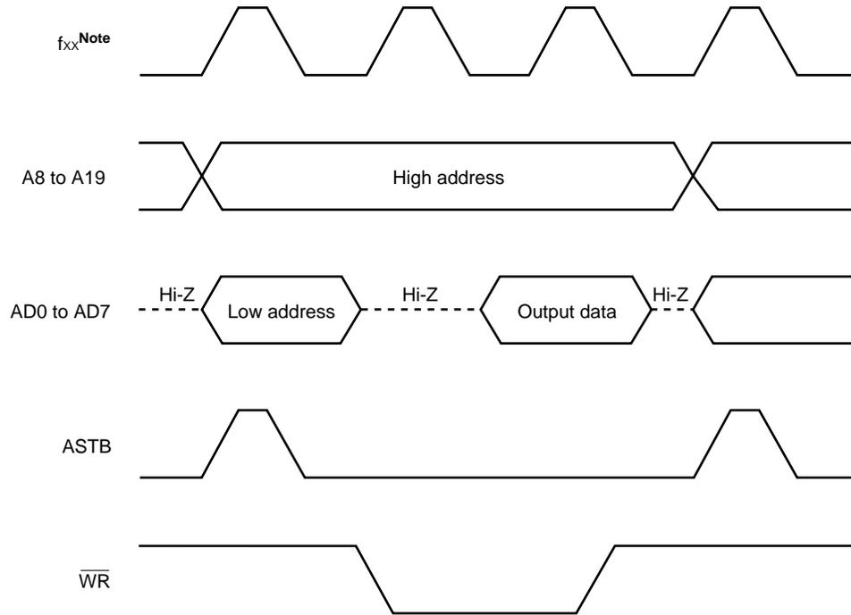
(d) Write timing when an address wait is inserted
