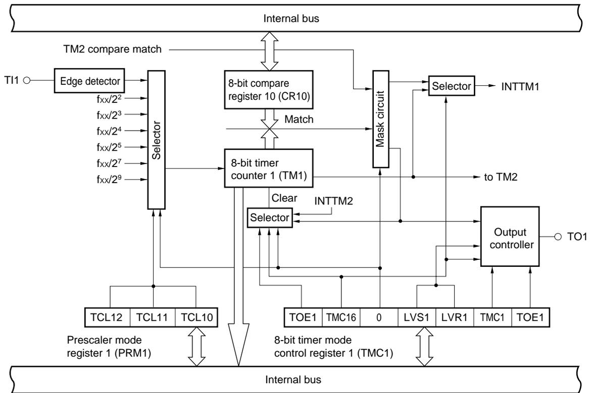
Figure 9-1. Block Diagram of 8-Bit Timer/Event Counter 1, 2 (2/2)
