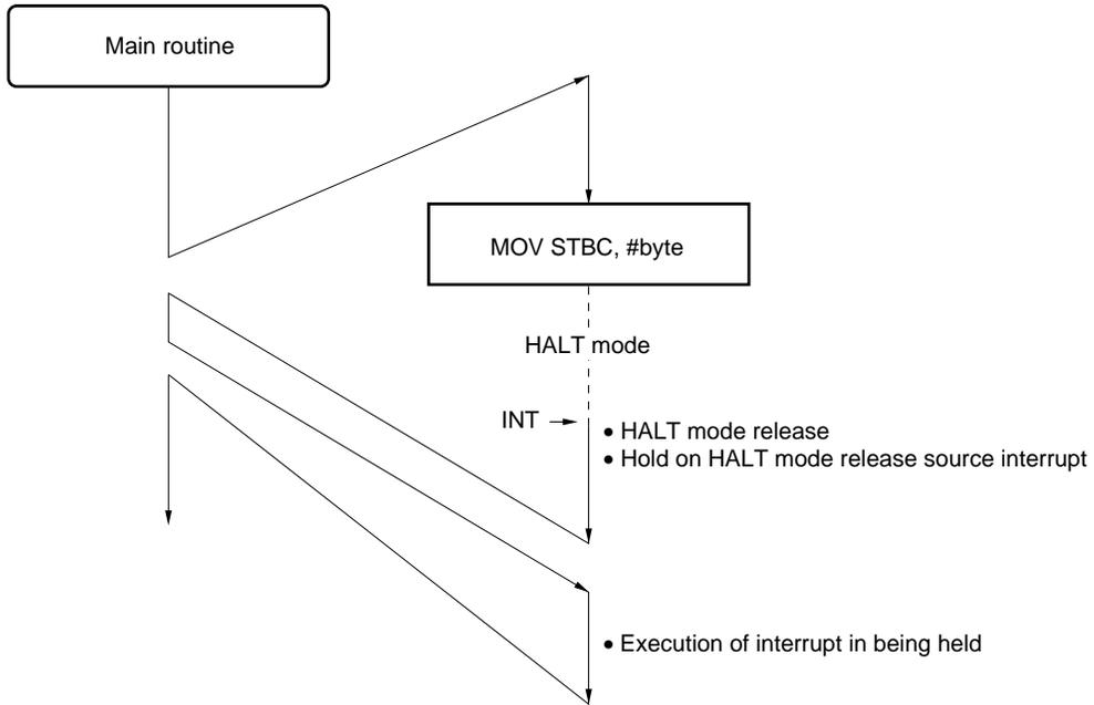
(4) HALT mode during interrupt processing routine whose priority is lower than release source interrupt
