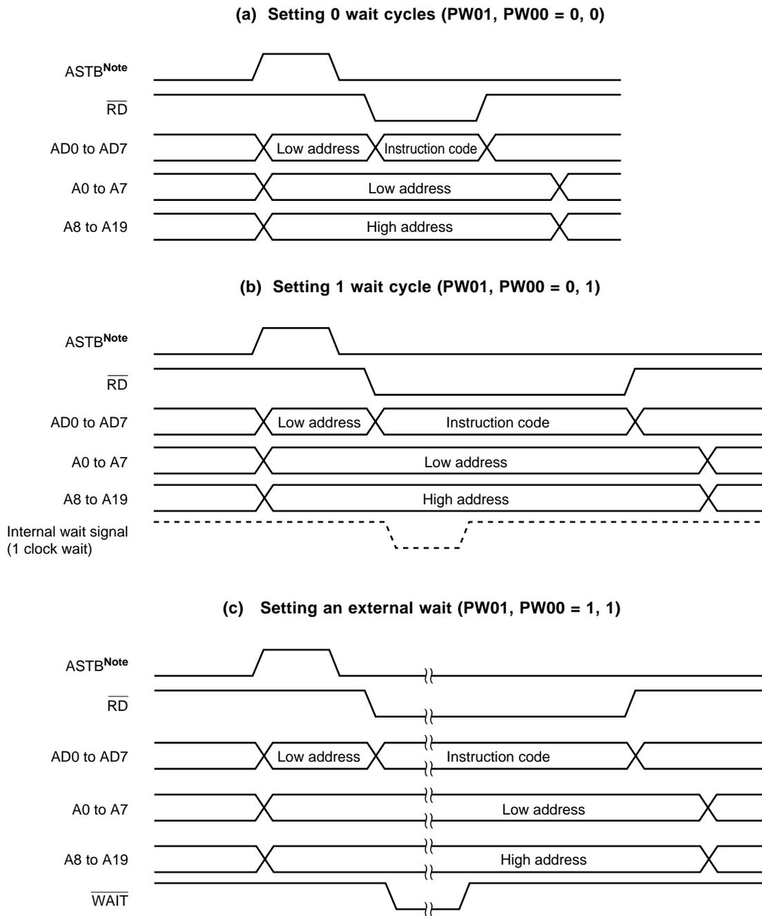
**Note** In the separate bus mode, the address strobe does not have to be used. However, the address strobe is output from the  $\overline{ASTB}/P67$  pin.
