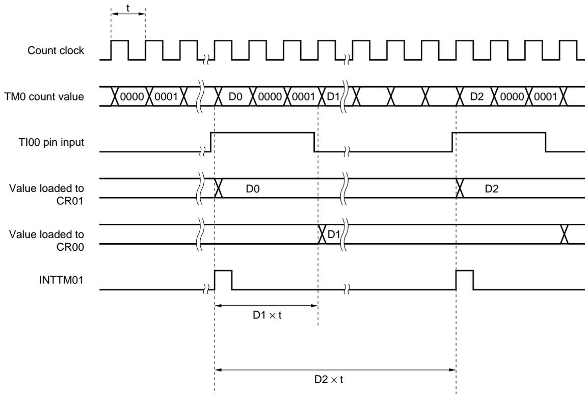
**Caution** For simplification purposes, delay due to noise elimination is not taken into consideration in the capture operation by TI00 pin input and in the interrupt request generation timing in the above figure. For a more accurate picture, refer to Figure 8-14 CR01 Capture Operation with Rising Edge Specified.
