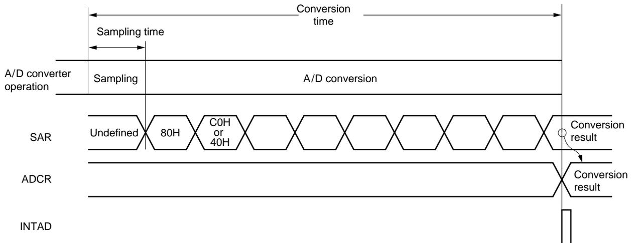
A/D conversion is performed continuously until ADM bit 7 (ADCS) is reset to 0 by software.
