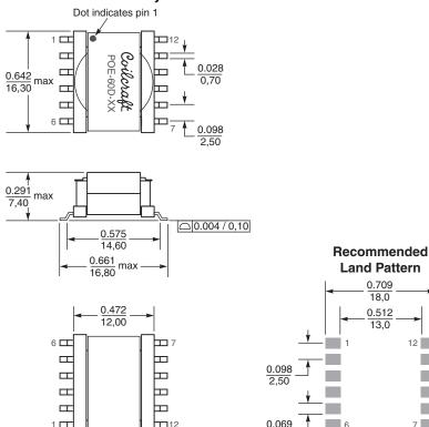
Dimensions are in  $\frac{\text{inches}}{\text{mm}}$
