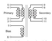
Primary windings and secondary windings to be connected in parallel on PC board.
