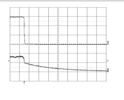
Turn-off at  $I_O$ =16 A resistive load at  $T_{ref}$ =+25 °C, Vin=3.3 V. Turn-off enabled by disconnecting  $V_{in}$ . Top trace: output voltage (0.5 V/div.). Bottom trace: input voltage (2 V/div.). Time scale: 2 ms/div.
