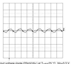
Output voltage ripple (20mV/div.) at  $\rm T_{ref}\!\!=\!\!+25~^{\circ}C,~Vin\!\!=\!\!3.3~V,~I_{0}\!\!=\!\!16~A$  resistive load. Band width=5MHz. Time scale: 2µs / div.
