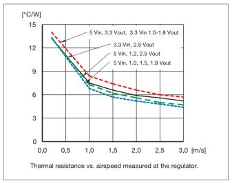
C. Max allowed calculated ambient temperature is: Max T<sub>ref</sub> of DC/DC regulator - temperature increase.
