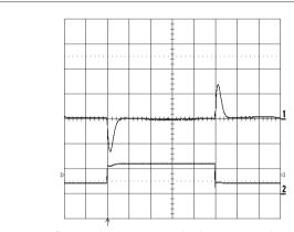
Output voltage response to load current step-change (4-12-4 A) at  $T_{ref}$  =+25 °C, Vin = 3.3 V. dl/dt = 5A/ $\mu s$  Top trace: output voltage (ac) (100 mV/div.). Bottom trace: load current (dc) (10 A/div.) Time scale: 0.1 ms/div.
