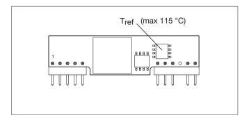
The PMB 4000 thermal testing is performed with the product mounted on an FR4 board 254  $\times$  254 mm with 8 layers of 35  $\mu$ m copper. Airflow is perpendicular to the  $T_{ref}$  side.
