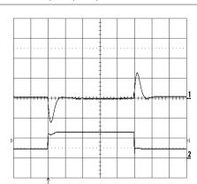
Output voltage response to load current step-change (4-12-4 A) at  $T_{ref}$  =+25 °C,  $V_{ref}$  = 3.3 V.  $V_{ref}$  div.) Top trace: output voltage (ac) (100 mV/div.). Bottom trace: load current (dc) (10 A/div.) Time scale: 0.1 ms/div.
