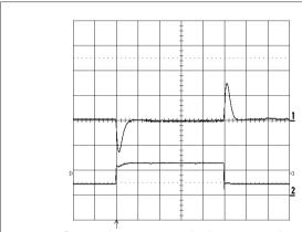
Output voltage response to load current step-change (4-12-4 A) at  $T_{ref}$  =+25 °C,  $V_{ref}$  = 3.3 V. dl/dt =  $5A/\mu s$  Top trace: output voltage (ac) (100 mV/div.). Bottom trace: load current (dc) (10 A/div.) Time scale: 0.1 ms/div.
