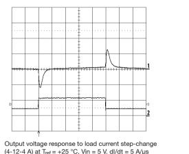
Output voltage response to load current step-change (4-12-4 A) at  $T_{ref}$  = +25 °C, Vin = 5 V. dl/dt = 5  $A/\mu s$  Top trace: output voltage (ac) (100 mV/div.). Bottom trace: load current (dc) (10 A/div.) Time scale: 0.1 ms/div.
