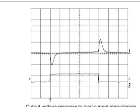
Output voltage response to load current step-change (4-12-4 A) at  $T_{ref}$  =+25 °C,  $V_{ref}$  =5 V.  $V_{ref}$  dl/dt = 5A/µs Top trace: output voltage (ac) (100 mV/div.). Bottom trace: load current (dc) (10 A/div.) Time scale: 0.1 ms/div.
