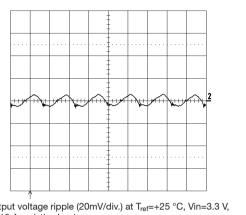
Output voltage ripple (20mV/div.) at  $T_{ref}$ =+25 °C,  $V_{ref}$ =3.3 V,  $I_{0}$ =16 A resistive load. Band width=5MHz. Time scale: 2 $\mu$ s / div.
