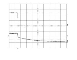
Turn-off at  $I_O$ =16 A resistive load at  $T_{ref}$ =+25 °C, Vin=3.3 V. Turn-off enabled by disconnecting  $V_{in}$ . Top trace: output voltage (0.5 V/div.). Bottom trace: input voltage (2 V/div.). Time scale: 2 ms/div.
