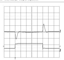
Output voltage response to load current step-change (4-12-4 A) at  $T_{ref}$  =+25 °C,  $V_{ref}$  Vin = 3.3 V.  $V_{ref}$  dI/dt =  $V_{ref}$ Top trace: output voltage (ac) (100 mV/div.). Bottom trace: load current (dc) (10 A/div.) Time scale: 0.1 ms/div.
