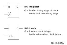
Figure 7. IOC Register Configurations
