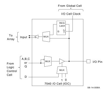
Figure 6. I/O Cell Block Diagram
