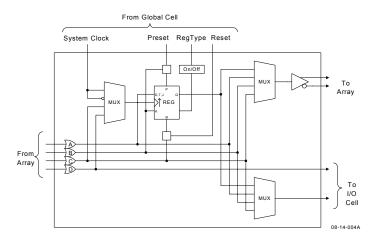
Figure 4. Logic Control Cell Block Diagram
