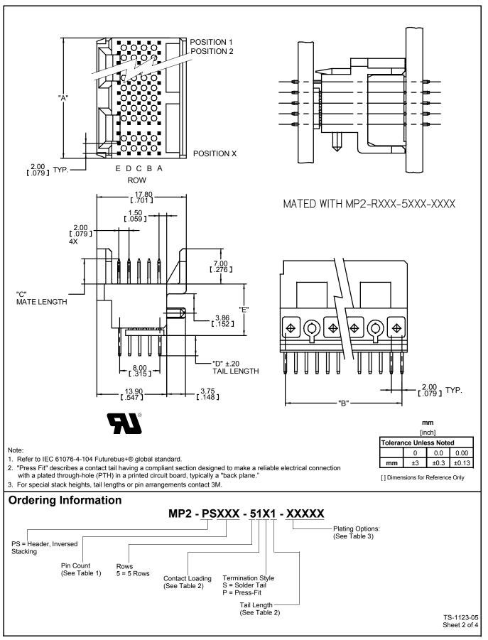
2 mm 5-Row, Stacking, Solder or Press-Fit Tail
