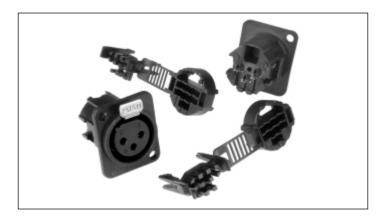
The Insulation Displacement Contact (IDC) connector is ideal for Original Equipment Manufacturers and end users alike and offers an alternative to our standard solder connector. Connectors can be can be quickly and easily assembled without screws or a soldering iron – by hand. Labour savings of up to 60% in termination time can be achieved.
