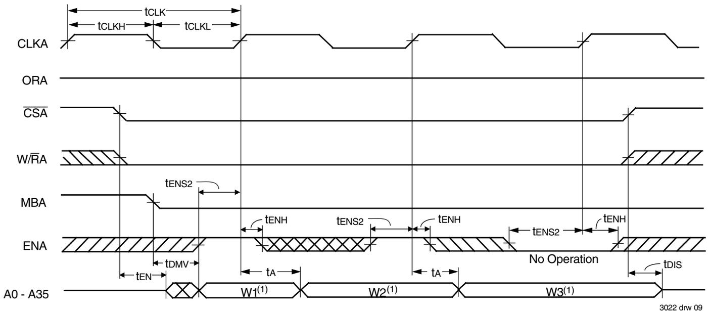
Figure 7. Port A Read Cycle Timing for FIFO2
