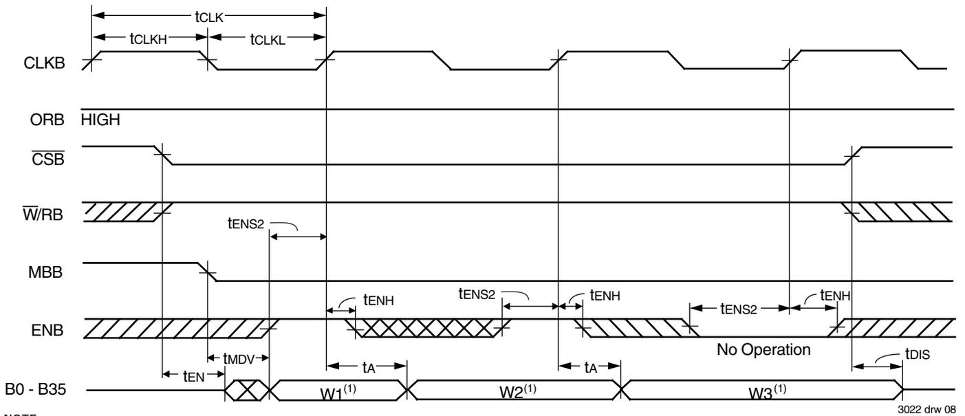
Figure 6. Port B Read Cycle Timing for FIFO1
