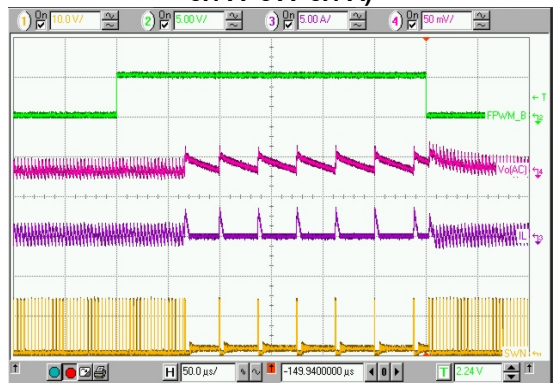
Top: FPWM#, FPWM# Signal, (5V/div) Middle 1: Vo2, CH2 Output Voltage Ripple, (50mV/div) Middle 2: iL2, CH2 Inductor Current, (5A/div) Bottom: SWN2, CH2 Switching Node Voltage, (10V/div) Time: 50µs/div
