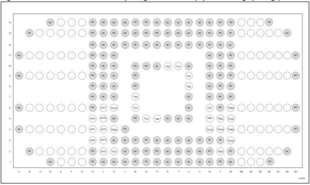
1. The ball corresponding to V<sub>CCI</sub> must be decoupled with an external capacitance.
