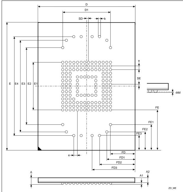
Figure 7. LFBGA169 14 x 18 x 1.4 mm 132+21+16 3R14 0.50 mm, package outline
