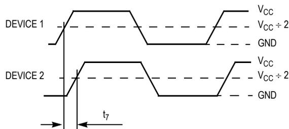
Figure 4. Device-to-Device Skew
