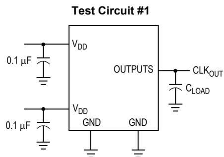
Test Circuit for all parameters
