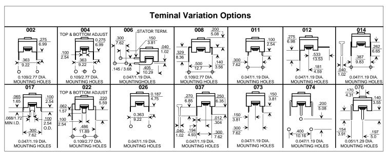
For dimensions  $\leq$  0.125"/3.18mm, tolerance is  $\pm$  0.015/0.38 For dimensions  $\geq$  0.126"/3.20mm, tolerance is  $\pm$  0.030/0.76 Specifications see page 2.
