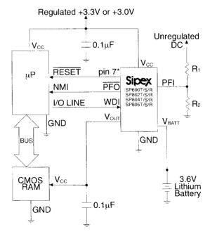
\*RESET for the SP690T/S/R and the SP802T/S/R RESET for the SP804T/S/R and the SP805T/S/R
