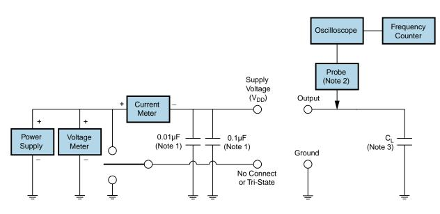
Note 1: An external 0.1µF low frequency tantalum bypass capacitor in parallel with a 0.01µF high frequency ceramic bypass capacitor close to the package ground and V<sub>DD</sub> pin is required.
