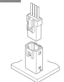
Applicable for waterproof usage. Its waterproof grade is more than 7 ingress protection of JIS C 0920 (IEC 60529 IPX7).
