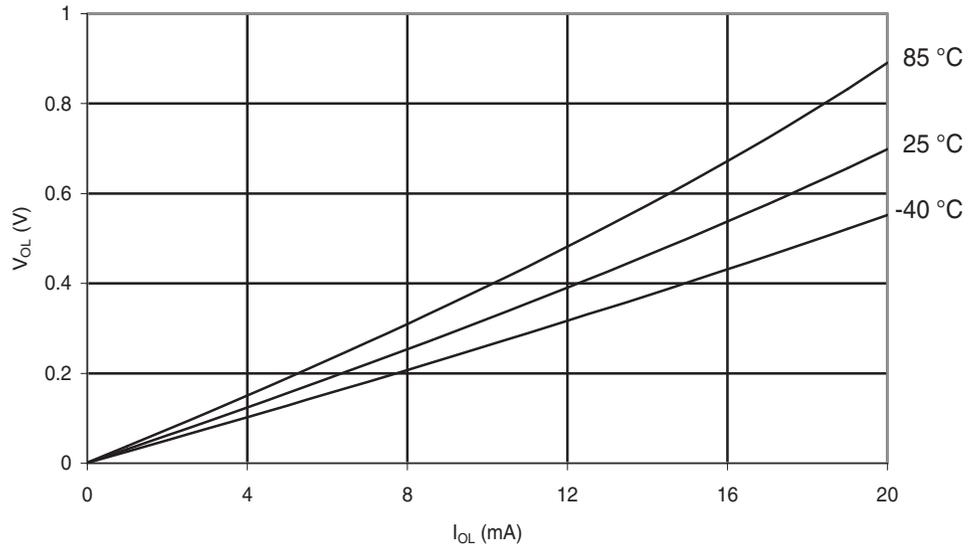
**Figure 6-157.** Atmel ATmega48PA: I/O Pin Output Voltage vs. Sink Current ( $V_{CC} = 5V$ )
