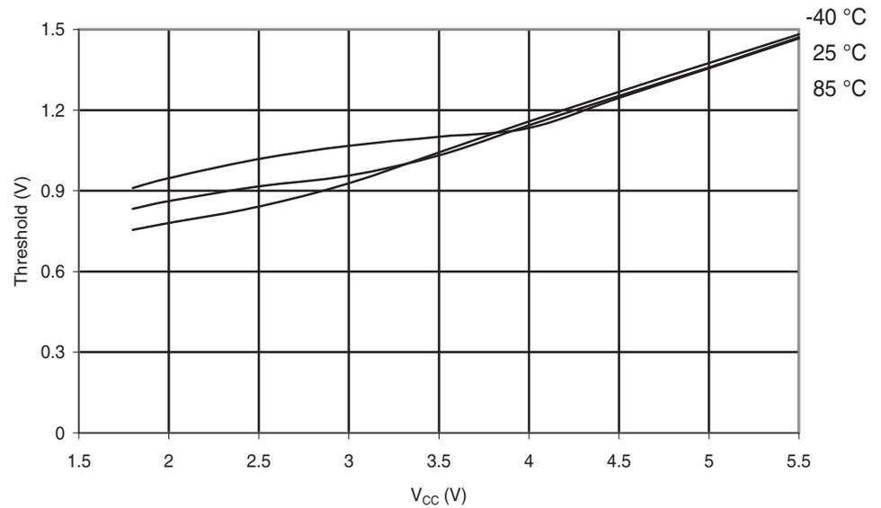
**Figure 6-210.** Atmel® ATmega88PA: Reset Input Threshold Voltage vs.  $V_{CC}$  ( $V_{IL}$ , I/O Pin read as '0')
