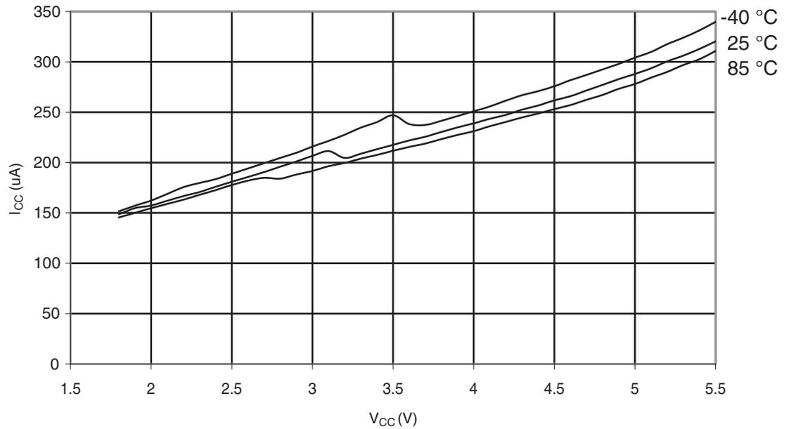
**Figure 6-313.** Atmel ATmega328P: Analog Comparator Current vs.  $V_{CC}$
