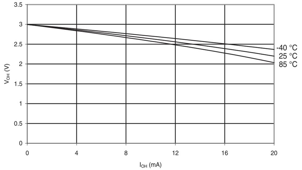
**Figure 6-205.** Atmel ATmega88PA: I/O Pin Output Voltage vs. Source Current ( $V_{CC} = 5V$ )
