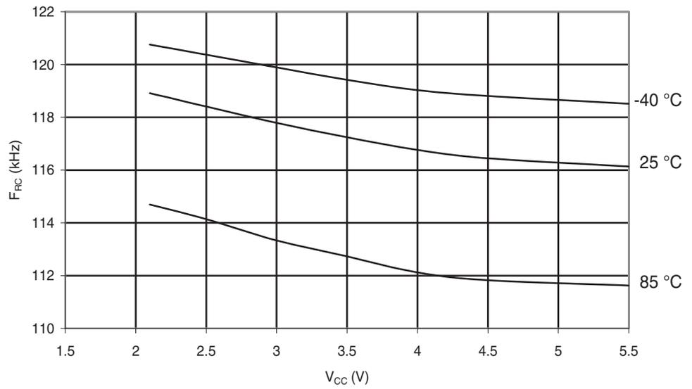
**Figure 6-263.** Atmel ATmega168PA: Calibrated 8MHz RC Oscillator Frequency vs.  $V_{CC}$
