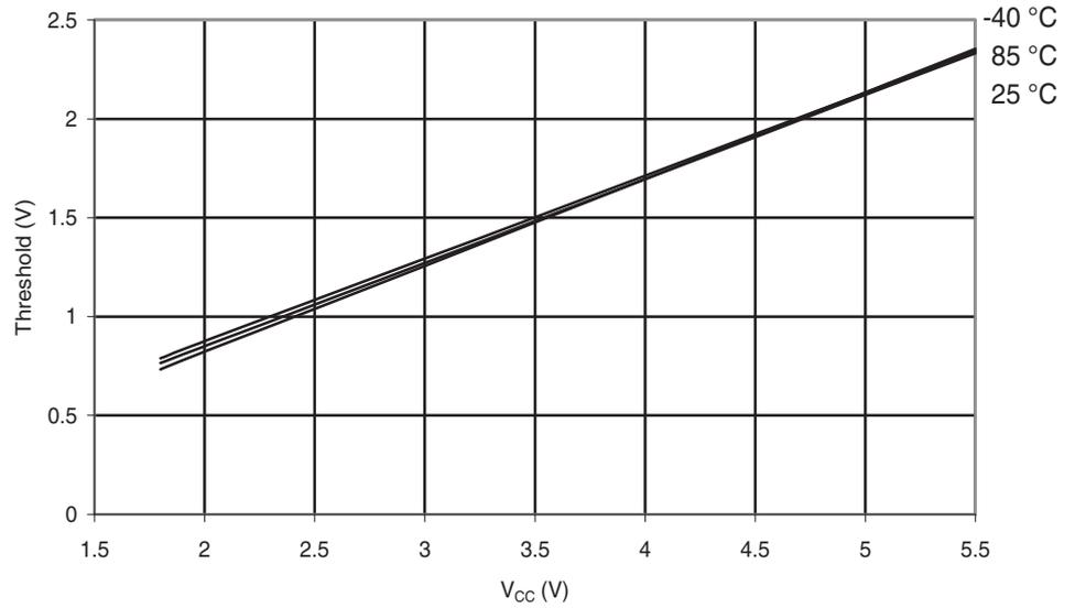
**Figure 6-257.** Atmel ATmega168PA: Reset Pin Input Hysteresis vs.  $V_{CC}$
