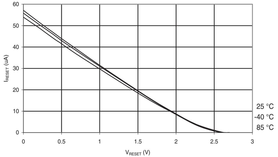
**Figure 6-201.** Atmel ATmega88PA: Reset Pull-up Resistor Current vs. Reset Pin Voltage ( $V_{CC} = 5V$ )
