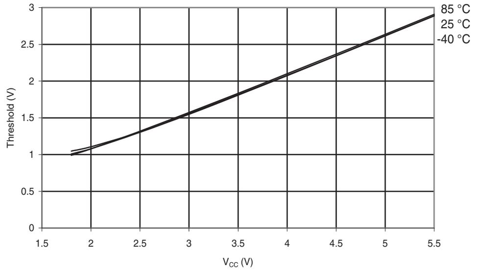
**Figure 6-253.** Atmel ATmega168PA: I/O Pin Input Threshold Voltage vs.  $V_{CC}$  ( $V_{IL}$ , I/O Pin read as '0')
