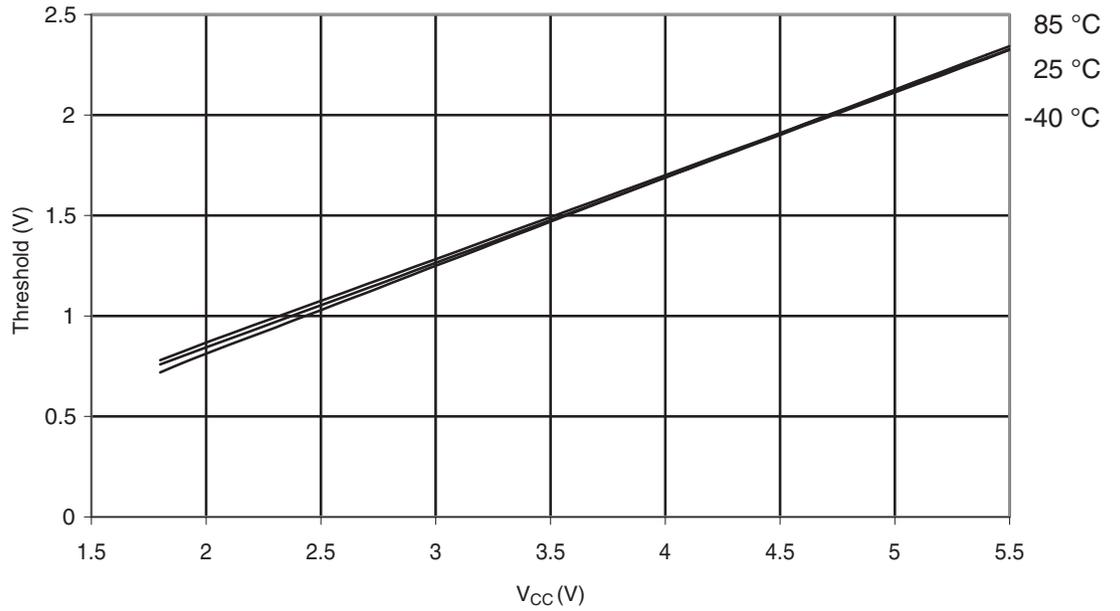
**Figure 6-303.** Atmel ATmega328P: Reset Pin Input Hysteresis vs.  $V_{CC}$
