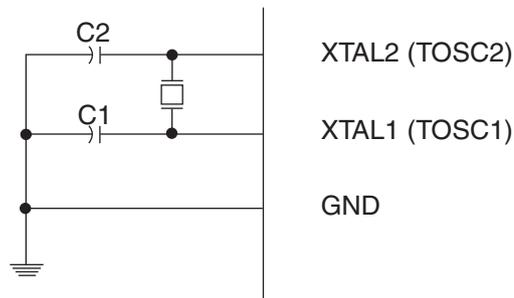
The Low Power Oscillator can operate in three different modes, each optimized for a specific frequency range. The operating mode is selected by the fuses CKSEL3..1 as shown in [Table 6-7 on page 55](#).
