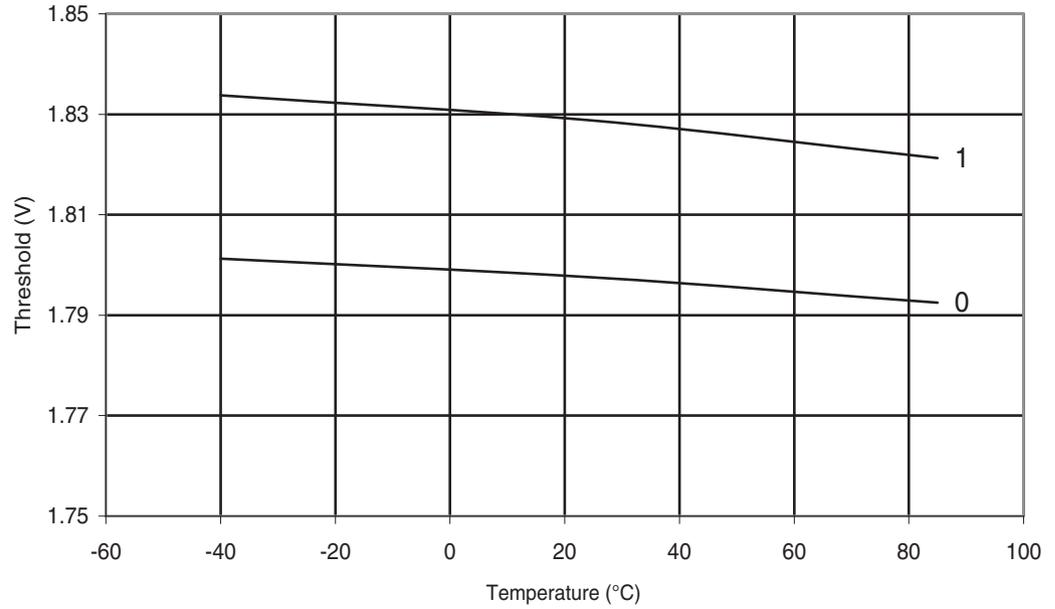
**Figure 6-305.** Atmel ATmega328P: BOD Thresholds vs. Temperature (BODLEVEL is 2.7V)
