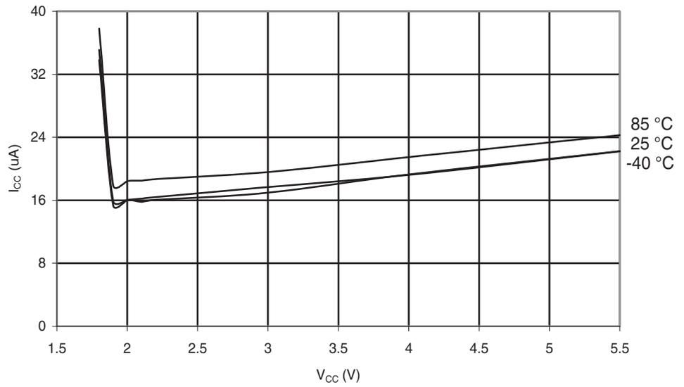
**Figure 6-178.** Atmel® ATmega48PA: Programming Current vs.  $V_{CC}$
