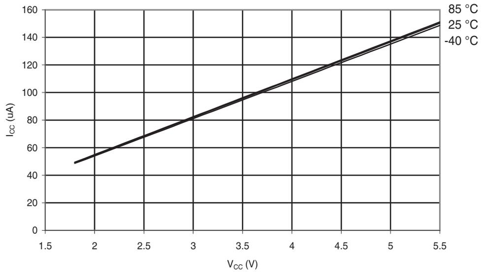
**Figure 6-223.** Atmel ATmega88PA: Brownout Detector Current vs.  $V_{CC}$
