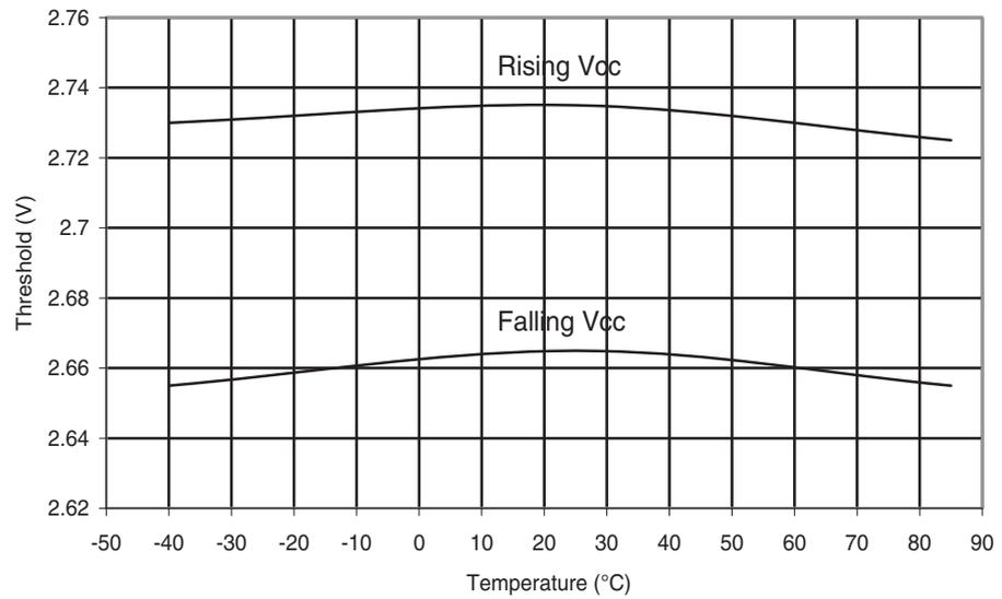
**Figure 6-260.** Atmel® ATmega168PA: BOD Thresholds vs. Temperature (BODLEVEL is 4.3V)
