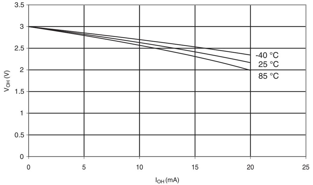
**Figure 6-297.** Atmel ATmega328P: I/O Pin Output Voltage vs. Source Current ( $V_{CC} = 5V$ )
