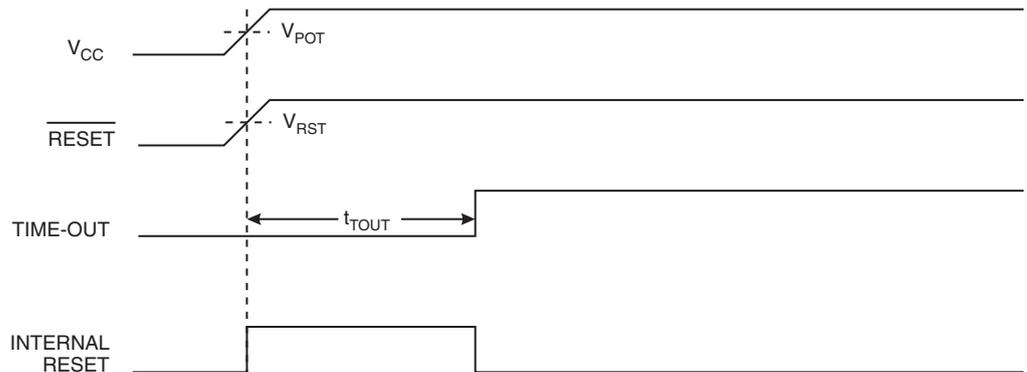
**Figure 6-17.** MCU Start-up,  $\overline{\text{RESET}}$  Extended Externally
