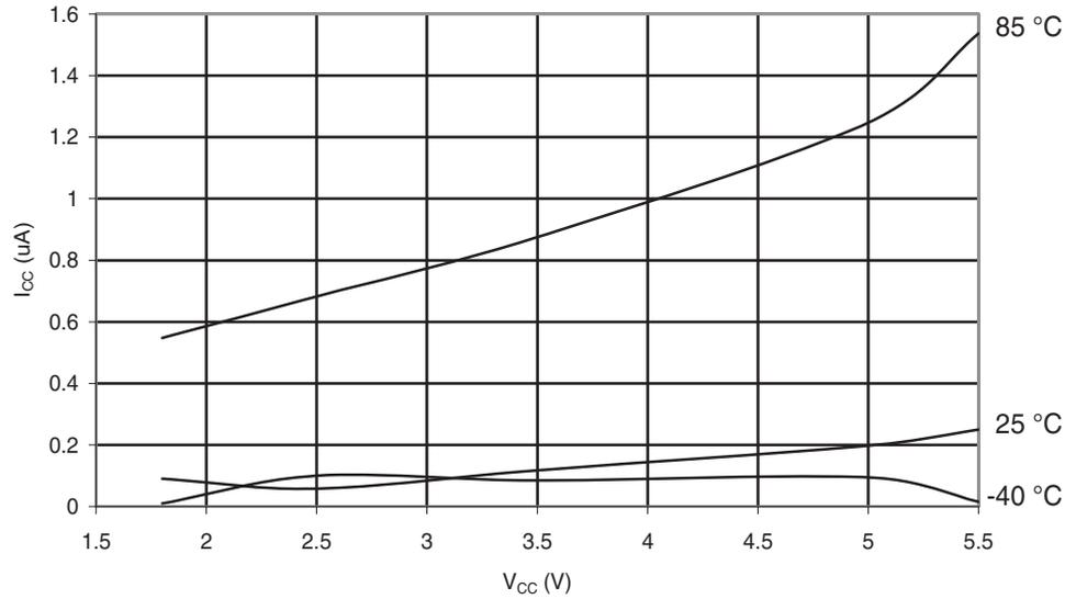
**Figure 6-193.** Atmel ATmega88PA: Power-Down Supply Current vs.  $V_{CC}$  (Watchdog Timer Enabled)
