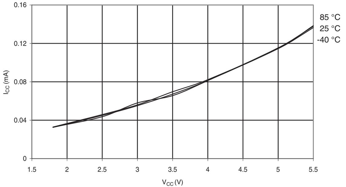
**Figure 6-277.** Atmel ATmega328P: Active Supply Current vs.  $V_{CC}$  (Internal RC Oscillator, 1MHz)
