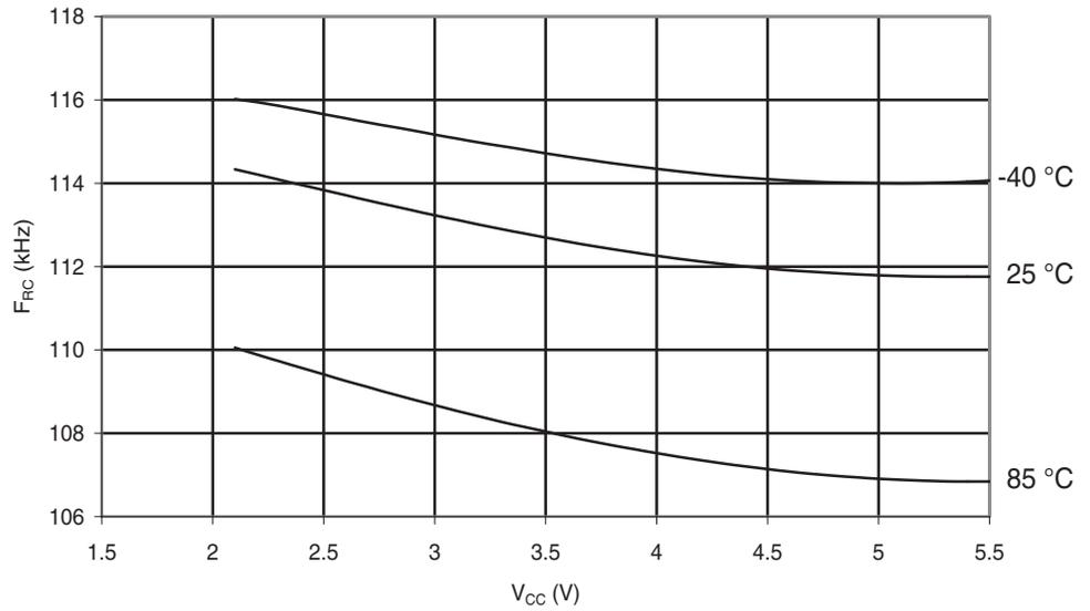
**Figure 6-171.** Atmel ATmega48PA: Calibrated 8 MHz RC Oscillator Frequency vs.  $V_{CC}$
