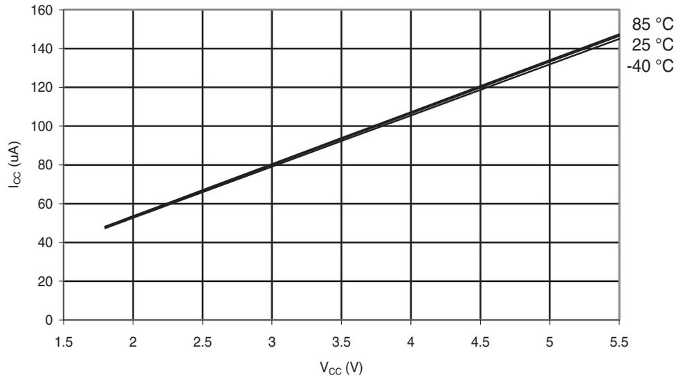
**Figure 6-177.** Atmel ATmega48PA: Brownout Detector Current vs.  $V_{CC}$
