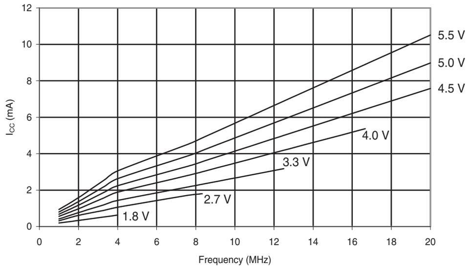
**Figure 6-138.** Atmel® ATmega48PA: Active Supply Current vs.  $V_{CC}$  (Internal RC Oscillator, 128kHz)
