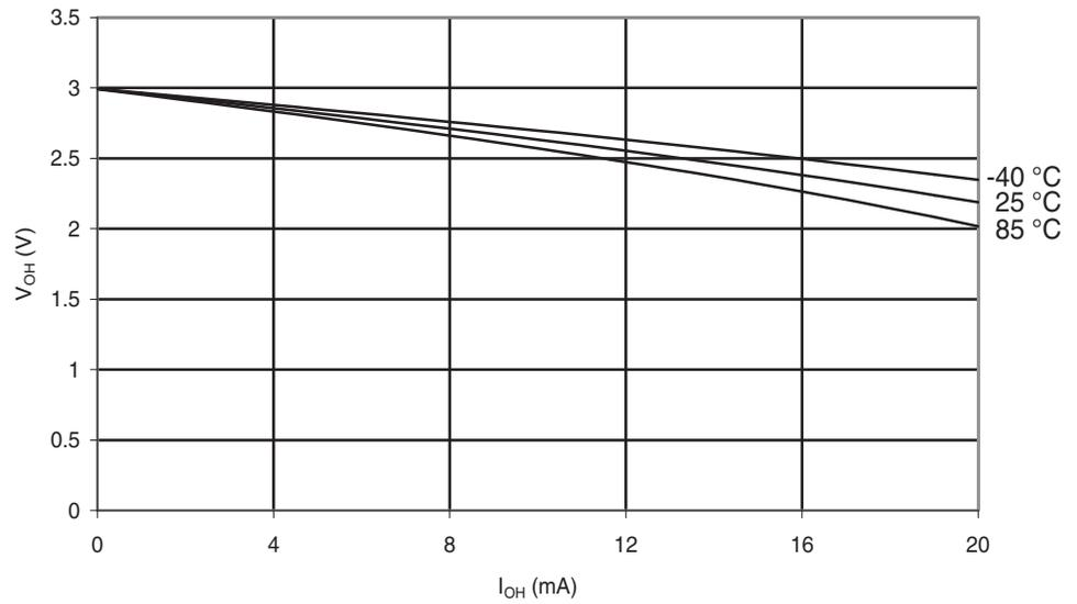
**Figure 6-251.** Atmel ATmega168PA: I/O Pin Output Voltage vs. Source Current ( $V_{CC} = 5V$ )
