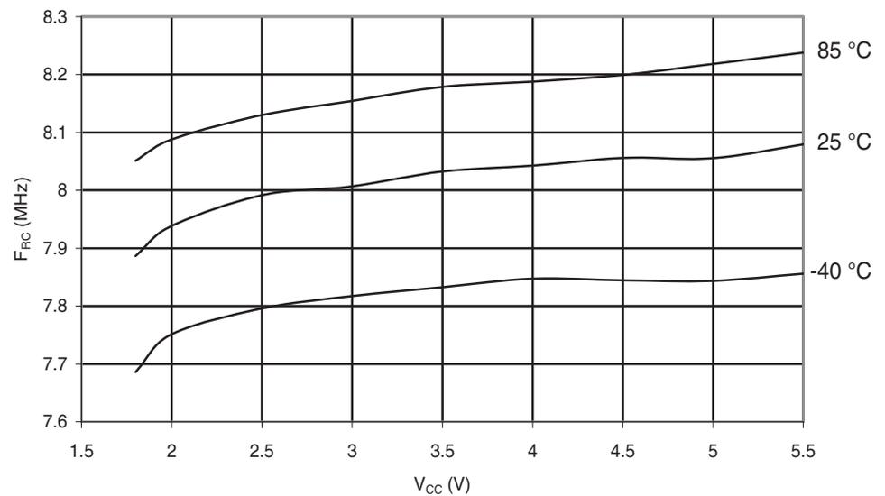
**Figure 6-218.** Atmel® ATmega88PA: Calibrated 8MHz RC Oscillator Frequency vs. Temperature
