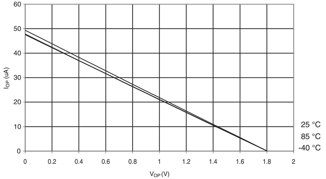
**Figure 6-289.** Atmel ATmega328P: I/O Pin Pull-up Resistor Current vs. Input Voltage ( $V_{CC} = 2.7V$ )
