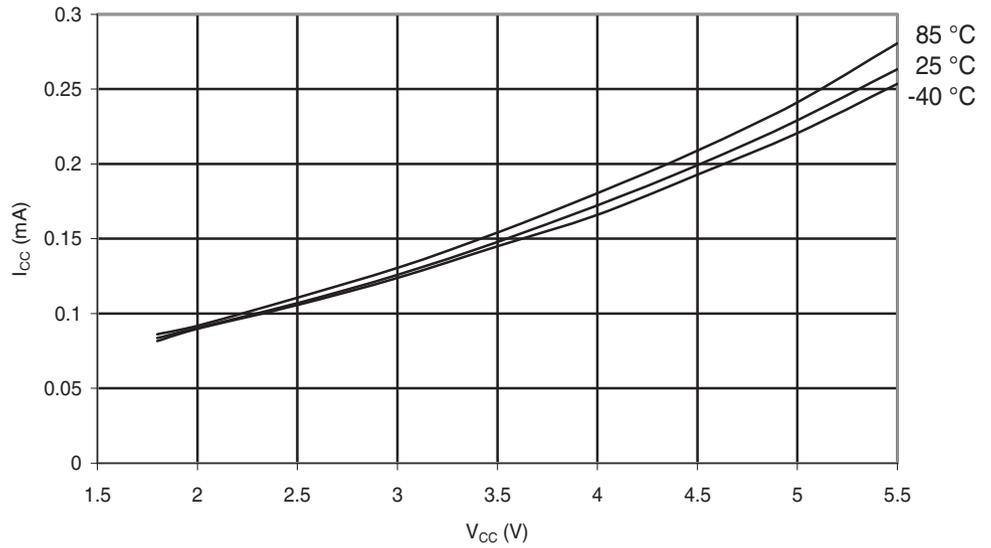
**Figure 6-237.** Atmel ATmega168PA: Idle Supply Current vs.  $V_{CC}$  (Internal RC Oscillator, 8MHz)
