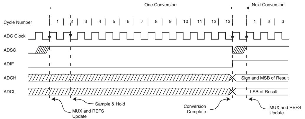
**Figure 6-106. ADC Timing Diagram, Auto Triggered Conversion**
