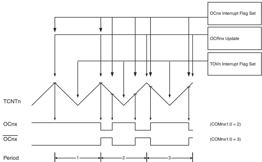
The Timer/Counter Overflow Flag (TOV2) is set each time the counter reaches BOTTOM. The Interrupt Flag can be used to generate an interrupt each time the counter reaches the BOTTOM value.
