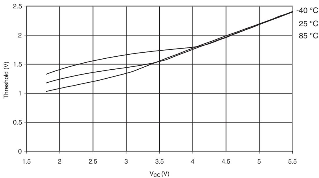
**Figure 6-302.** Atmel® ATmega328P: Reset Input Threshold Voltage vs.  $V_{CC}$  ( $V_{IL}$ , I/O Pin read as '0')
