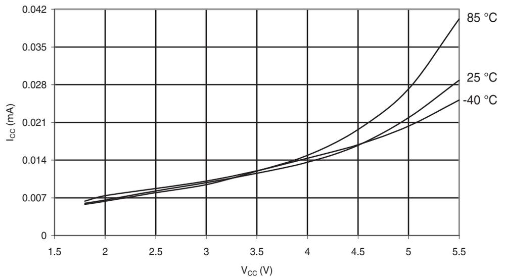
**Figure 6-144.** Atmel® ATmega48PA: Idle Supply Current vs.  $V_{CC}$  (Internal RC Oscillator, 1MHz)
