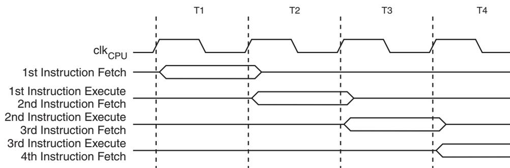
Figure 6-6 shows the internal timing concept for the Register File. In a single clock cycle an ALU operation using two register operands is executed, and the result is stored back to the destination register.
