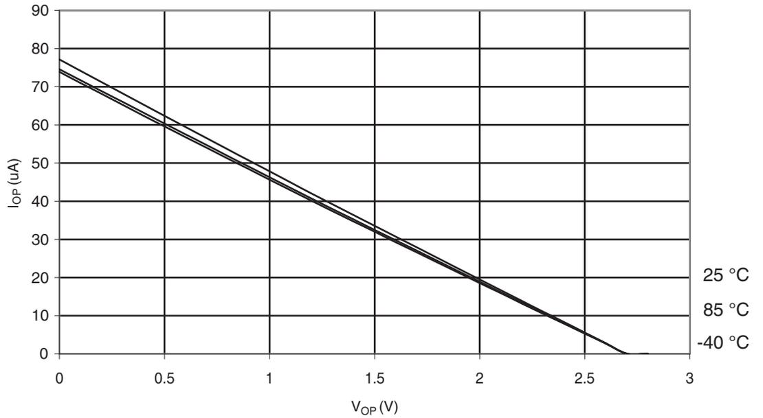
**Figure 6-290.** Atmel® ATmega328P: I/O Pin Pull-up Resistor Current vs. Input Voltage ( $V_{CC} = 5V$ )
