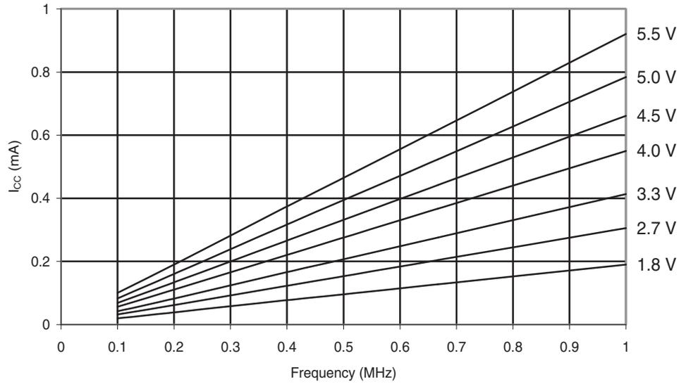
**Figure 6-229.** Atmel ATmega168PA: Active Supply Current vs. Frequency (1-20MHz)
