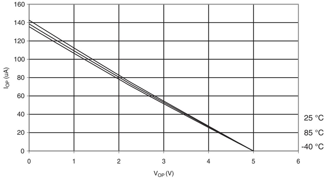
**Figure 6-291.** Atmel ATmega328P: Reset Pull-up Resistor Current vs. Reset Pin Voltage ( $V_{CC} = 1.8V$ )
