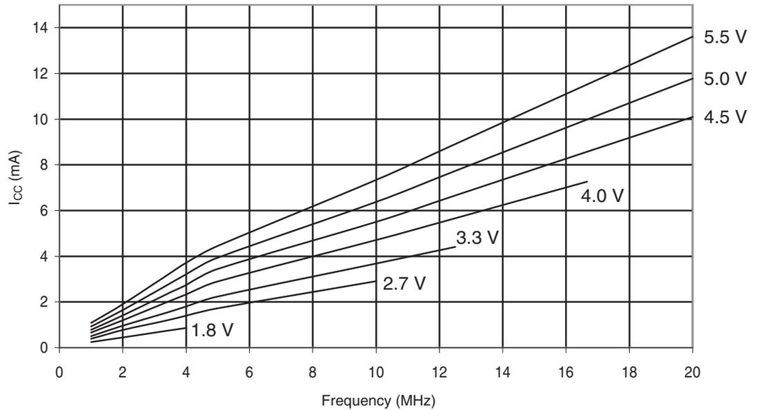
**Figure 6-276.** Atmel® ATmega328P: Active Supply Current vs.  $V_{CC}$  (Internal RC Oscillator, 128kHz)
