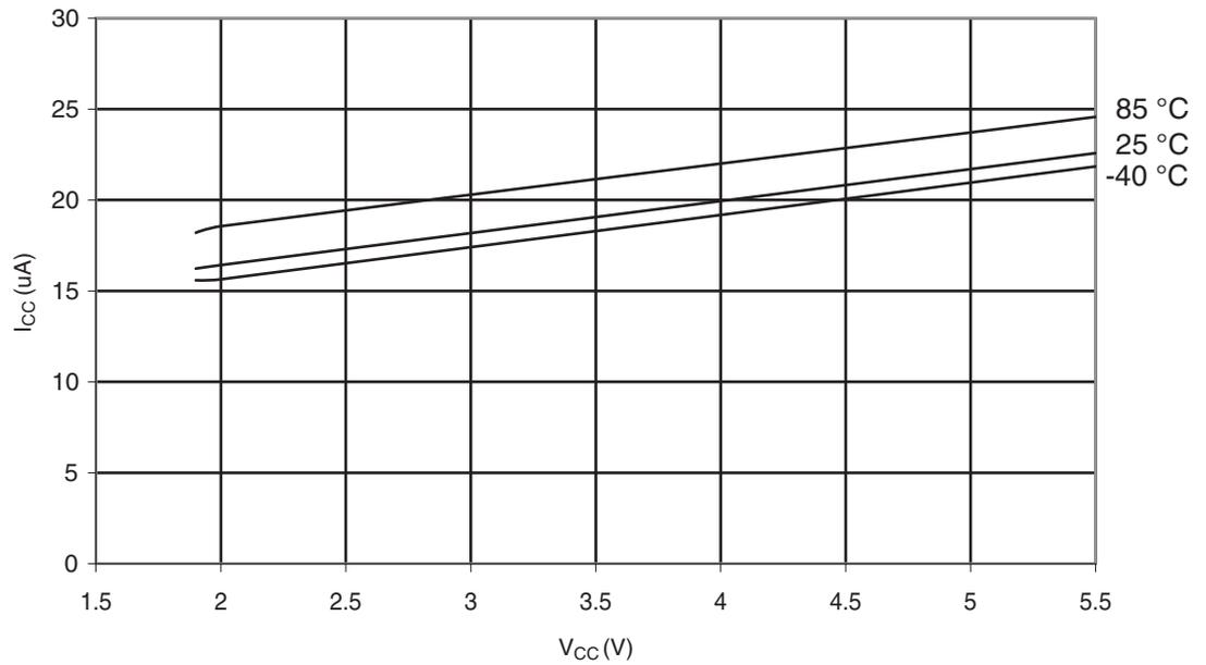
**Figure 6-316.** Atmel® ATmega328P: Programming Current vs.  $V_{CC}$
