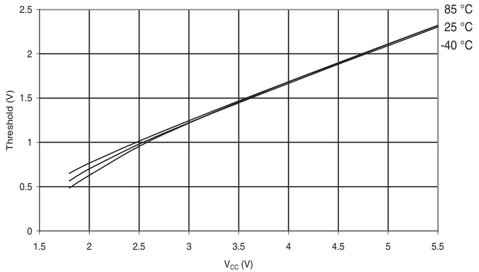
**Figure 6-254.** Atmel® ATmega168PA: I/O Pin Input Hysteresis vs.  $V_{CC}$
