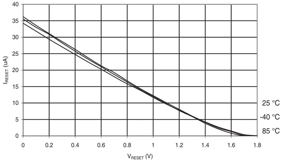
**Figure 6-200.** Atmel® ATmega88PA: Reset Pull-up Resistor Current vs. Reset Pin Voltage ( $V_{CC} = 2.7V$ )
