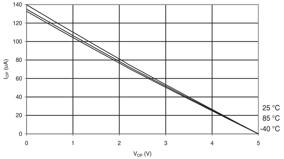
**Figure 6-199.** Atmel ATmega88PA: Reset Pull-up Resistor Current vs. Reset Pin Voltage ( $V_{CC} = 1.8V$ )
