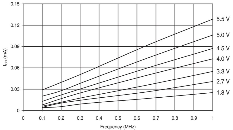
**Figure 6-188.** Atmel® ATmega88PA: Idle Supply Current vs. Frequency (1 - 20MHz)
