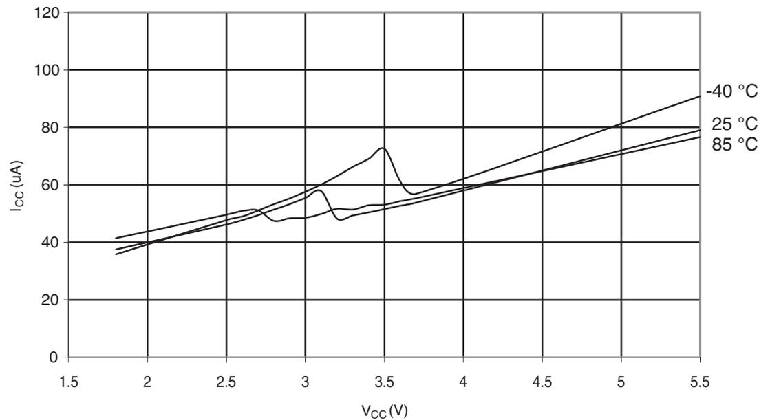
**Figure 6-314.** Atmel® ATmega328P: AREF External Reference Current vs.  $V_{CC}$
