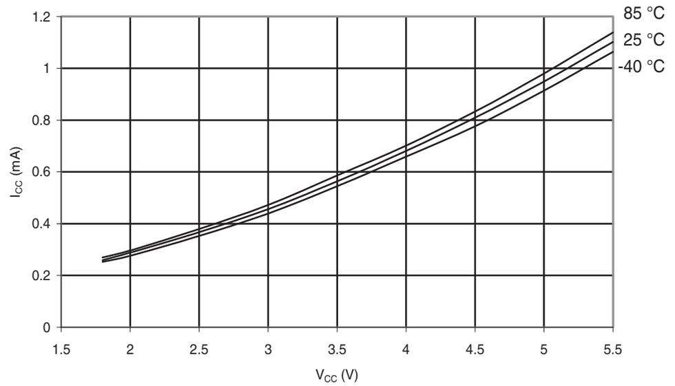
**Figure 6-186.** Atmel® ATmega88PA: Active Supply Current vs.  $V_{CC}$  (Internal RC Oscillator, 8MHz)
