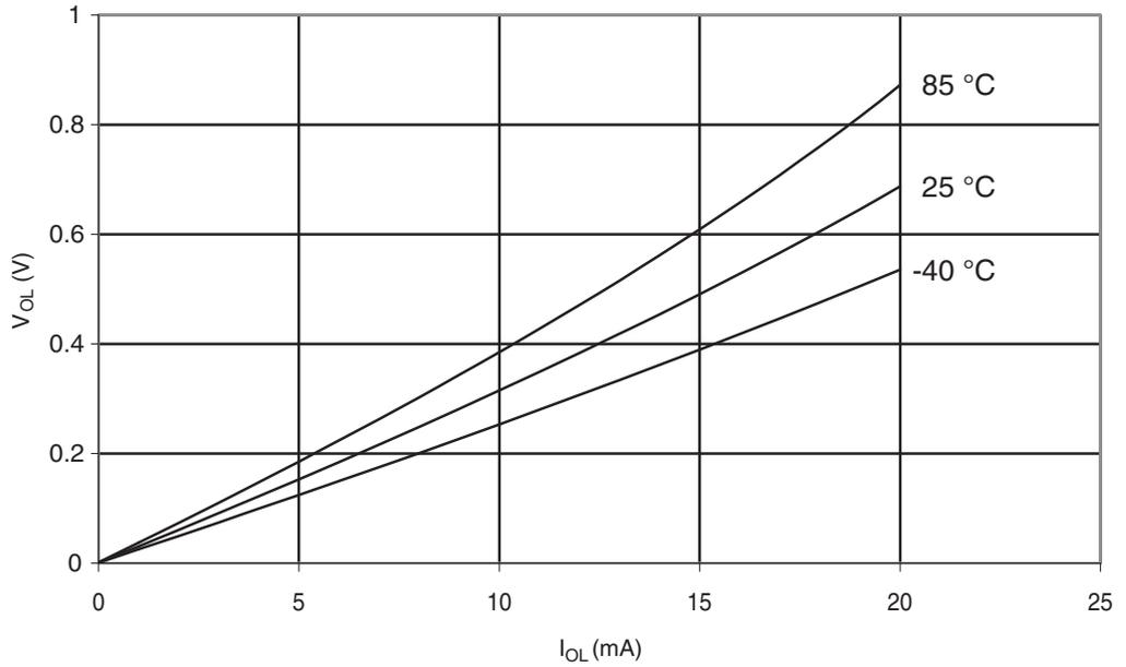
**Figure 6-295.** Atmel ATmega328P: I/O Pin Output Voltage vs. Sink Current ( $V_{CC} = 5V$ )
