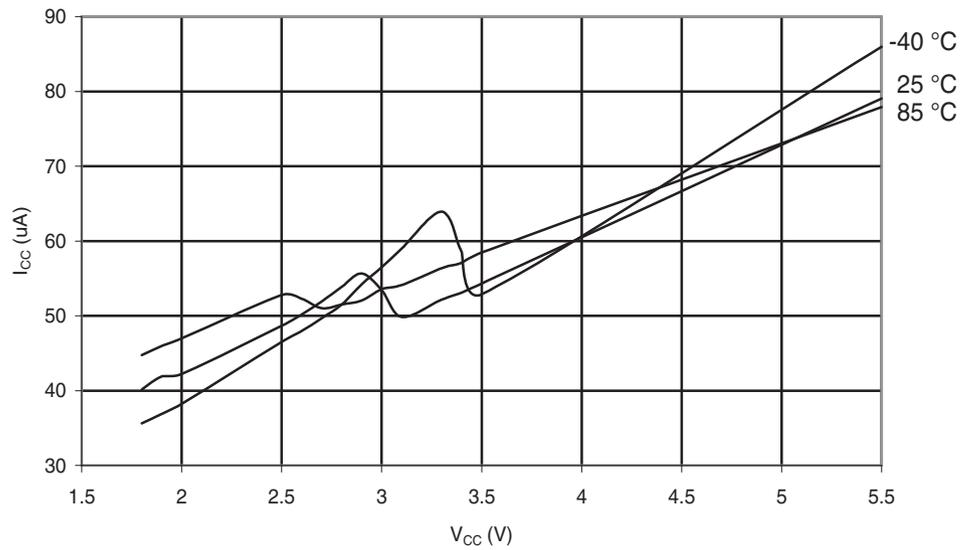
**Figure 6-268.** Atmel® ATmega168PA: AREF External Reference Current vs.  $V_{CC}$
