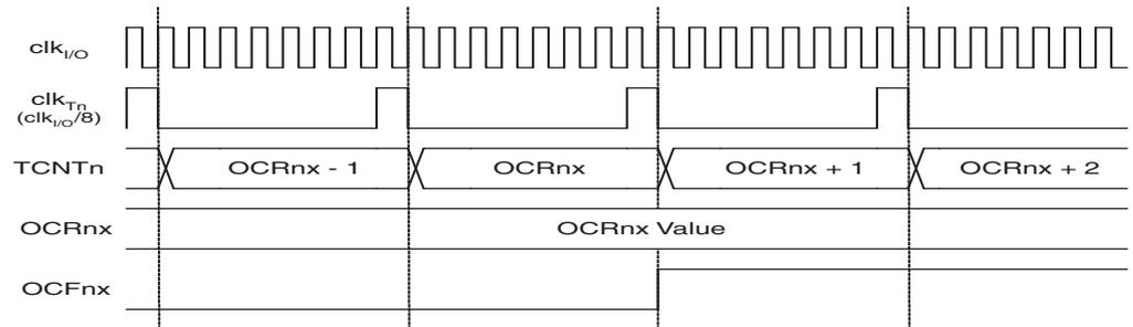
Figure 6-64 shows the setting of OCF2A and the clearing of TCNT2 in CTC mode.
