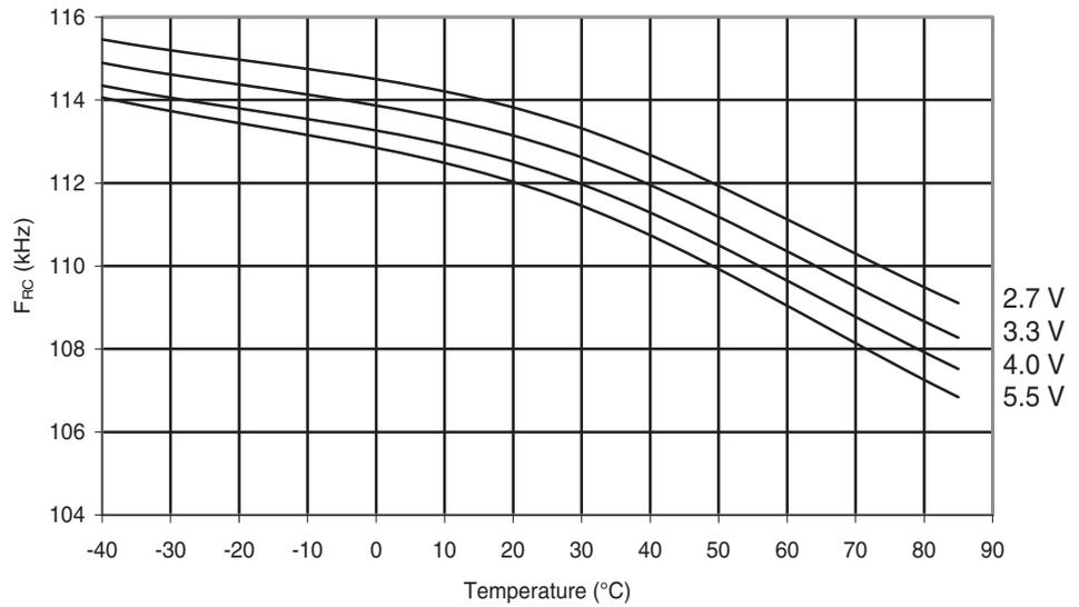
**Figure 6-170.** Atmel® ATmega48PA: Watchdog Oscillator Frequency vs.  $V_{CC}$
