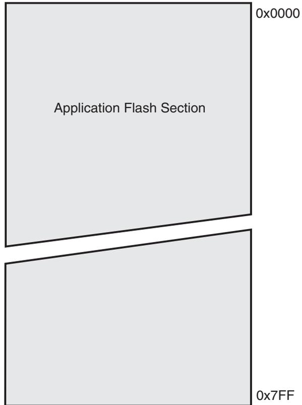
**Figure 6-8.** Program Memory Map Atmel ATmega88PA, ATmega168PA and ATmega328P
