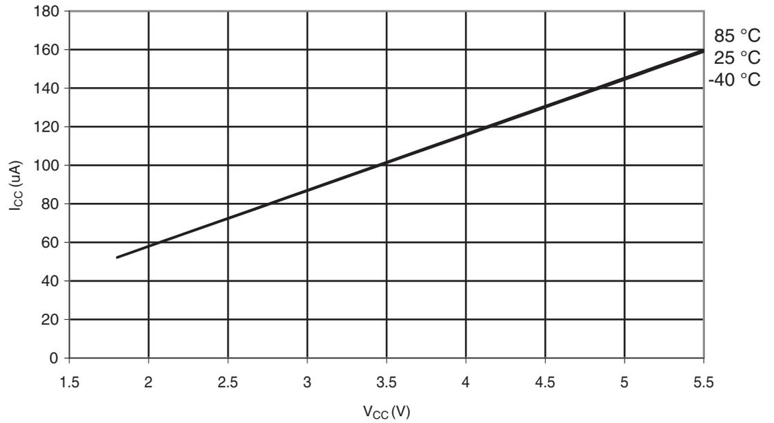
**Figure 6-315.** Atmel ATmega328P: Brownout Detector Current vs.  $V_{CC}$
