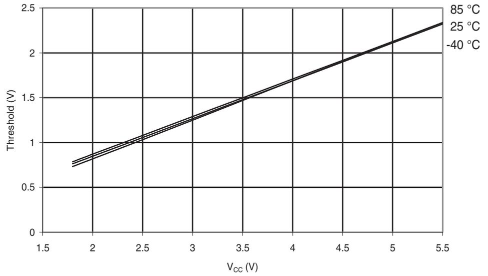
**Figure 6-211.** Atmel ATmega88PA: Reset Pin Input Hysteresis vs.  $V_{CC}$
