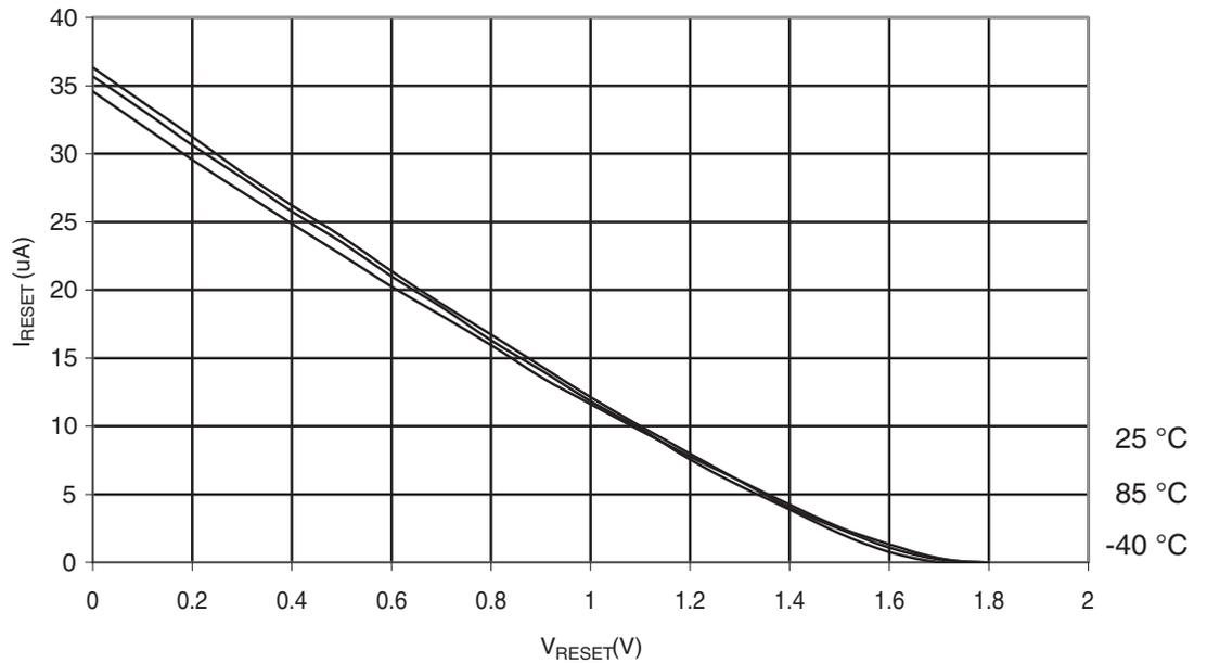
**Figure 6-292.** Atmel® ATmega328P: Reset Pull-up Resistor Current vs. Reset Pin Voltage ( $V_{CC} = 2.7V$ )
