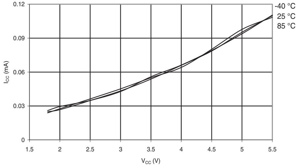
**Figure 6-185.** Atmel ATmega88PA: Active Supply Current vs.  $V_{CC}$  (Internal RC Oscillator, 1MHz)
