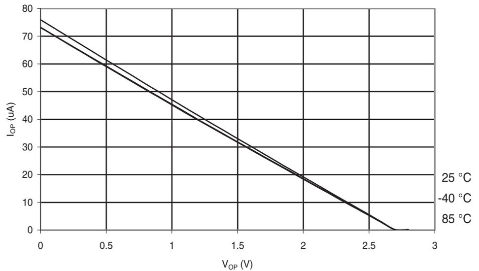
**Figure 6-244.** Atmel® ATmega168PA: I/O Pin Pull-up Resistor Current vs. Input Voltage ( $V_{CC} = 5V$ )
