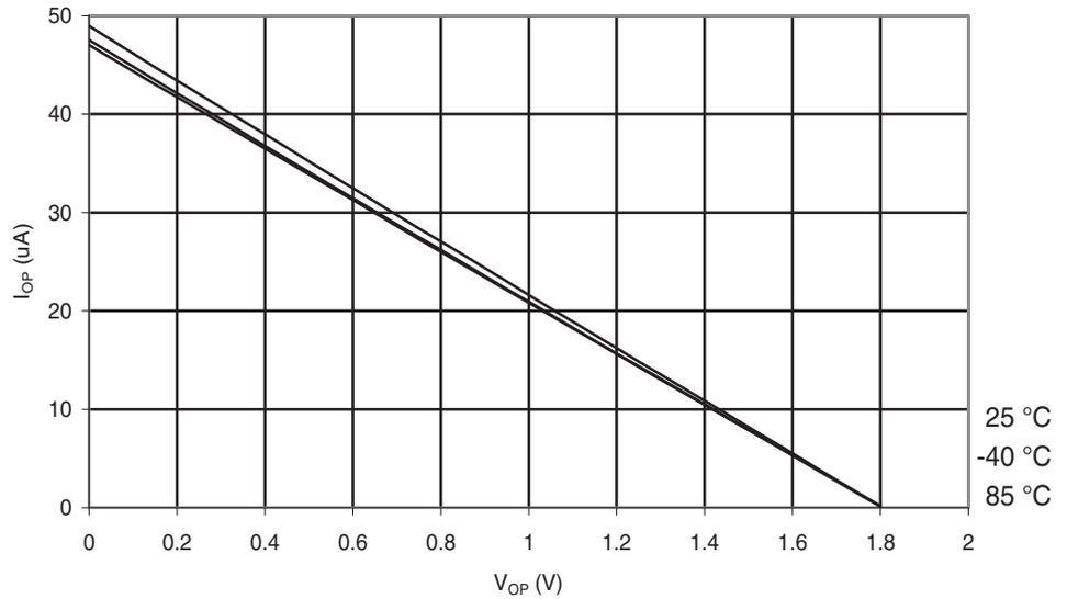
**Figure 6-243.** Atmel ATmega168PA: I/O Pin Pull-up Resistor Current vs. Input Voltage ( $V_{CC} = 2.7V$ )
