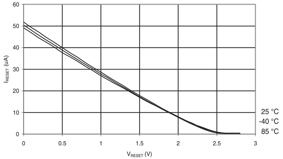
**Figure 6-155.** Atmel ATmega48PA: Reset Pull-up Resistor Current vs. Reset Pin Voltage ( $V_{CC} = 5V$ )
