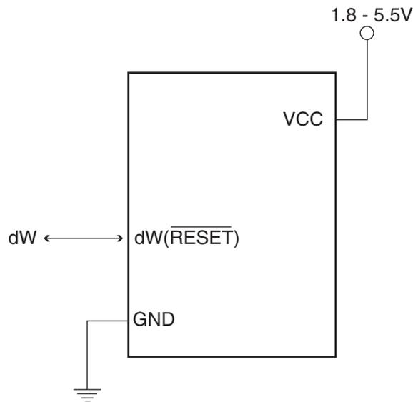
Figure 6-114 shows the schematic of a target MCU, with debugWIRE enabled, and the emulator connector. The system clock is not affected by debugWIRE and will always be the clock source selected by the CKSEL Fuses.
