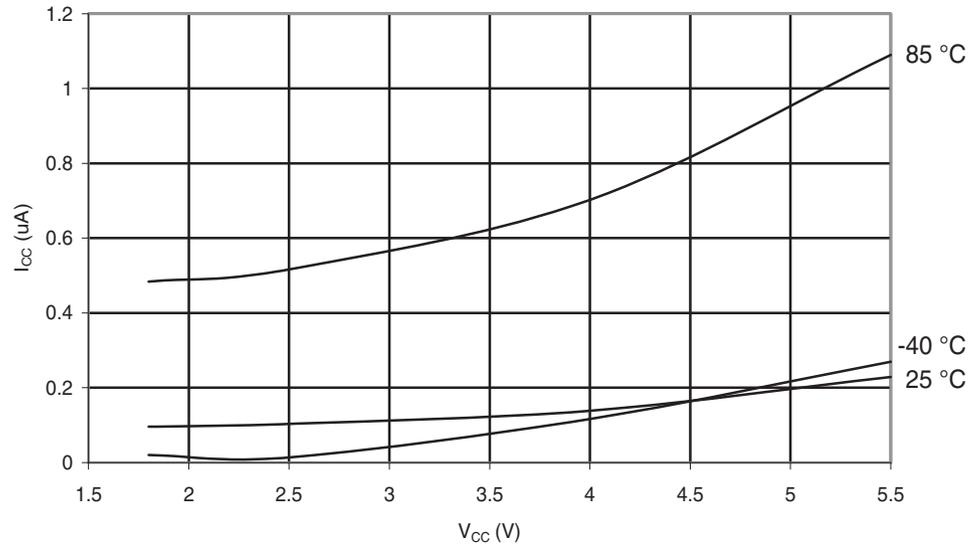
**Figure 6-147.** Atmel ATmega48PA: Power-Down Supply Current vs.  $V_{CC}$  (Watchdog Timer Enabled)
