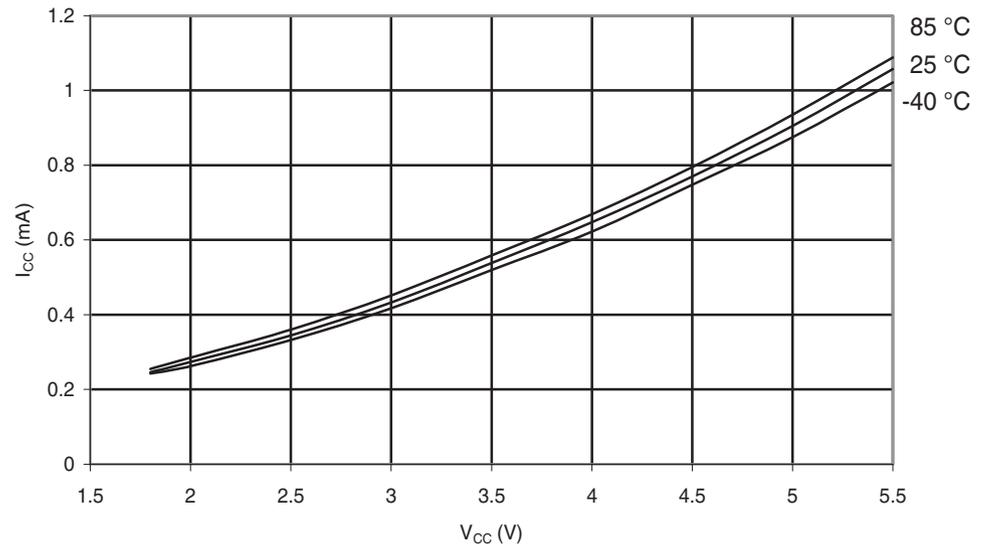
**Figure 6-232.** Atmel® ATmega168PA: Active Supply Current vs.  $V_{CC}$  (Internal RC Oscillator, 8MHz)
