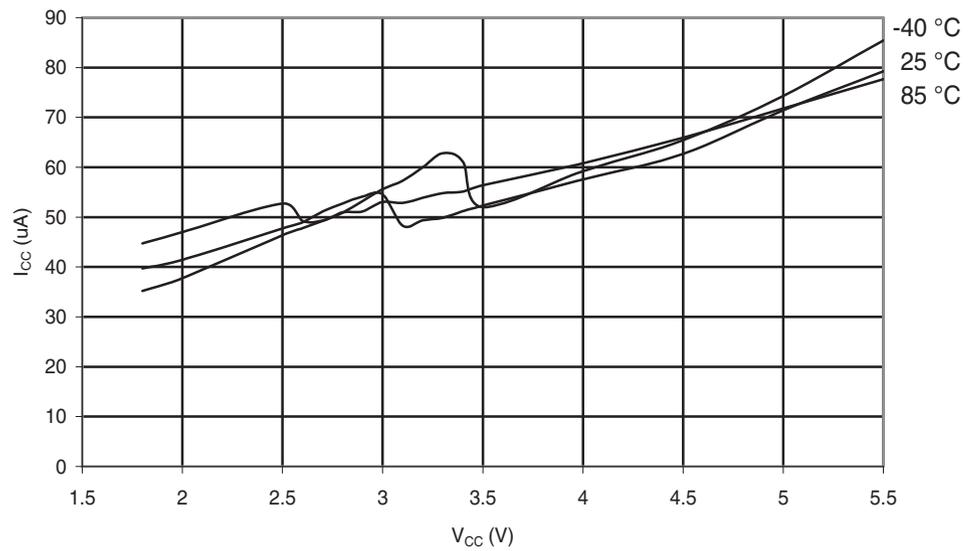
**Figure 6-222.** Atmel® ATmega88PA: AREF External Reference Current vs.  $V_{CC}$
