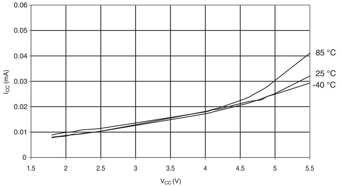
**Figure 6-282.** Atmel® ATmega328P: Idle Supply Current vs.  $V_{CC}$  (Internal RC Oscillator, 1MHz)
