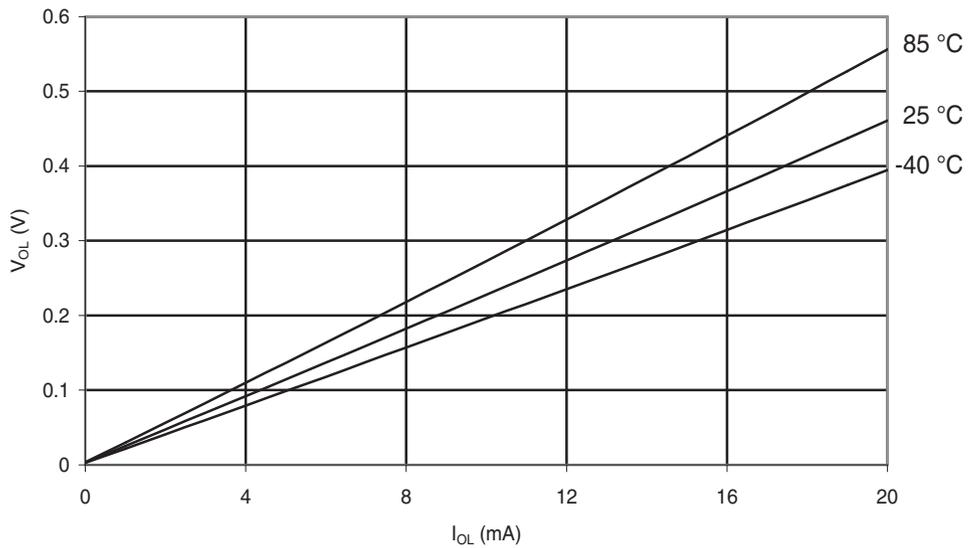
**Figure 6-250.** Atmel® ATmega168PA: I/O Pin Output Voltage vs. Source Current ( $V_{CC} = 3V$ )
