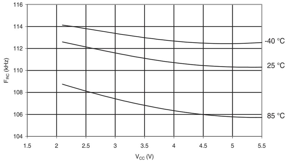
**Figure 6-217.** Atmel ATmega88PA: Calibrated 8 MHz RC Oscillator Frequency vs.  $V_{CC}$
