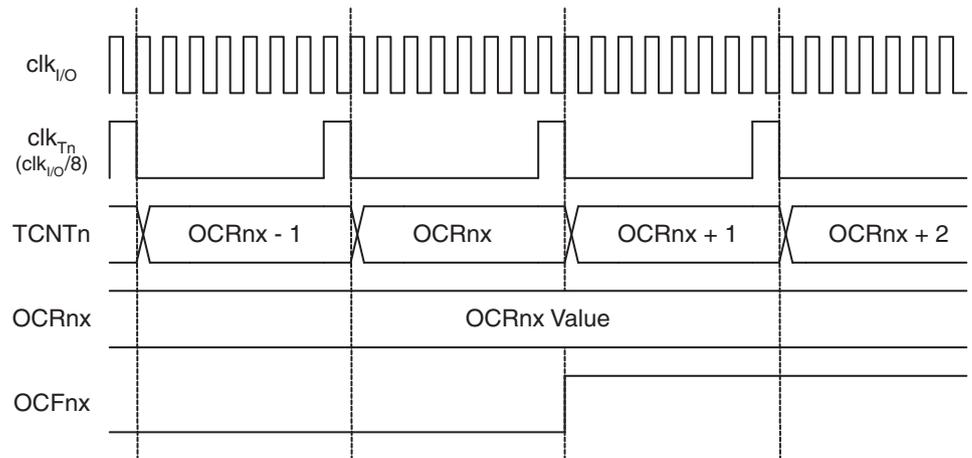
Figure 6-50 shows the count sequence close to TOP in various modes. When using phase and frequency correct PWM mode the  $OCR1x$  Register is updated at BOTTOM. The timing diagrams will be the same, but TOP should be replaced by BOTTOM, TOP-1 by BOTTOM+1 and so on. The same renaming applies for modes that set the TOV1 Flag at BOTTOM.
