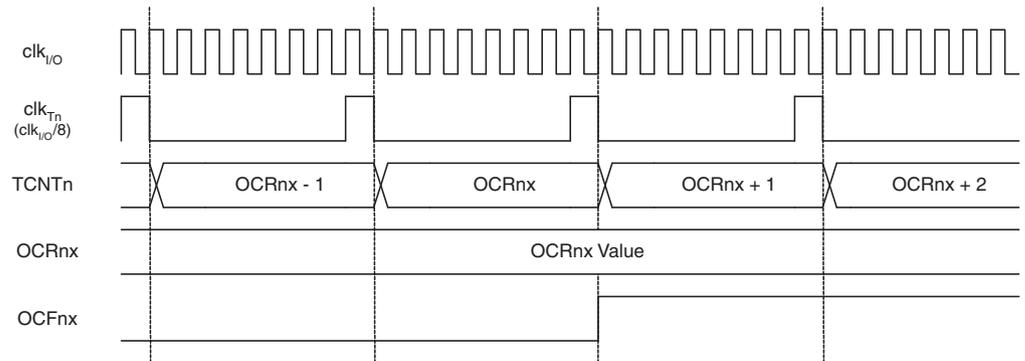
Figure 6-38 shows the setting of OCF0A and the clearing of TCNT0 in CTC mode and fast PWM mode where OCR0A is TOP.
