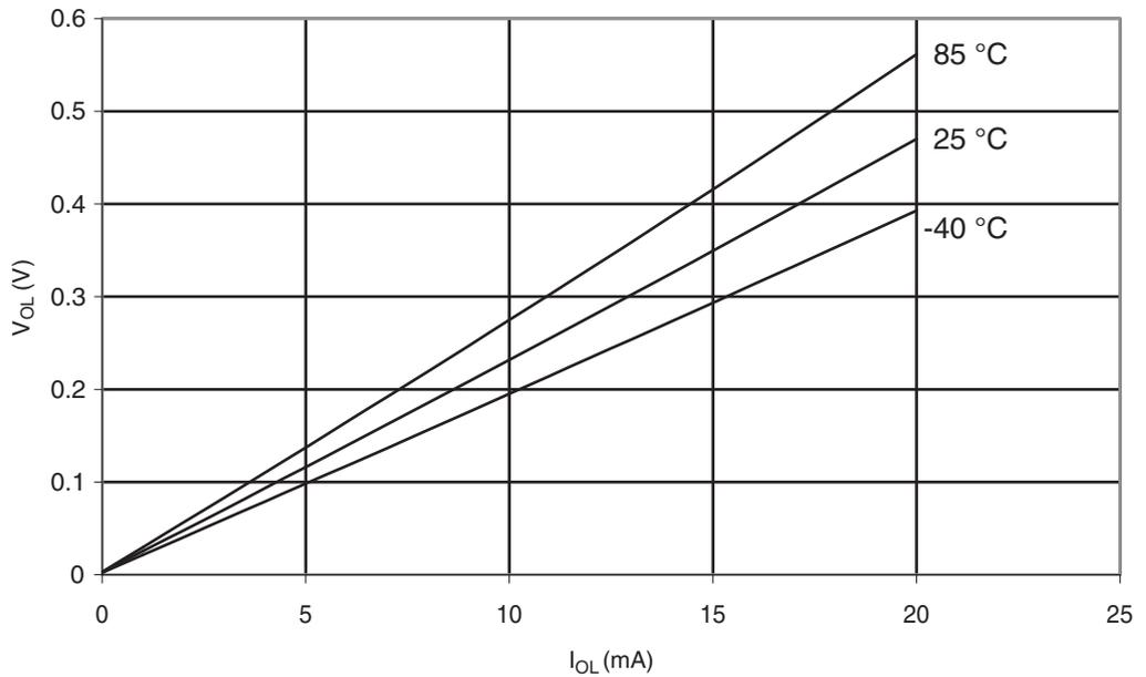
**Figure 6-296.** Atmel® ATmega328P: I/O Pin Output Voltage vs. Source Current ( $V_{CC} = 3V$ )
