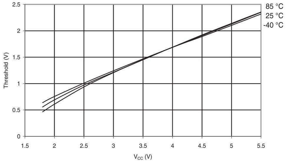
**Figure 6-162.** Atmel® ATmega48PA: I/O Pin Input Hysteresis vs.  $V_{CC}$
