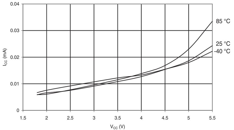
**Figure 6-190.** Atmel® ATmega88PA: Idle Supply Current vs.  $V_{CC}$  (Internal RC Oscillator, 1MHz)
