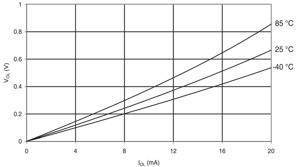
**Figure 6-249.** Atmel ATmega168PA: I/O Pin Output Voltage vs. Sink Current ( $V_{CC} = 5V$ )
