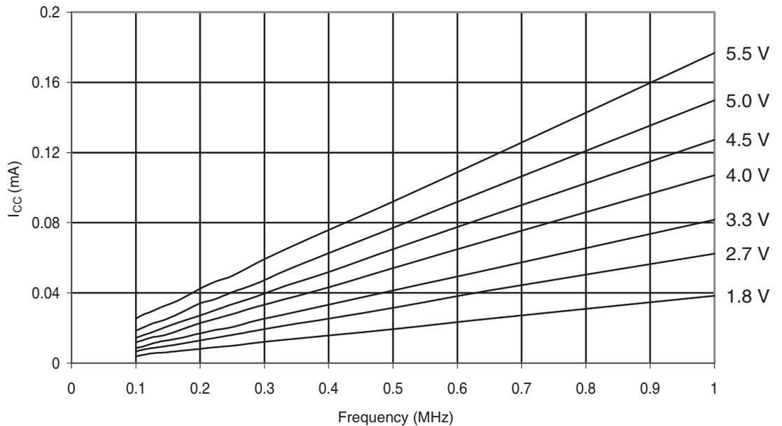
**Figure 6-280.** Atmel® ATmega328P: Idle Supply Current vs. Frequency (1 - 20MHz)
