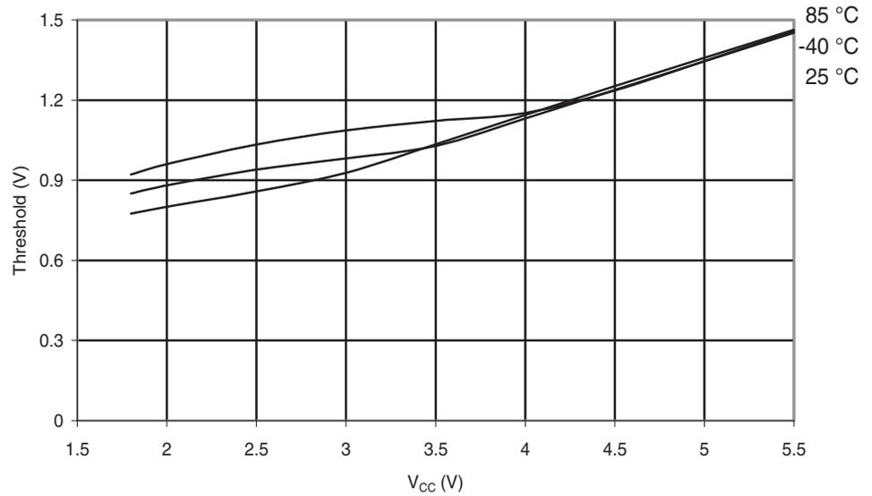
**Figure 6-256.** Atmel® ATmega168PA: Reset Input Threshold Voltage vs.  $V_{CC}$  ( $V_{IL}$ , I/O Pin read as '0')
