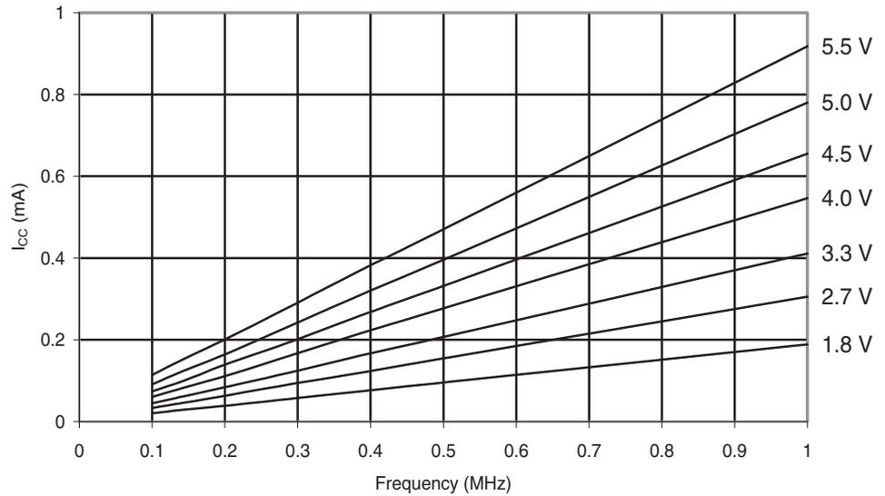
**Figure 6-137.** Atmel ATmega48PA: Active Supply Current vs. Frequency (1-20MHz)
