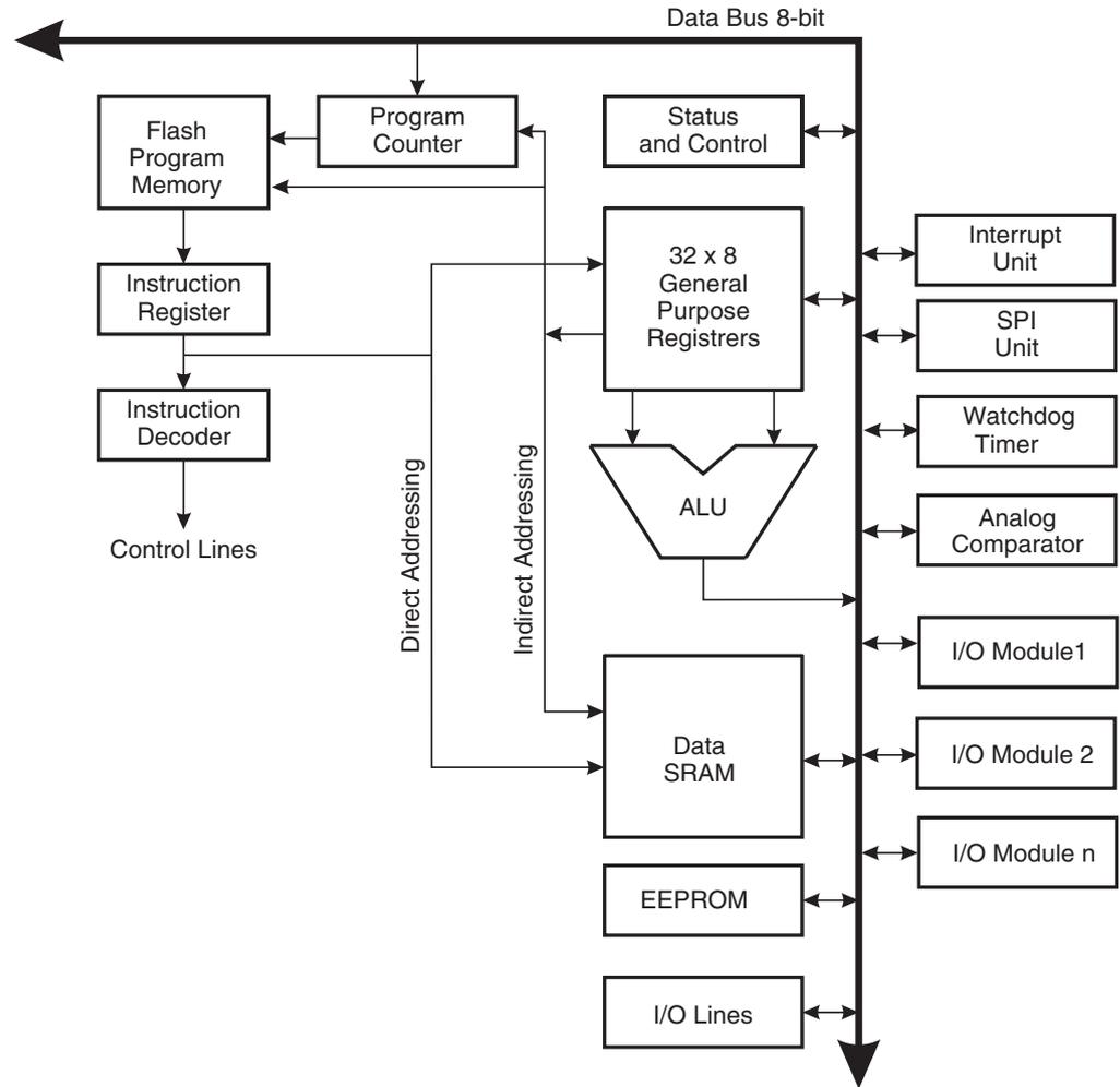
In order to maximize performance and parallelism, the Atmel® AVR uses a Harvard architecture – with separate memories and buses for program and data. Instructions in the program memory are executed with a single level pipelining. While one instruction is being executed, the next instruction is pre-fetched from the program memory. This concept enables instructions to be executed in every clock cycle. The program memory is In-System Reprogrammable Flash memory.
