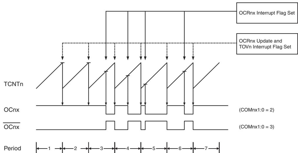
The Timer/Counter Overflow Flag (TOV0) is set each time the counter reaches TOP. If the interrupt is enabled, the interrupt handler routine can be used for updating the compare value.
