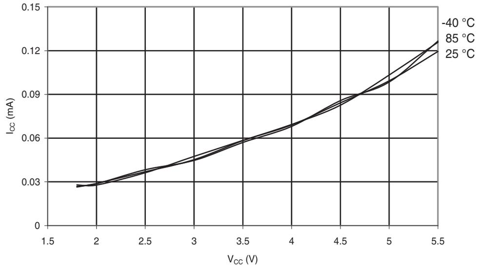
**Figure 6-231.** Atmel ATmega168PA: Active Supply Current vs.  $V_{CC}$  (Internal RC Oscillator, 1MHz)
