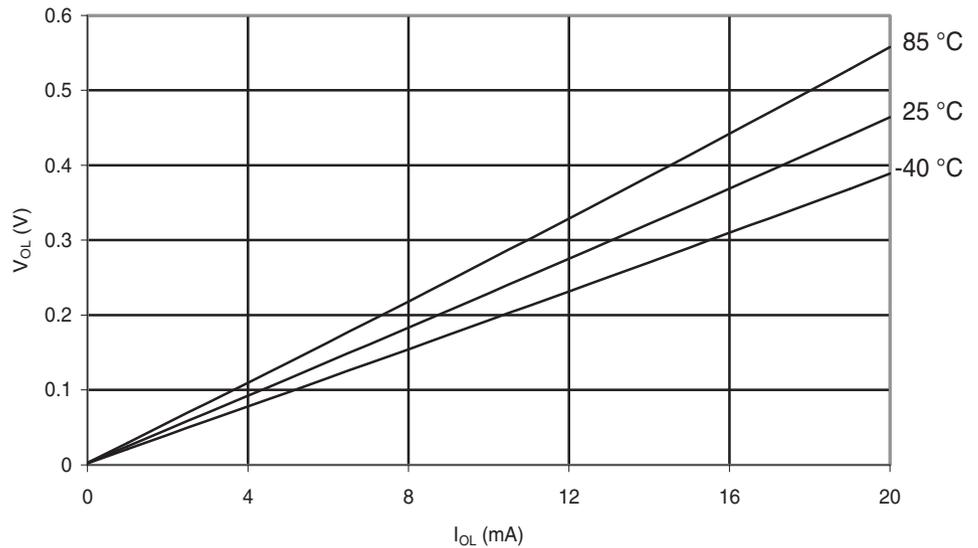
**Figure 6-204.** Atmel® ATmega88PA: I/O Pin Output Voltage vs. Source Current ( $V_{CC} = 3V$ )
