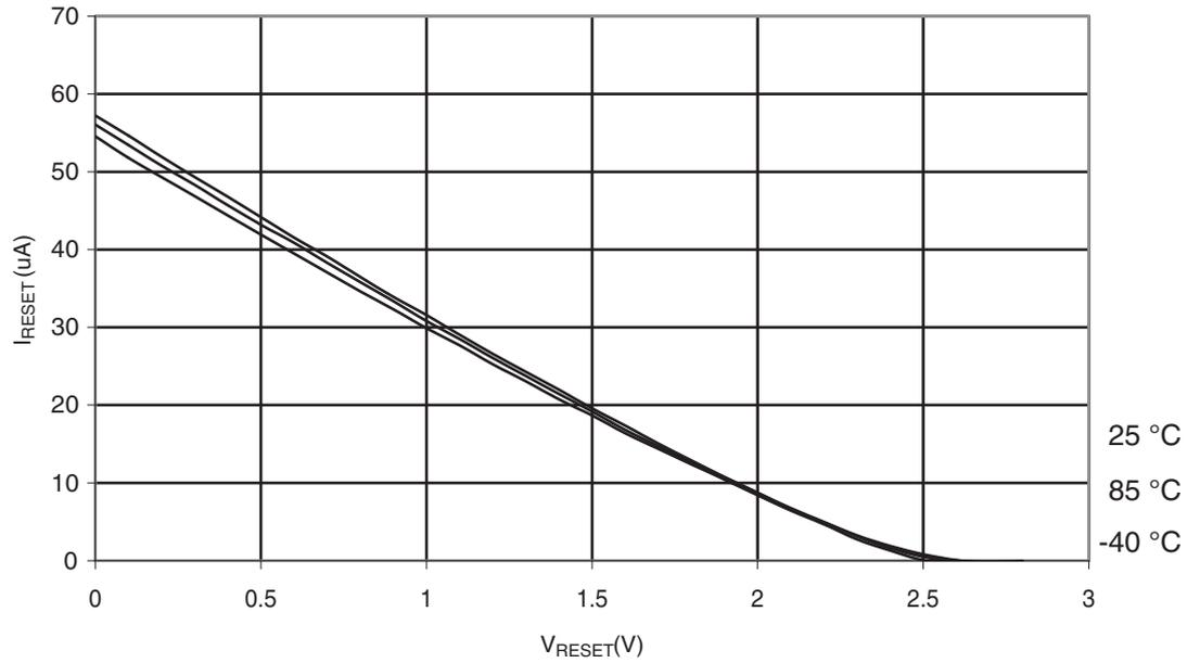
**Figure 6-293.** Atmel ATmega328P: Reset Pull-up Resistor Current vs. Reset Pin Voltage ( $V_{CC} = 5V$ )
