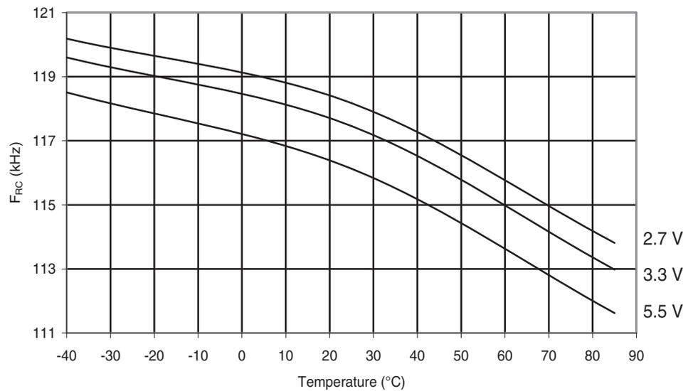
**Figure 6-262.** Atmel® ATmega168PA: Watchdog Oscillator Frequency vs.  $V_{CC}$
