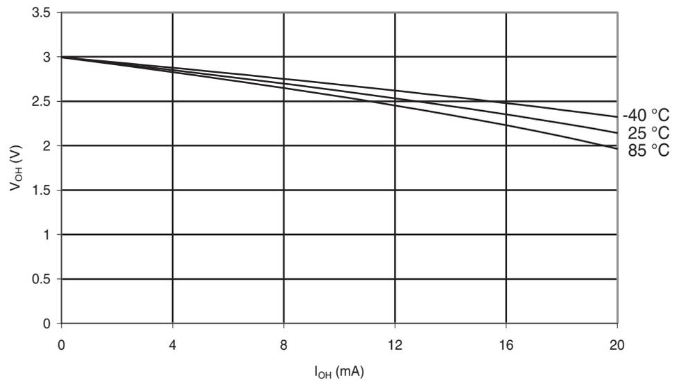
**Figure 6-159.** Atmel ATmega48PA: I/O Pin Output Voltage vs. Source Current ( $V_{CC} = 5V$ )
