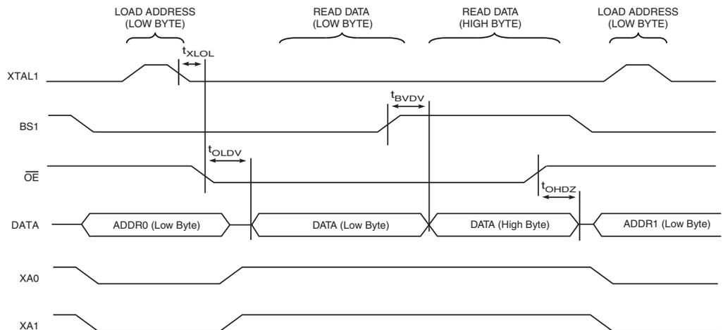
Note: 1. The timing requirements shown in [Figure 6-133](#) (i.e.,  $t_{DVXH}$ ,  $t_{XHL}$ , and  $t_{XLDX}$ ) also apply to reading operation.
