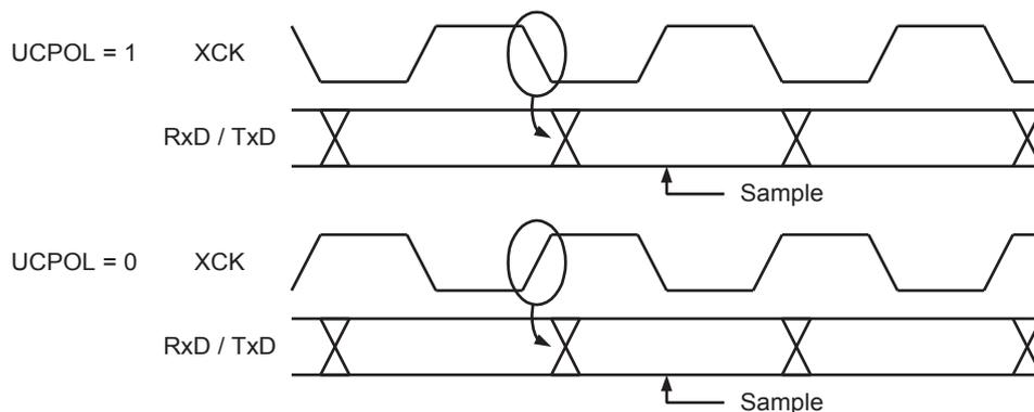
The UC POLn bit UCRSC selects which XCKn clock edge is used for data sampling and which is used for data change. As [Figure 6-72](#) shows, when UC POLn is zero the data will be changed at rising XCKn edge and sampled at falling XCKn edge. If UC POLn is set, the data will be changed at falling XCKn edge and sampled at rising XCKn edge.
