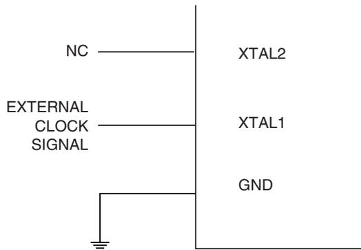
When this clock source is selected, start-up times are determined by the SUT Fuses as shown in [Table 6-19](#).
