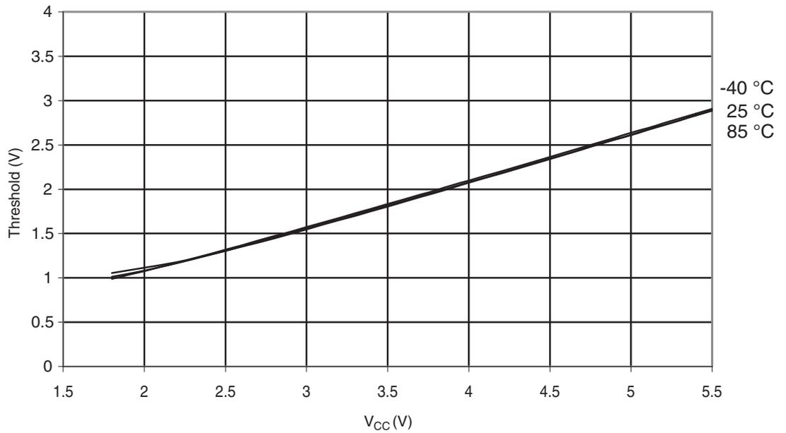
**Figure 6-299.** Atmel ATmega328P: I/O Pin Input Threshold Voltage vs.  $V_{CC}$  ( $V_{IL}$ , I/O Pin read as '0')
