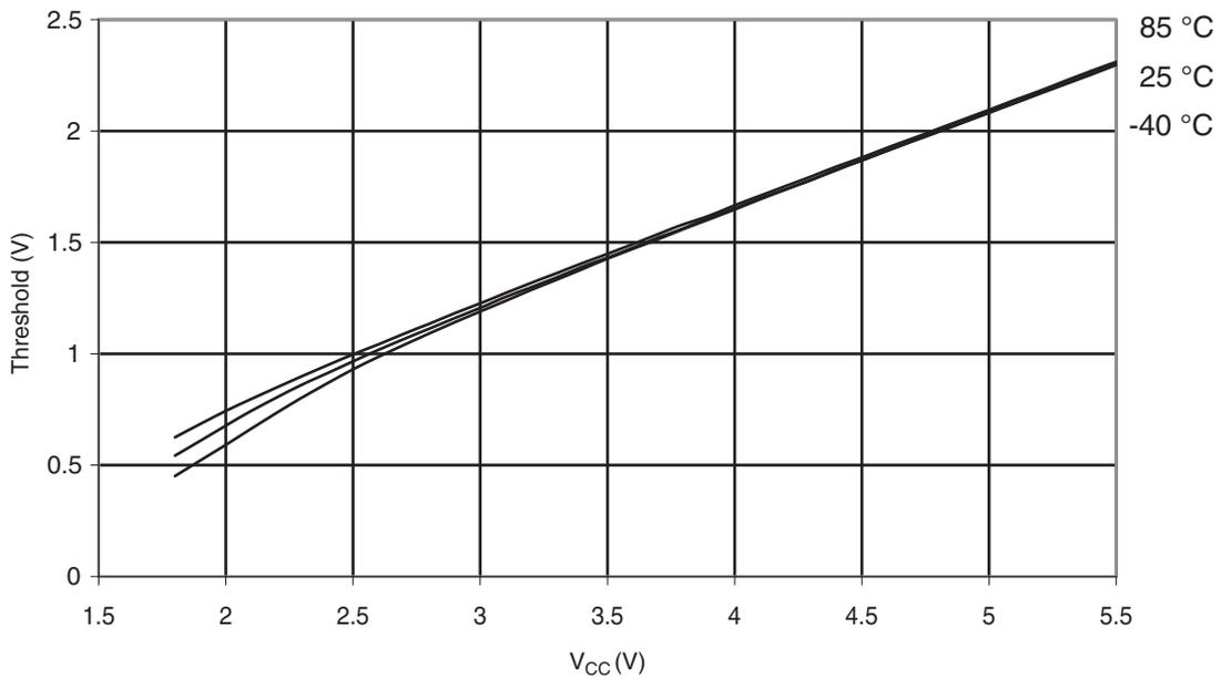
**Figure 6-300.** Atmel® ATmega328P: I/O Pin Input Hysteresis vs.  $V_{CC}$
