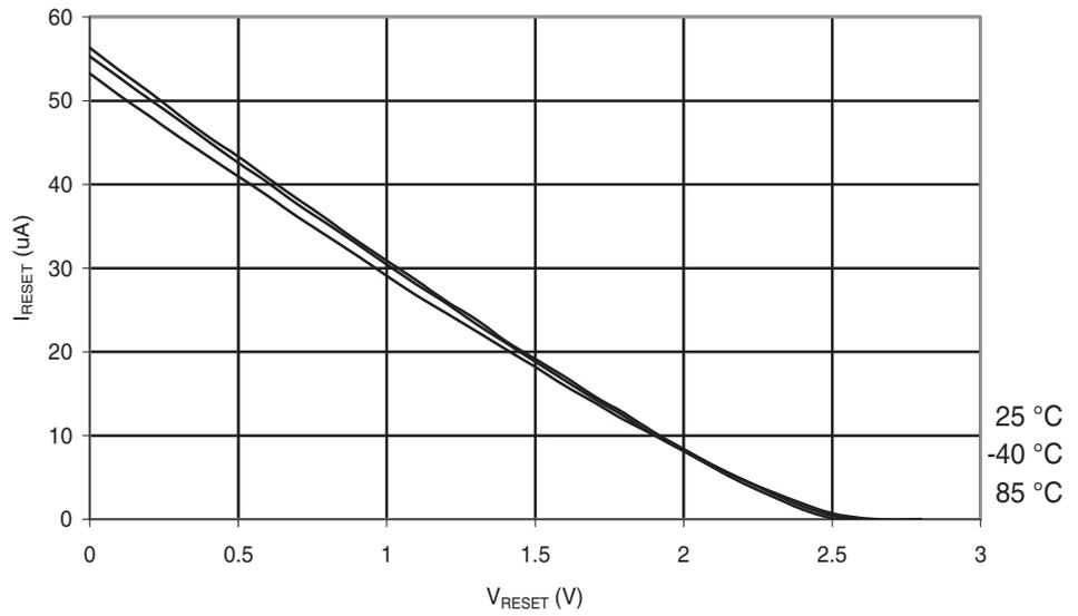
**Figure 6-247.** Atmel ATmega168PA: Reset Pull-up Resistor Current vs. Reset Pin Voltage ( $V_{CC} = 5V$ )
