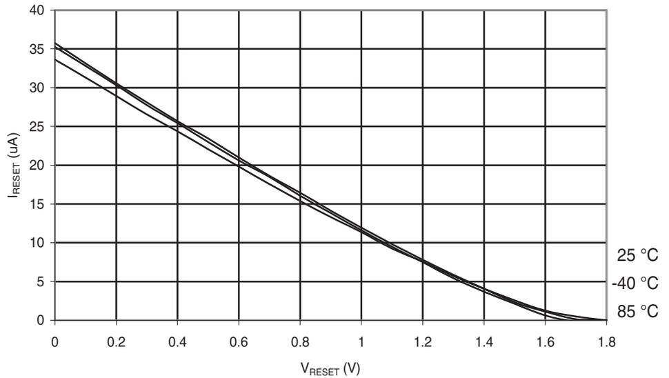
**Figure 6-246.** Atmel® ATmega168PA: Reset Pull-up Resistor Current vs. Reset Pin Voltage ( $V_{CC} = 2.7V$ )
