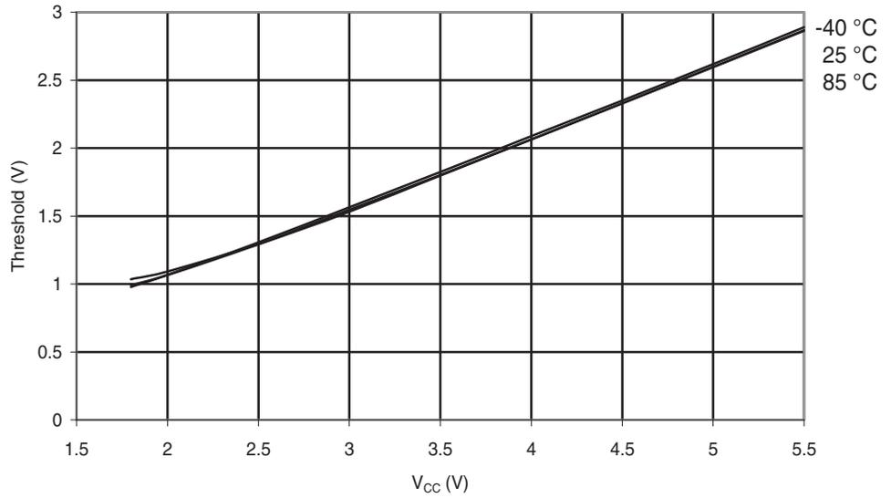
**Figure 6-161.** Atmel ATmega48PA: I/O Pin Input Threshold Voltage vs.  $V_{CC}$  ( $V_{IL}$ , I/O Pin read as '0')
