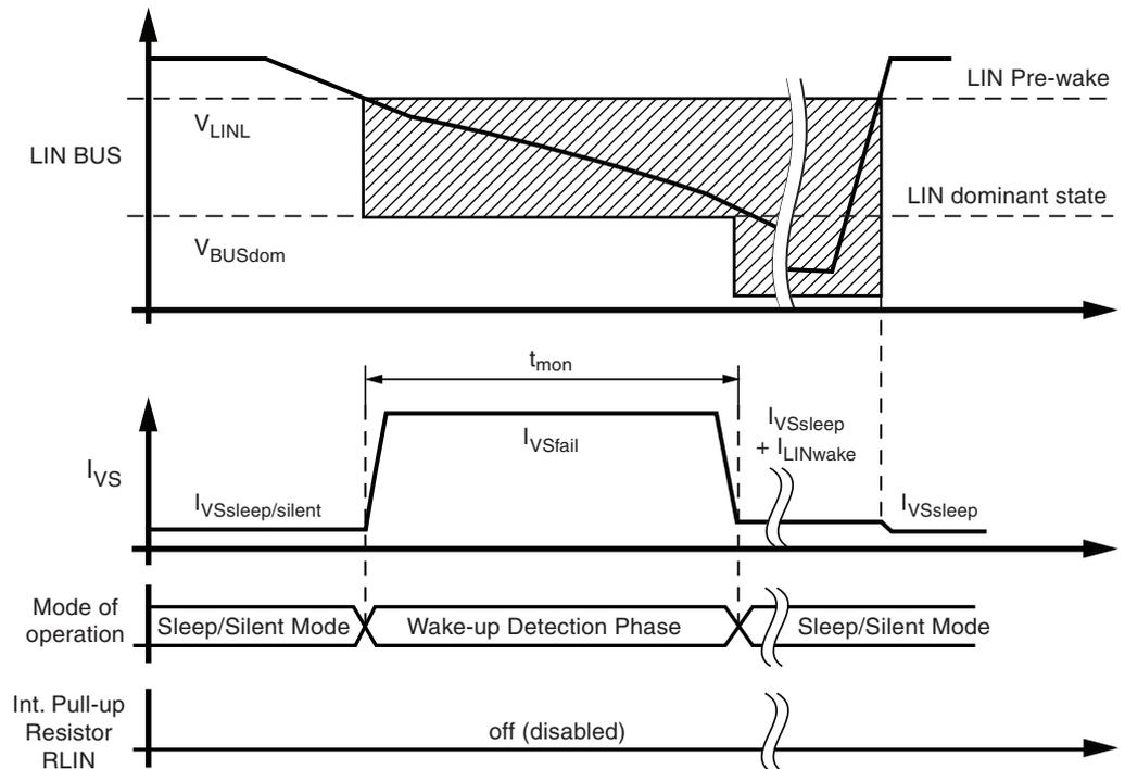
If the Atmel® ATA6630 is in Sleep or Silent Mode and the voltage level at the LIN-bus is in dominant state ( $V_{LIN} < V_{BUSdom}$ ) for a time period exceeding  $t_{mon}$  (during a short circuit at LIN, for example), the IC switches back to Sleep Mode respectively Silent Mode. The  $V_S$  current consumption then consists of  $I_{VSsleep}$  or  $I_{VSsilent}$  plus  $I_{LINWAKE}$ . After a positive edge at pin LIN the IC switches directly to Fail-safe Mode (see [Figure 3-8 on page 16](#)).
