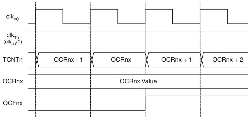
Figure 6-49 shows the same timing data, but with the prescaler enabled.
