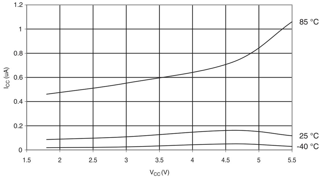
**Figure 6-285.** ATmega328P: Power-Down Supply Current vs.  $V_{CC}$  (Watchdog Timer Enabled)
