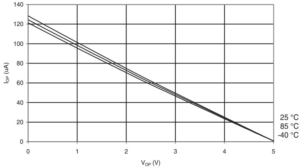
**Figure 6-153.** Atmel ATmega48PA: Reset Pull-up Resistor Current vs. Reset Pin Voltage ( $V_{CC} = 1.8V$ )
