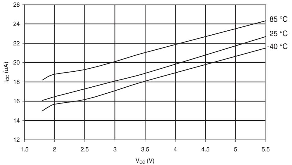
**Figure 6-270.** Atmel® ATmega168PA: Programming Current vs.  $V_{CC}$
