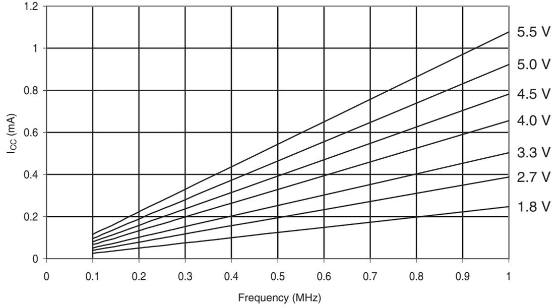
**Figure 6-275.** Atmel ATmega328P: Active Supply Current vs. Frequency (1 - 20MHz)
