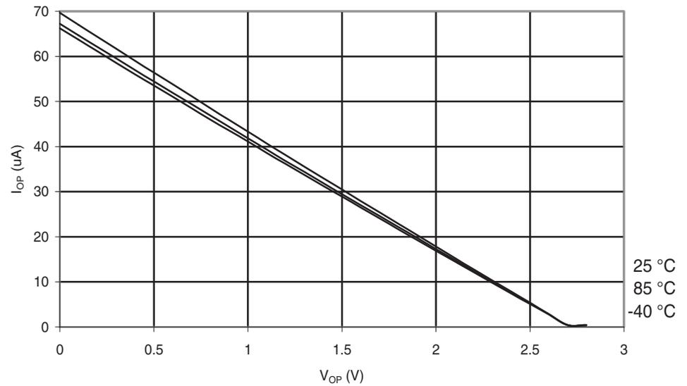
**Figure 6-152.** Atmel® ATmega48PA: I/O Pin Pull-up Resistor Current vs. Input Voltage ( $V_{CC} = 5V$ )
