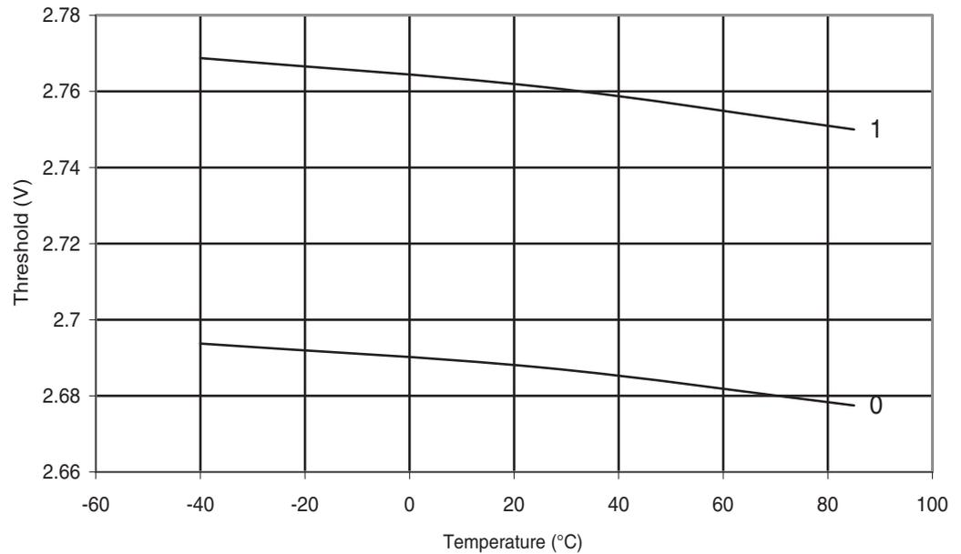
**Figure 6-306.** Atmel® ATmega328P: BOD Thresholds vs. Temperature (BODLEVEL is 4.3V)
