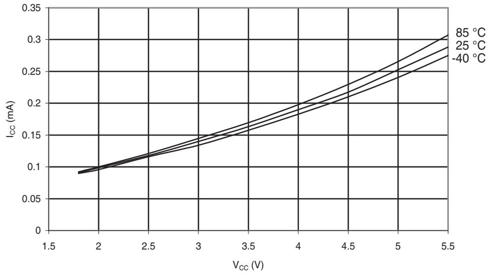
**Figure 6-145.** Atmel ATmega48PA: Idle Supply Current vs.  $V_{CC}$  (Internal RC Oscillator, 8MHz)
