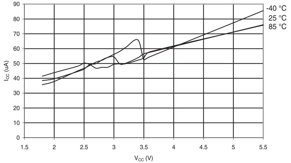
**Figure 6-176.** Atmel® ATmega48PA: AREF External Reference Current vs.  $V_{CC}$
