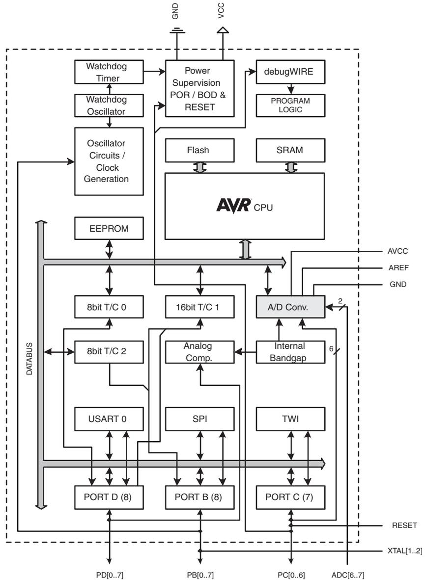
The AVR<sup>®</sup> core combines a rich instruction set with 32 general purpose working registers. All the 32 registers are directly connected to the Arithmetic Logic Unit (ALU), allowing two independent registers to be accessed in one single instruction executed in one clock cycle. The resulting architecture is more code efficient while achieving throughputs up to ten times faster than conventional CISC microcontrollers.
