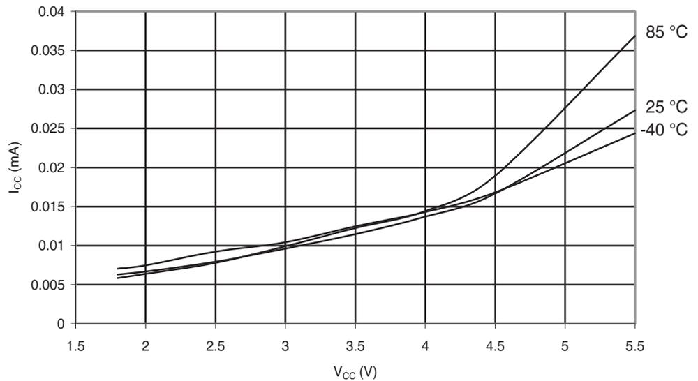
**Figure 6-236.** Atmel® ATmega168PA: Idle Supply Current vs.  $V_{CC}$  (Internal RC Oscillator, 1MHz)
