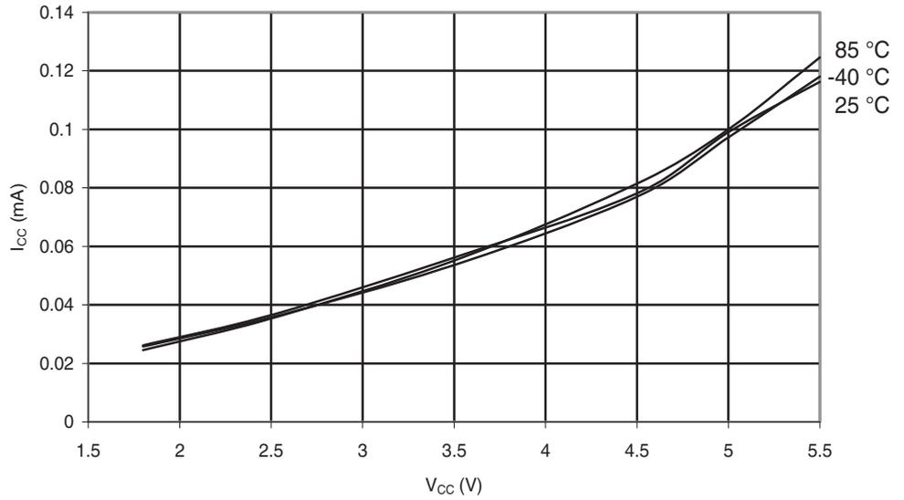
**Figure 6-139.** Atmel ATmega48PA: Active Supply Current vs.  $V_{CC}$  (Internal RC Oscillator, 1MHz)
