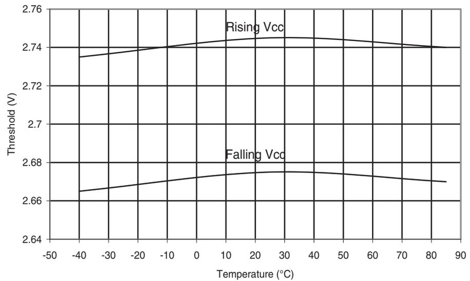
**Figure 6-214.** Atmel® ATmega88PA: BOD Thresholds vs. Temperature (BODLEVEL is 4.3V)
