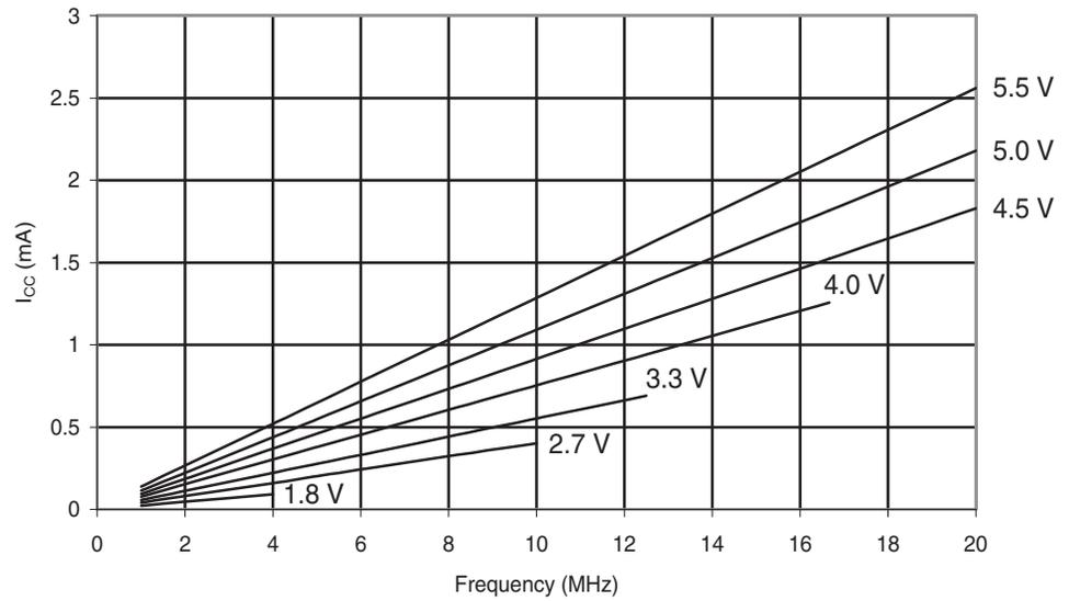
**Figure 6-235.** Atmel® ATmega168PA: Idle Supply Current vs.  $V_{CC}$  (Internal RC Oscillator, 128kHz)
