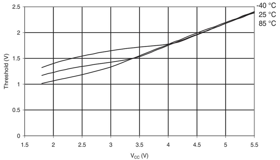
**Figure 6-164.** Atmel® ATmega48PA: Reset Input Threshold Voltage vs.  $V_{CC}$  ( $V_{IL}$ , I/O Pin read as '0')
