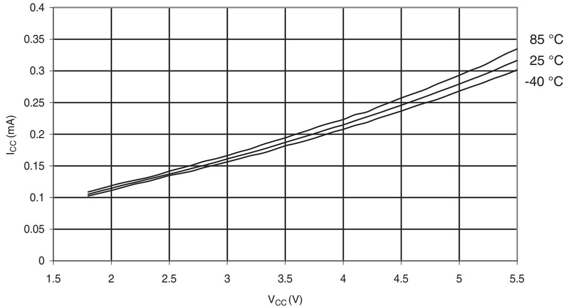
**Figure 6-283.** Atmel ATmega328P: Idle Supply Current vs.  $V_{CC}$  (Internal RC Oscillator, 8MHz)
