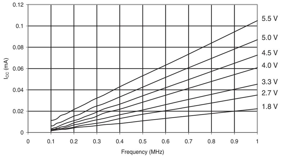
**Figure 6-226.** Atmel® ATmega88PA: Reset Supply Current vs. Frequency (1 - 20MHz)
