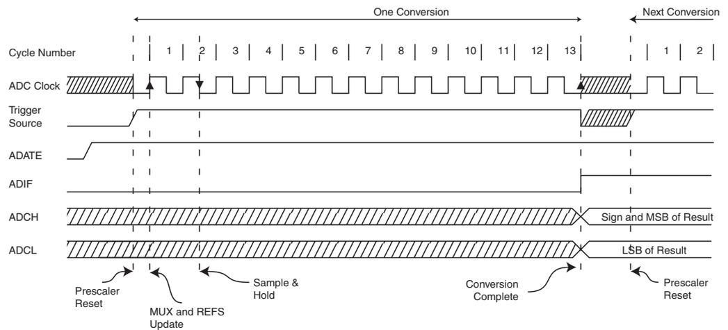
**Figure 6-107. ADC Timing Diagram, Free Running Conversion**
