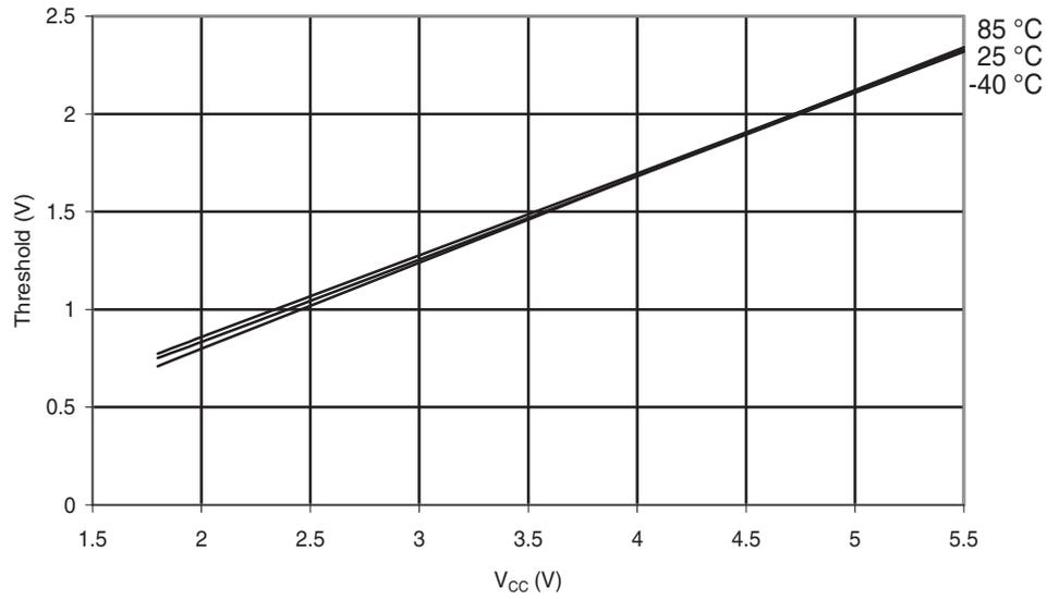
**Figure 6-165.** Atmel ATmega48PA: Reset Pin Input Hysteresis vs.  $V_{CC}$
