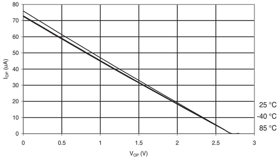
**Figure 6-198.** Atmel® ATmega88PA: I/O Pin Pull-up Resistor Current vs. Input Voltage ( $V_{CC} = 5V$ )
