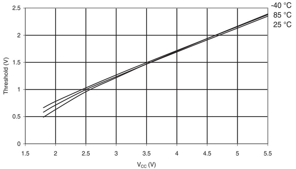
**Figure 6-208.** Atmel® ATmega88PA: I/O Pin Input Hysteresis vs.  $V_{CC}$
