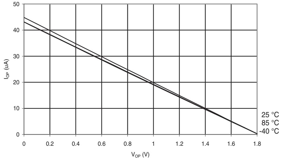
**Figure 6-151.** Atmel ATmega48PA: I/O Pin Pull-up Resistor Current vs. Input Voltage ( $V_{CC} = 2.7 V$ )
