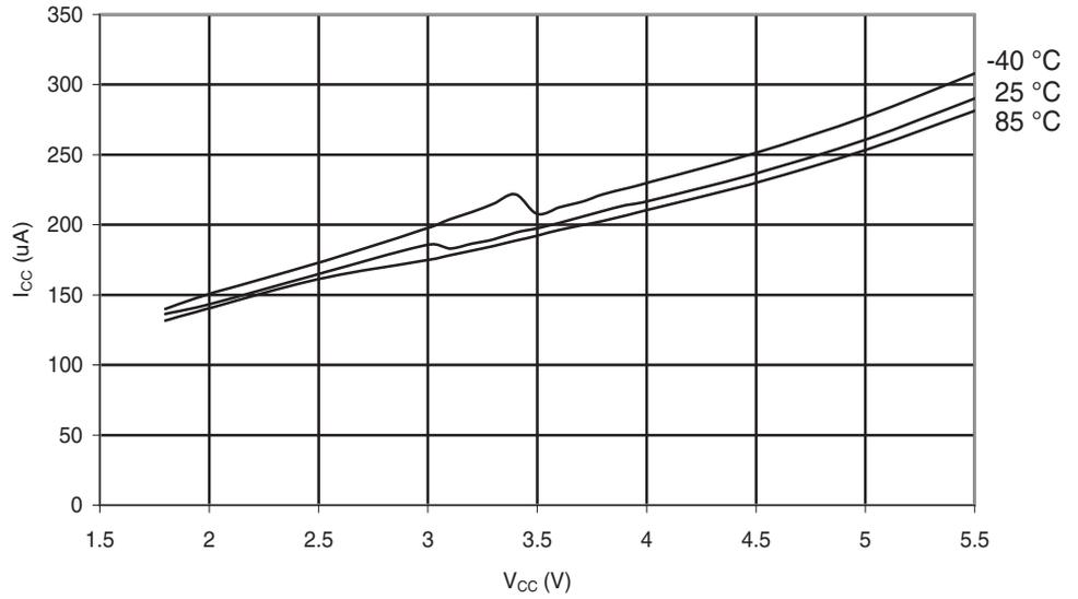
**Figure 6-175.** Atmel ATmega48PA: Analog Comparator Current vs.  $V_{CC}$
