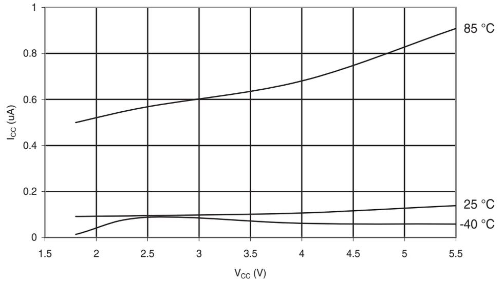
**Figure 6-239.** Atmel ATmega168PA: Power-Down Supply Current vs.  $V_{CC}$  (Watchdog Timer Enabled)
