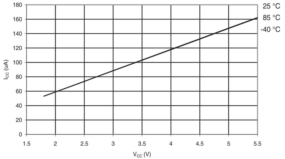
**Figure 6-269.** Atmel ATmega168PA: Brownout Detector Current vs.  $V_{CC}$
