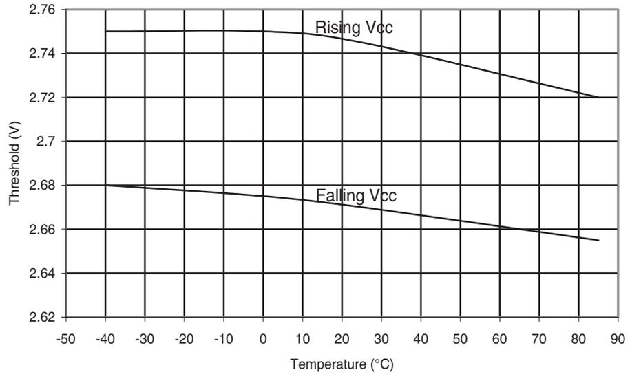
**Figure 6-168.** Atmel® ATmega48PA: BOD Thresholds vs. Temperature (BODLEVEL is 4.3V)
