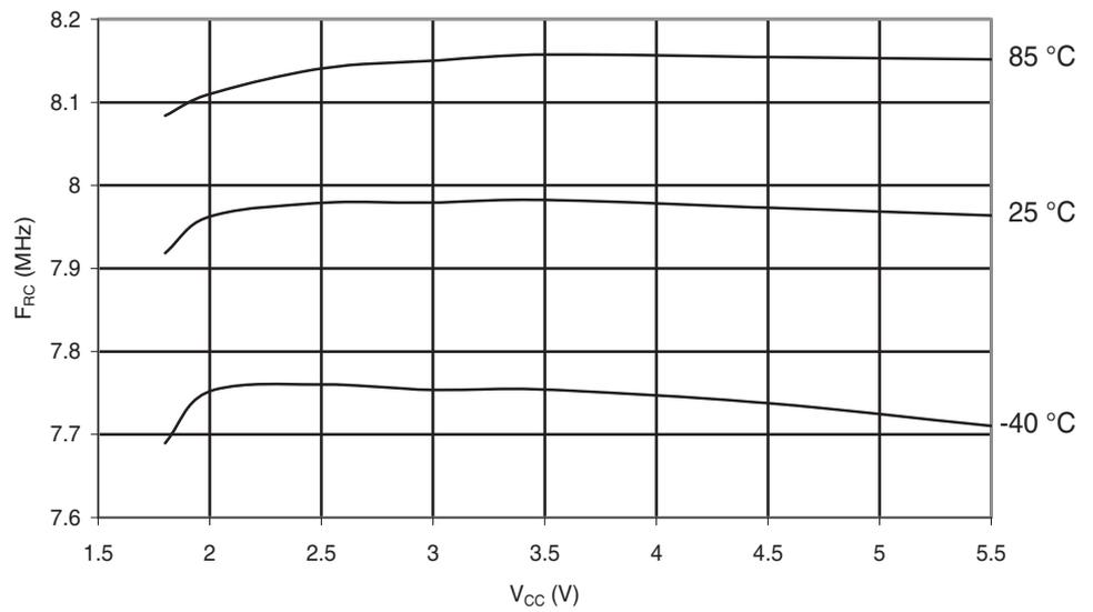
**Figure 6-172.** Atmel® ATmega48PA: Calibrated 8MHz RC Oscillator Frequency vs. Temperature
