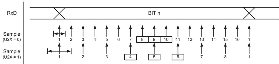
The decision of the logic level of the received bit is taken by doing a majority voting of the logic value to the three samples in the center of the received bit. The center samples are emphasized on the figure by having the sample number inside boxes. The majority voting process is done as follows: If two or all three samples have high levels, the received bit is registered to be a logic 1.
