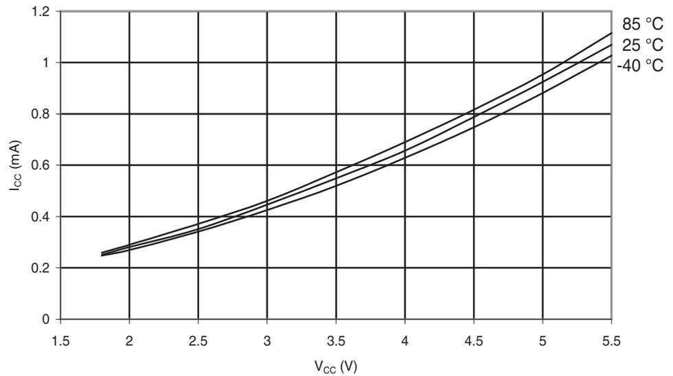
**Figure 6-140.** Atmel® ATmega48PA: Active Supply Current vs.  $V_{CC}$  (Internal RC Oscillator, 8MHz)
