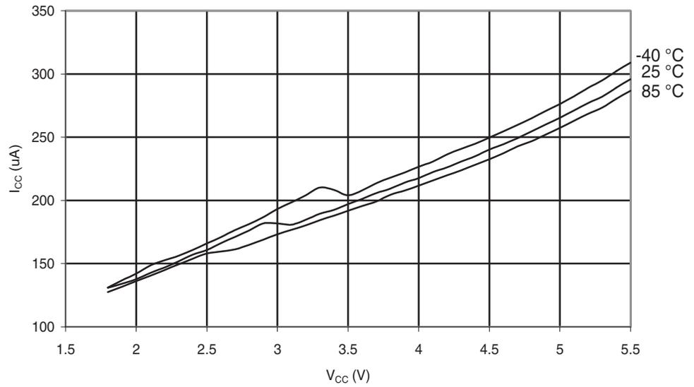
**Figure 6-267.** Atmel ATmega168PA: Analog Comparator Current vs.  $V_{CC}$
