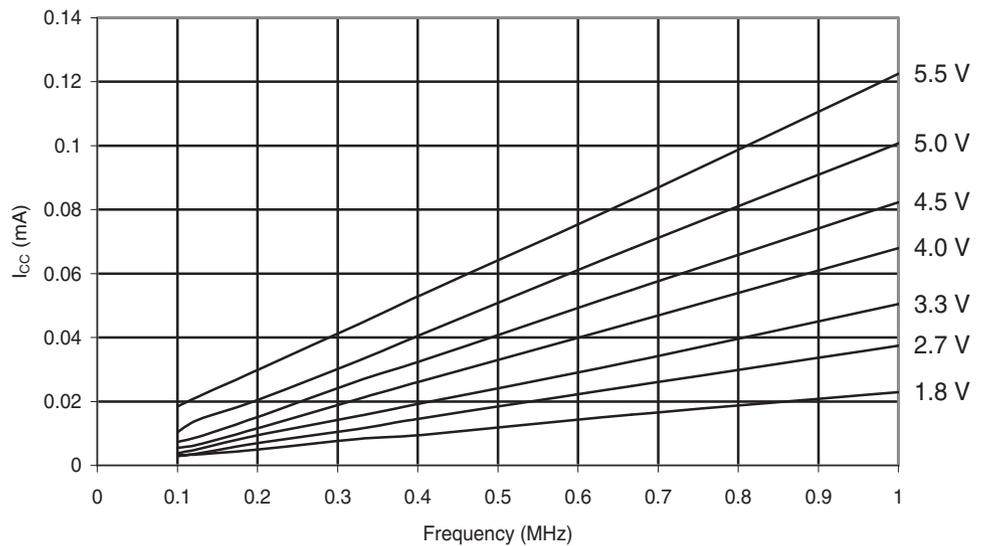
**Figure 6-180.** Atmel® ATmega48PA: Reset Supply Current vs. Frequency (1 - 20MHz)
