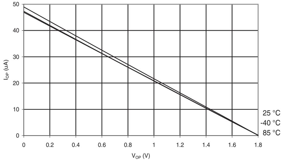
**Figure 6-197.** Atmel ATmega88PA: I/O Pin Pull-up Resistor Current vs. Input Voltage ( $V_{CC} = 2.7V$ )
