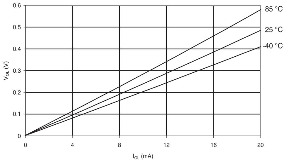
**Figure 6-158.** Atmel® ATmega48PA: I/O Pin Output Voltage vs. Source Current ( $V_{CC} = 3V$ )
