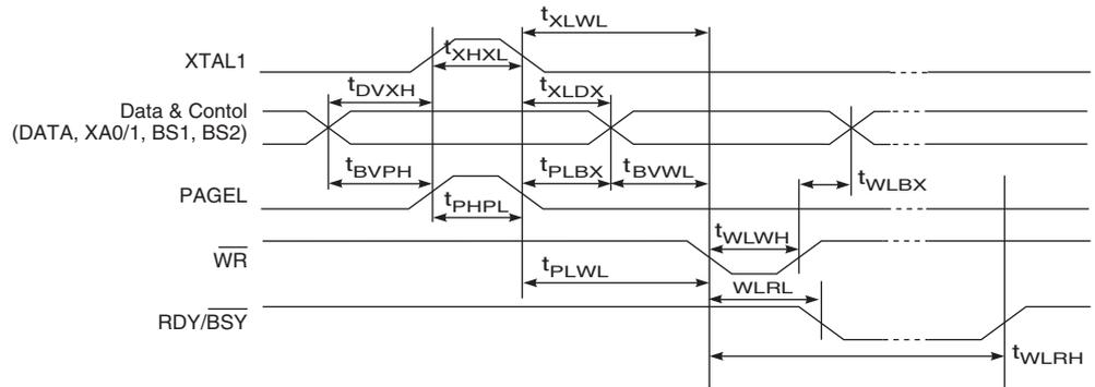
**Figure 6-134. Parallel Programming Timing, Loading Sequence with Timing Requirements<sup>(1)</sup>**
