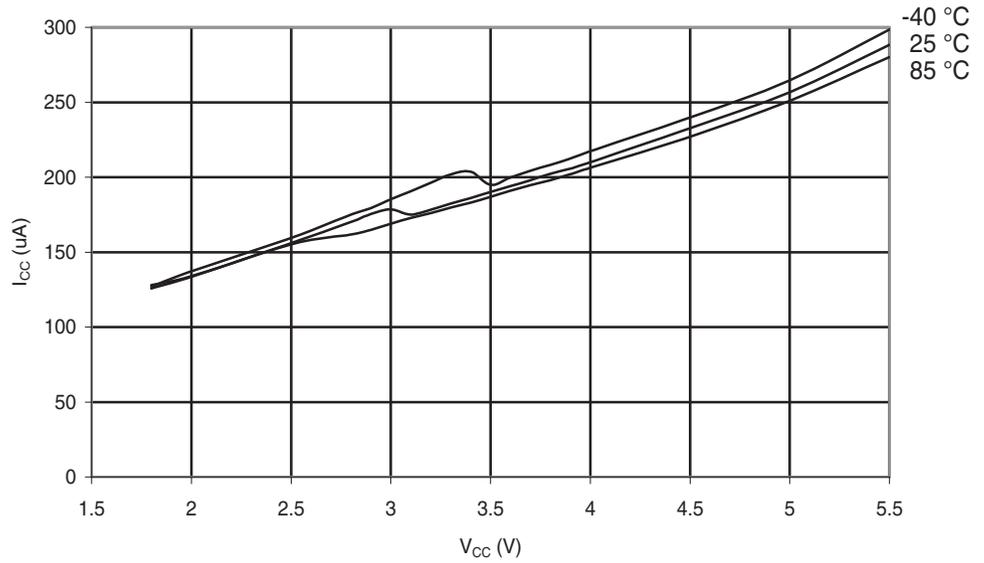
**Figure 6-221.** Atmel ATmega88PA: Analog Comparator Current vs.  $V_{CC}$
