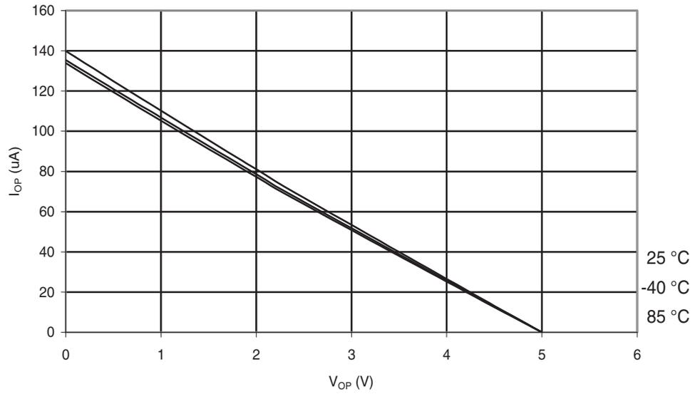
**Figure 6-245.** Atmel ATmega168PA: Reset Pull-up Resistor Current vs. Reset Pin Voltage ( $V_{CC} = 1.8V$ )
