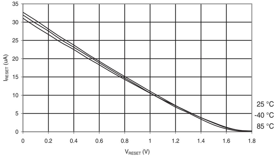
**Figure 6-154.** Atmel® ATmega48PA: Reset Pull-up Resistor Current vs. Reset Pin Voltage ( $V_{CC} = 2.7V$ )
