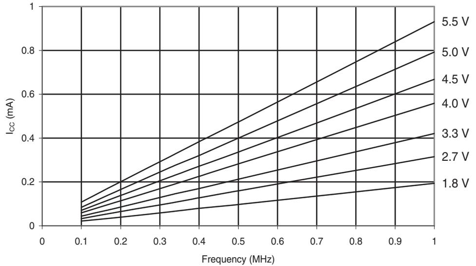
**Figure 6-183.** Atmel ATmega88PA: Active Supply Current vs. Frequency (1 - 20MHz)
