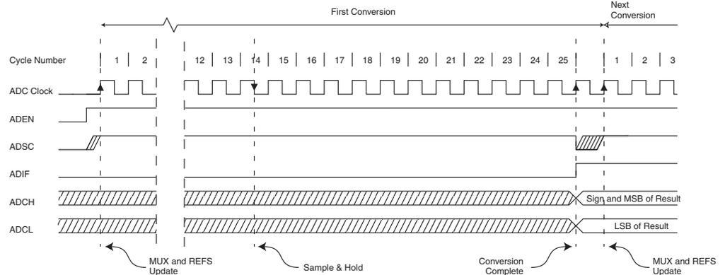
**Figure 6-105. ADC Timing Diagram, Single Conversion**
