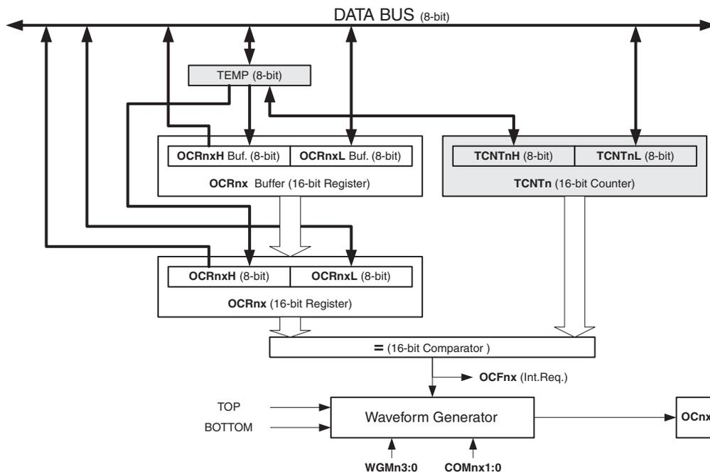
The OCR1x Register is double buffered when using any of the twelve *Pulse Width Modulation* (PWM) modes. For the Normal and *Clear Timer on Compare* (CTC) modes of operation, the double buffering is disabled. The double buffering synchronizes the update of the OCR1x Compare Register to either TOP or BOTTOM of the counting sequence.
