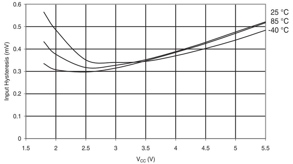
**Figure 6-209.** Atmel ATmega88PA: Reset Input Threshold Voltage vs.  $V_{CC}$  ( $V_{IH}$ , I/O Pin read as '1')
