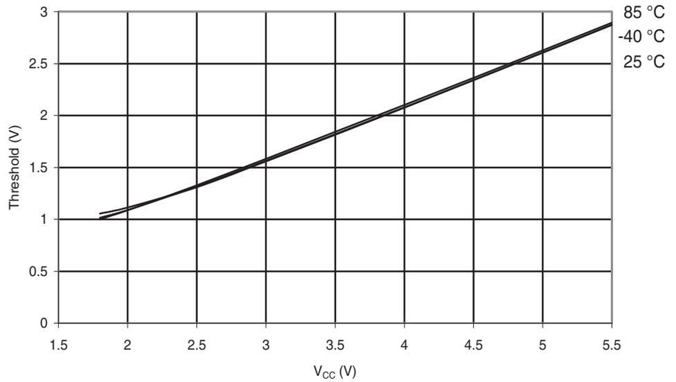
**Figure 6-207.** Atmel ATmega88PA: I/O Pin Input Threshold Voltage vs.  $V_{CC}$  ( $V_{IL}$ , I/O Pin read as '0')
