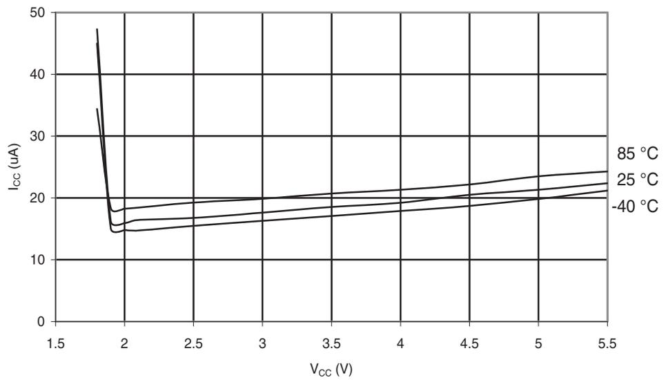
**Figure 6-224.** Atmel® ATmega88PA: Programming Current vs.  $V_{CC}$
