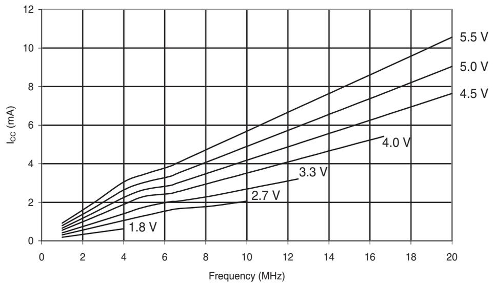
**Figure 6-230.** Atmel® ATmega168PA: Active Supply Current vs.  $V_{CC}$  (Internal RC Oscillator, 128kHz)
