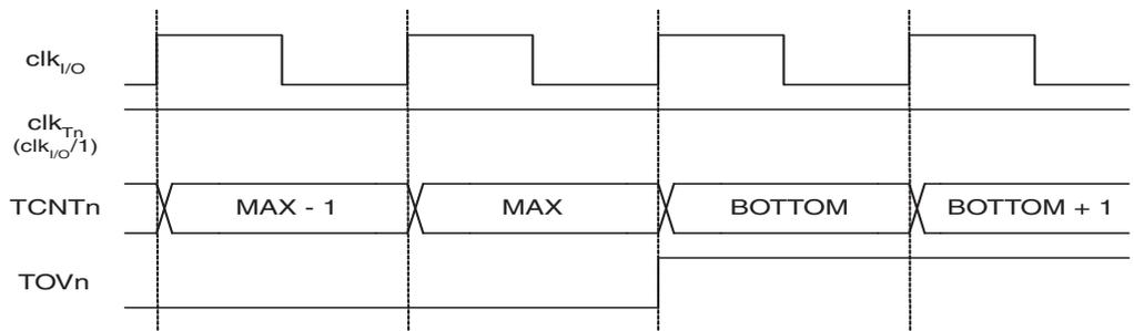
[Figure 6-62](#) shows the same timing data, but with the prescaler enabled.
