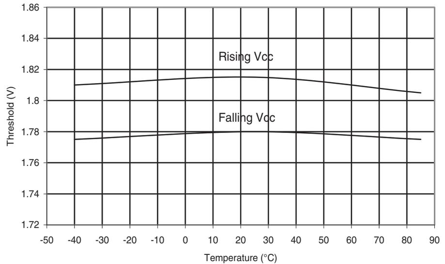
**Figure 6-259.** Atmel ATmega168PA: BOD Thresholds vs. Temperature (BODLEVEL is 2.7V)
