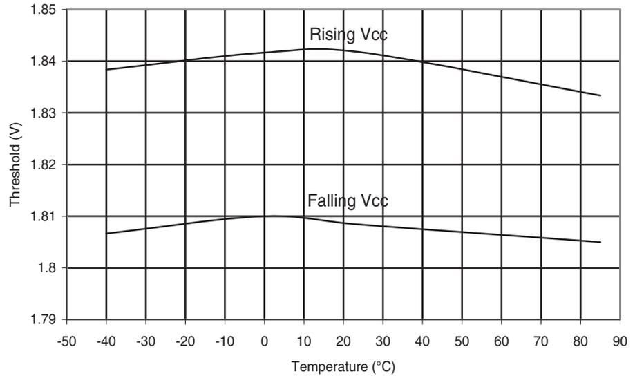
**Figure 6-167.** Atmel ATmega48PA: BOD Thresholds vs. Temperature (BODLEVEL is 2.7V)
