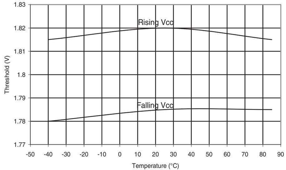
**Figure 6-213.** Atmel ATmega88PA: BOD Thresholds vs. Temperature (BODLEVEL is 2.7V)
