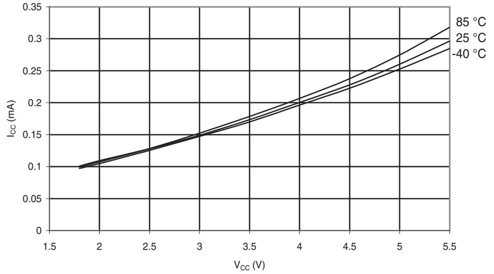
**Figure 6-191.** Atmel ATmega88PA: Idle Supply Current vs.  $V_{CC}$  (Internal RC Oscillator, 8MHz)
