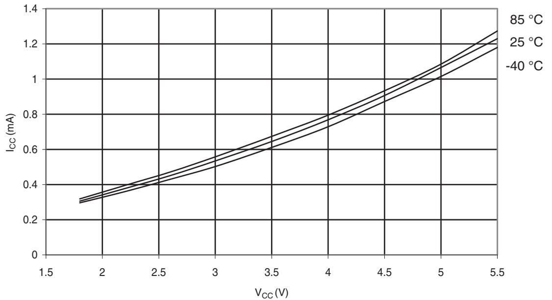
**Figure 6-278.** Atmel® ATmega328P: Active Supply Current vs.  $V_{CC}$  (Internal RC Oscillator, 8MHz)
