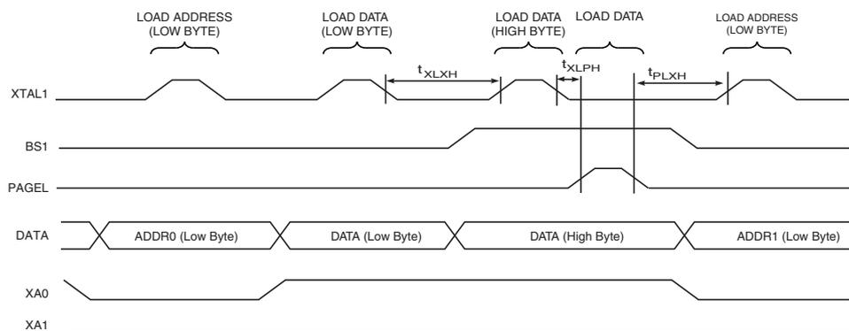
Note: 1. The timing requirements shown in [Figure 6-133](#) (i.e.,  $t_{DVXH}$ ,  $t_{XHL}$ , and  $t_{XLDX}$ ) also apply to loading operation.
