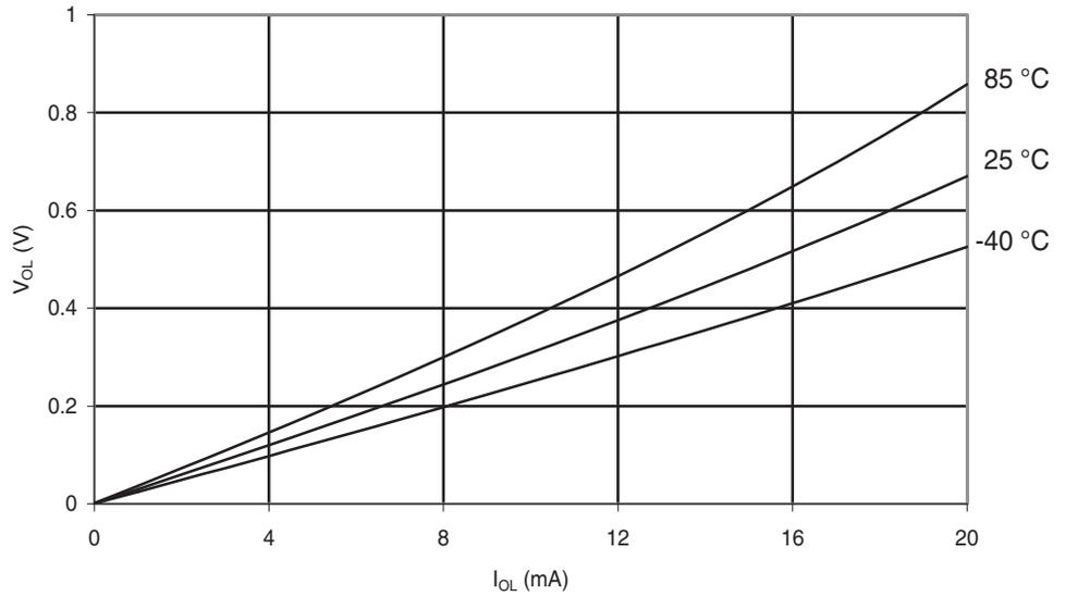
**Figure 6-203.** Atmel ATmega88PA: I/O Pin Output Voltage vs. Sink Current ( $V_{CC} = 5V$ )
