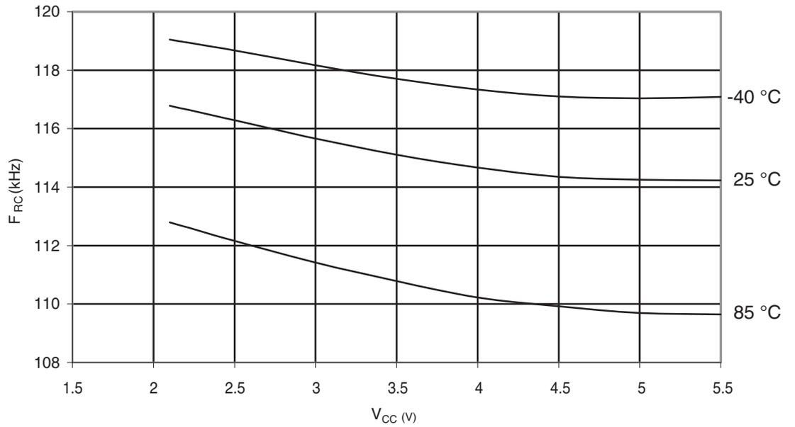
**Figure 6-309.** Atmel ATmega328P: Calibrated 8MHz RC Oscillator Frequency vs.  $V_{CC}$
