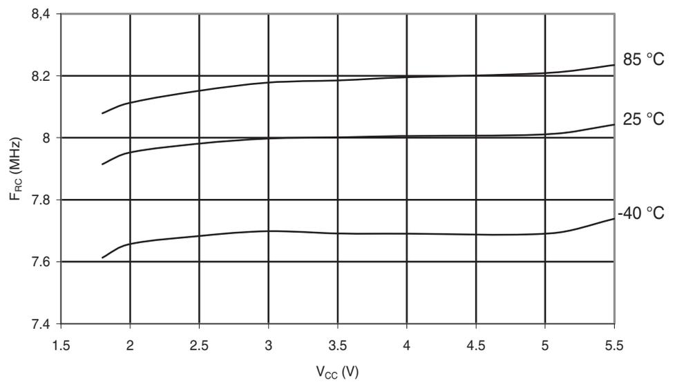
**Figure 6-264.** Atmel® ATmega168PA: Calibrated 8MHz RC Oscillator Frequency vs. Temperature
