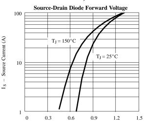
V<sub>SD</sub> - Source-to-Drain Voltage (V)
