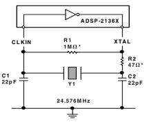
R2 SHOULD BE CHOSEN TO LIMIT CRYSTAL DRIVE POWER. REFER TO CRYSTAL MANUFACTURER'S SPECIFICATIONS
