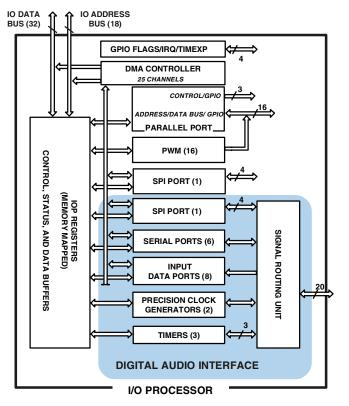
Figure 3. ADSP-21363 I/O Processor and Peripherals Block Diagram
