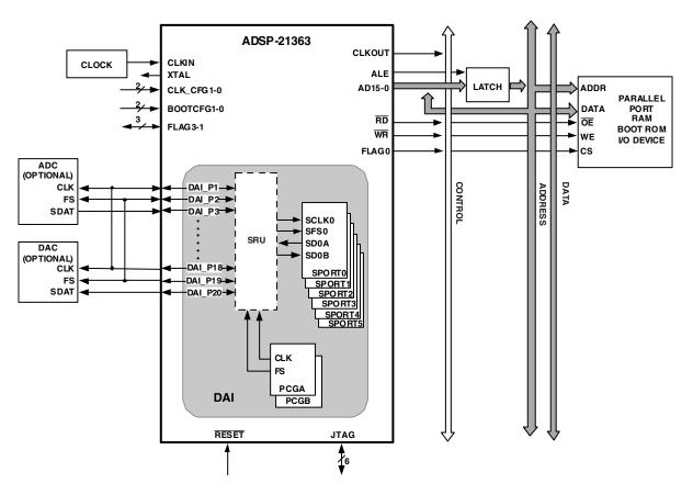
Figure 2. ADSP-21363 System Sample Configuration
