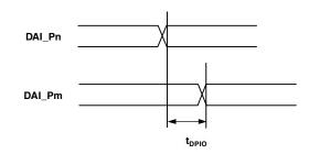
Figure 14. DAI Pin to Pin Direct Routing
