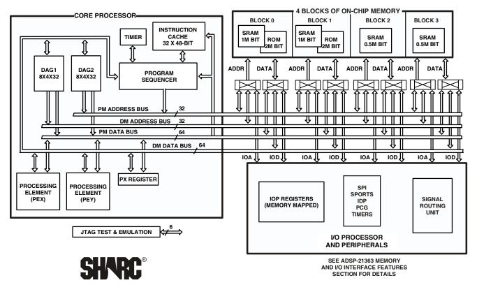
Figure 1. Functional Block Diagram—Processor Core
