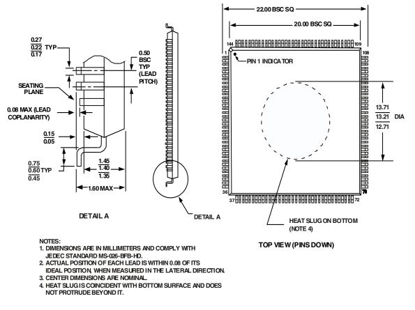
Figure 35. 144-Lead Low Profile Quad Flat Package, with Integrated Heatsink [LQFP\_INT\_HS] (SQ-144-3)
