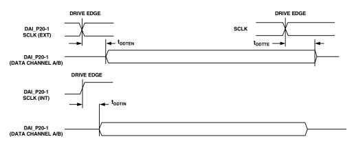
Figure 22. Serial Ports
