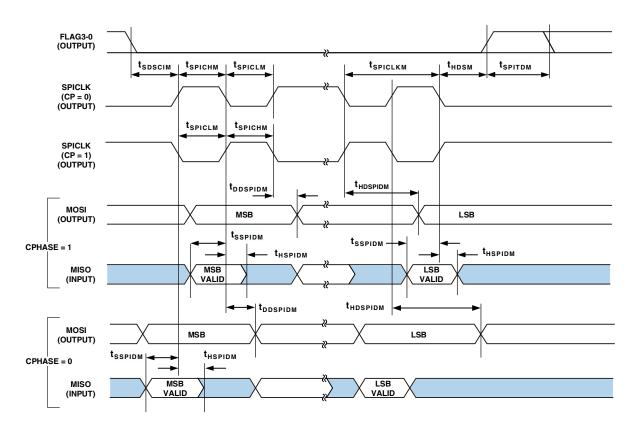
Figure 25. SPI Master Timing
