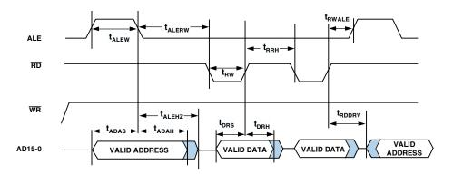
NOTE: FOR 16-BIT MEMORY READS, WHEN EMPP  $\neq$  0, ONLY ONE  $\overline{\text{RD}}$  PULSE OCCURS BETWEEN ALE CYCLES. WHEN EMPP = 0, MULTIPLE  $\overline{\text{RD}}$  PULSES OCCUR BETWEEN ALE CYCLES. FOR COMPLETE INFORMATION, SEE THE ADSP-2136X SHARC PROCESSOR HARDWARE REFERENCE.
