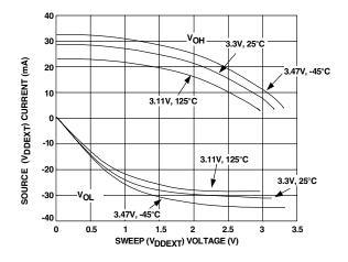
Figure 28. ADSP-21363 Typical Drive
