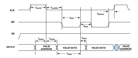
NOTE: FOR 16-BIT MEMORY WRITES, WHEN EMPP ▷ 0, ONLY ONE WR PULSE OCCURS BETWEEN ALE CYCLES. WHEN EMPP = 0, MULTIPLE WR PULSES OCCUR BETWEEN ALE CYCLES. FOR COMPLETE INFORMATION, SEE THE ADSP-2136X SHARC PROCESSOR HARDWARE REFERENCE.
