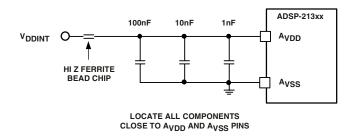
Figure 4. Analog Power (A<sub>VDD</sub>) Filter Circuit
