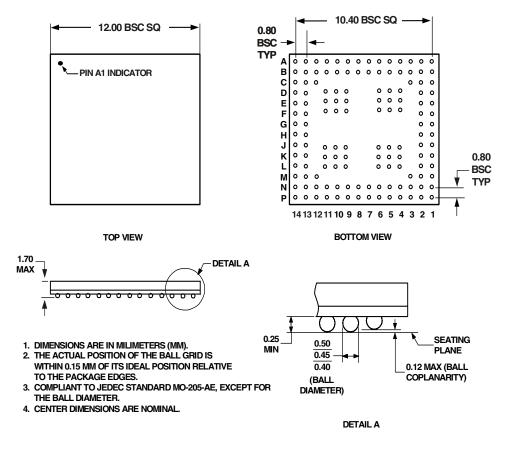
Figure 36. 136-Lead Chip Scale Package Ball Grid Array [CSP\_BGA](BC-136-2)
