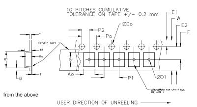
REEL DIMENSIONS inches 7.0 26.0 13.0 А 177.8 254.0 330.2 mm inches 2.50 4.00 3.75 В mm 63.5 101.6 95.3 Tape Width С mm 13.0 +0.5 / -0.2 D mm 16.4 16.4 16.4 16.0 +2.0 +2.0 +2.0
