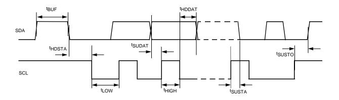
Figure 2. M\_BUS TIMING
