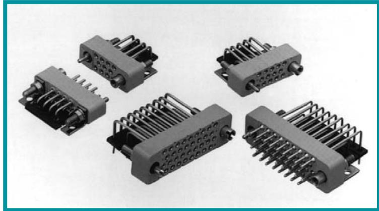
SMPL Series connectors are high reliability, high density, rectangular connectors meeting the performance requirements of MIL-DTL-28748. Termination style is right angle printed board mount. SMPL Series connectors are interchangeable with Positronic SGM and SGMC series connectors.
