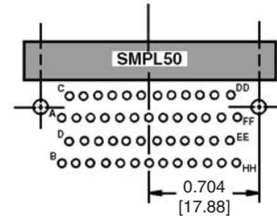
SUGGEST 0.105 [2.66] Ø HOLES IN PRINTED BOARD FOR CONNECTOR MOUNTING HOLES
