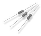
The resistive element comprises a metal oxide film deposited on a ceramic former. The element is protected by a flameproof coating which will withstand overload conditions without flame or mechanical damage. They are recommended for use in applications such as line protection etc...
