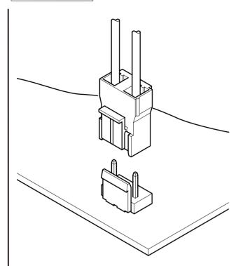
7.92mm pitch crimp style, large current carrying capacity connector, that is best suited for various kinds of power supply circuits. Box-shaped contacts offer reliable connection.
