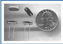
Monitor Products' MS49 and SMS49 crystals greatly reduce the space required by conventional MM49 mounted crystals. Their low height allows them to be vertically mounted between circuit boards and affords superior protection against shock and vibration. Our resistance-welded packages offer excellent aging characteristics and may be used with all types of wave soldering and vapor cleaning equipment.
