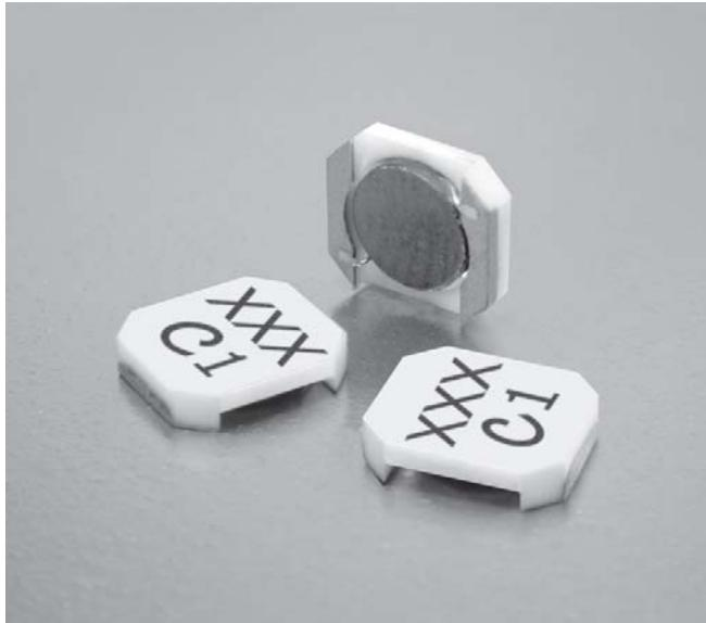
LPO4815 power inductors share the same footprint as our LPO4812 series (4,6 x 4,8 mm), but their 0,3 mm extra height allows them to handle up to 35% more current. A rugged ceramic case completely protects the winding and provides an ideal surface for pick and place handling.
