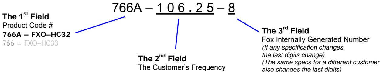
This example, **FXO-HC325R-106.25** = HCMOS Output, Ceramic 3.2 x 2.5mm Package, 2.5V, ±50 PPM Stability, -40 to +85°C Temperature Range, at 106.25 MHz
