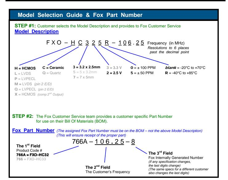
This example, FXO-HC325R-106.25 = HCMOS Output, Ceramic 3.2 x 2.5mm Package, 2.5V,  $\pm$ 50 PPM Stability, -40 to +85°C Temperature Range, at 106.25 MHz
