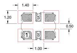
Note: XpressO HCMOS XO's are designed to fit on industry standard, 4 pad layouts.
