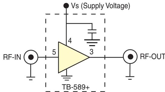
**Fig 1.** Block Diagram of Test Circuit used for characterization. (DUT soldered on Mini-Circuits Characterization Test Fixture TB-589+) Gain, Return loss, Output power at 1dB compression (P1 dB), Output IP3 (OIP3) and Noise Figure measured using Agilent’s N5242A PNA-X microwave network analyzer.
