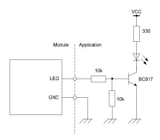
Figure 5.14-1 Recommended circuit for an LED
