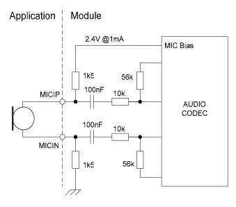
Figure 5.9–1 Microphone connections to the wireless modem
