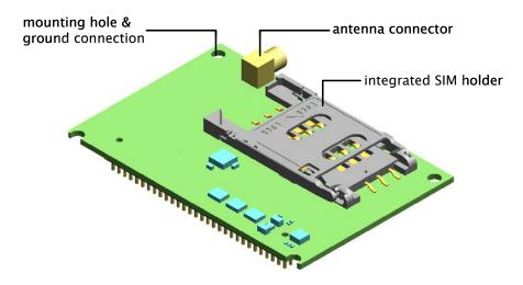
Figure 4.1–2 Wireless modem, viewed from above (Integrated SIM holder variant)
