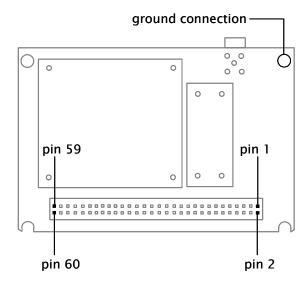
Figure 5.1-1 Wireless modem, viewed from underneath
