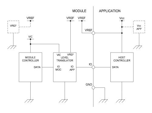
Figure 5.6-1 Level shifter arrangement
