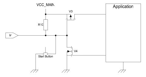
Figure 5.20-3 Example of host wake-up circuit
