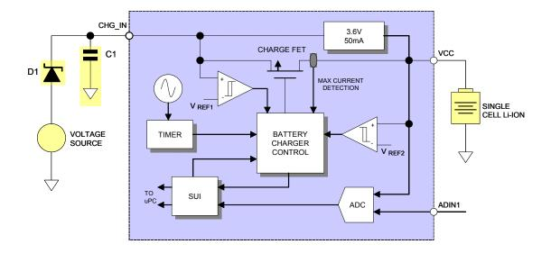
Figure 5.7-1 Typical application for pulse charging a battery
