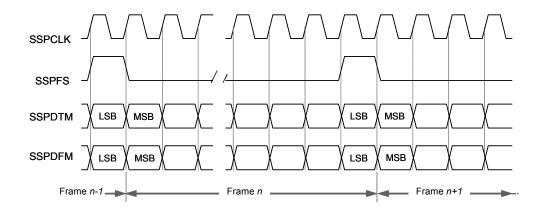
Figure 5.10-3 PCM Frame format for a continuous transfer
