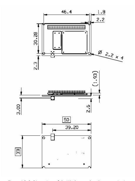
Figure 4.2–2 Dimensions of the Wireless modem (Legacy variant)
