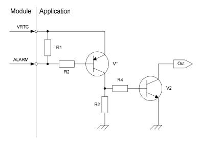
Figure 5.20-2 Typical host-side circuit for ALARM output
