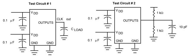
For parameter t<sub>8</sub> (output slew rate) on -1H devices
