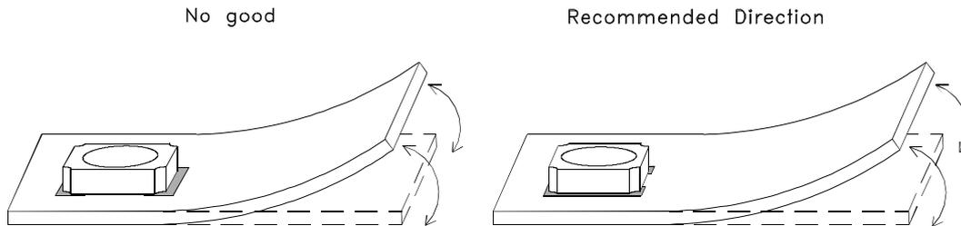
Appropriate LED mounting is to place perpendicularly against the stress affected side.
