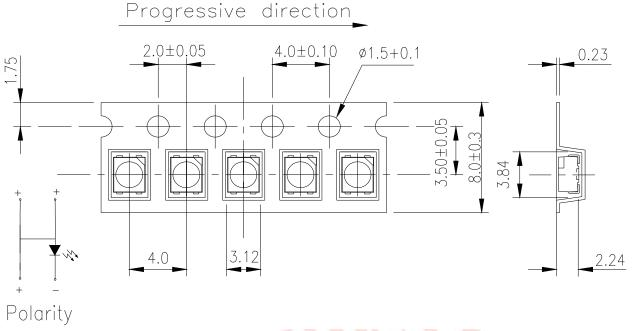
**Note:** Tolerances Unless Dimension  $\pm 0.1$ mm, Unit = mm
