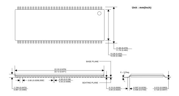
**Note** : Package do not mold protrusion. Allowable protrusion of both sides is 0.4mm.
