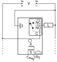
$\label{eq:constraint} \begin{array}{l} C = Common, \mbox{ Transfer Contact} \\ NO = \mbox{ Normally Open } L = Load \\ NOTE: \mbox{ A knob, or terminals } 4 \& 5 \mbox{ are only included} \\ on \mbox{ adjustable units. } R_T \mbox{ is used when external} \\ \mbox{ adjustment is ordered. } Relay \mbox{ contacts are not} \\ \mbox{ isolated. } Dashed \mbox{ lines are internal connections.} \end{array}$
