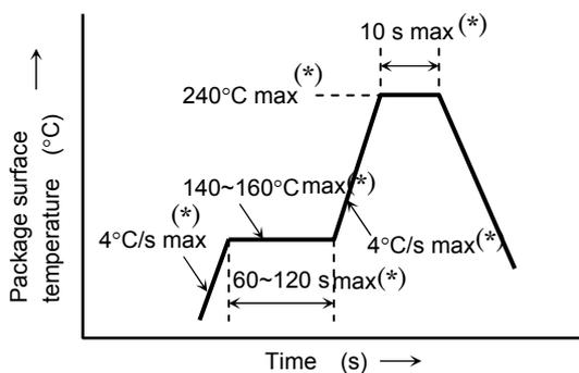
Temperature profile for Pb-free soldering (example)
