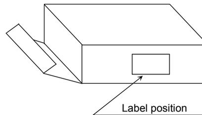
• The aluminum package in which the reel is supplied also has a copy of the label attached to the center of one side.
