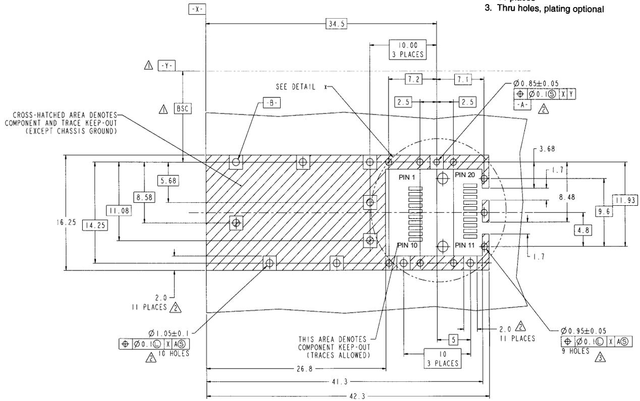
Figure 5. SFP Host Board Mechanical Layout (Cont.)
