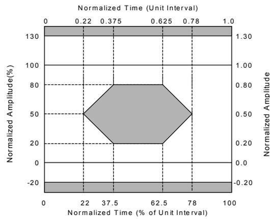
Figure 8. Eye Diagram Mask for Optical Output ( IEEE 802.3 )
