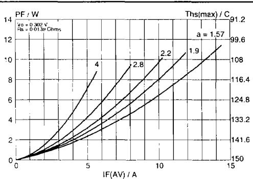
Fig.2. Maximum forward dissipation  $P_F = f(I_{F(AV)})$ ; sinusoidal current waveform where  $a = \text{form factor} = I_{F(RMS)} / I_{F(AV)}$ .
