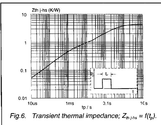
Fig.6. Transient thermal impedance;  $Z_{thj-hs} = f(t_p)$ .
