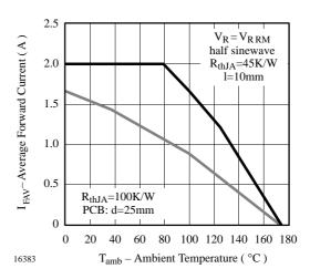
Figure 3. Max. Average Forward Current vs.
