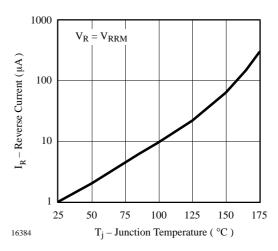
Figure 4. Reverse Current vs. Junction Temperature
