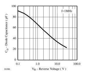
Figure 6. Diode Capacitance vs. Reverse Voltage
