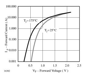
Figure 2. Forward Current vs. Forward Voltage
