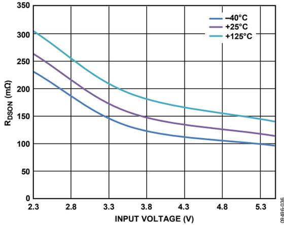
Figure 15.  $R_{DS(on)}$  PFET vs. Input Voltage, Across Temperature
