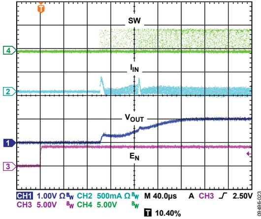
Figure 27. Startup,  $V_{OUT} = 0.8\text{ V}$ ,  $I_{OUT} = 10\text{ mA}$
