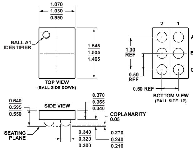
Figure 39. 6-Ball Wafer Level Chip Scale Package [WLCSP]
