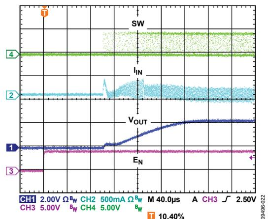
Figure 26. Startup,  $V_{OUT} = 1.8$  V,  $I_{OUT} = 10$  mA
