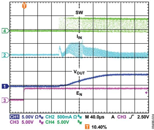
Figure 28. Startup,  $V_{OUT} = 0.8\text{ V}$ ,  $I_{OUT} = 10\text{ mA}$
