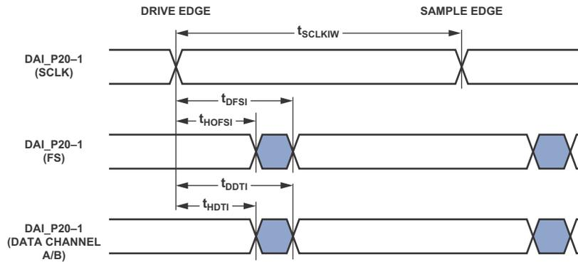
Figure 35. S/PDIF Receiver Internal Digital PLL Mode Timing
