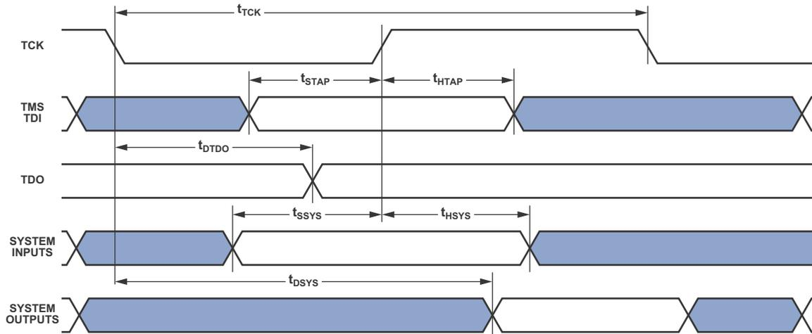
Figure 46. IEEE 1149.1 JTAG Test Access Port
