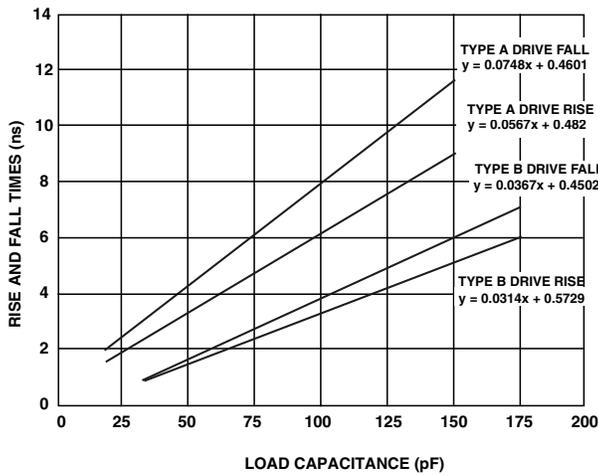
Figure 51. Typical Output Rise/Fall Time (20% to 80%,  $V_{DD\_EXT} = Min$ )
