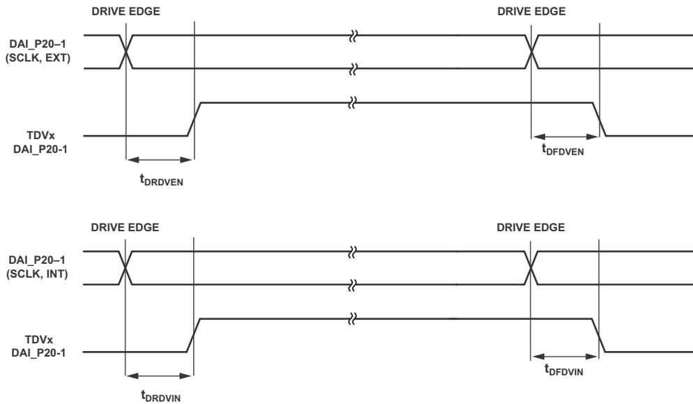
Figure 25. Serial Ports—TDM Internal and External Clock
