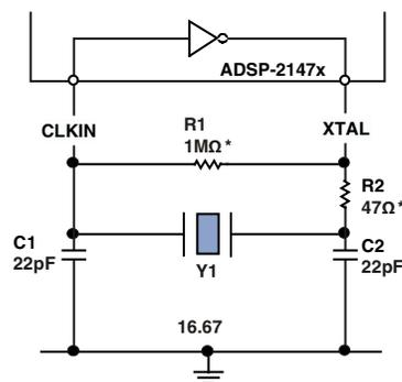
R2 SHOULD BE CHOSEN TO LIMIT CRYSTAL DRIVE POWER. REFER TO CRYSTAL MANUFACTURER'S SPECIFICATIONS
