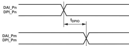
Figure 16. DAI Pin to Pin Direct Routing
