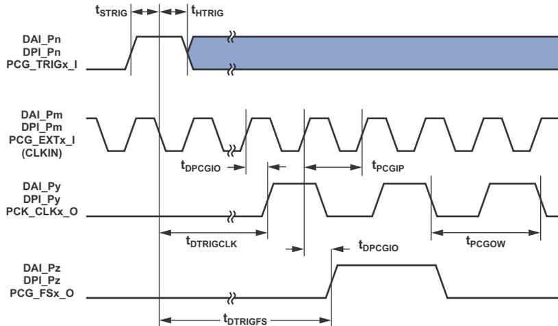
Figure 17. Precision Clock Generator (Direct Pin Routing)
