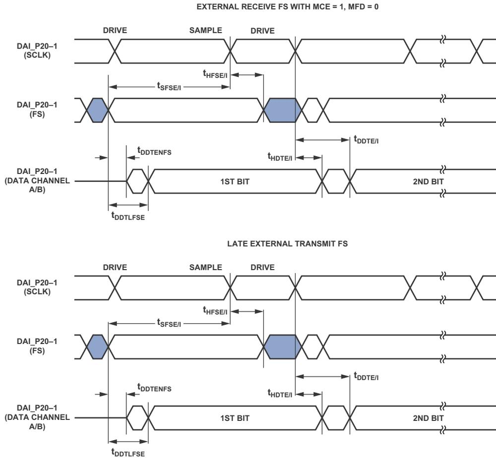
Figure 23. External Late Frame Sync<sup>1</sup>
