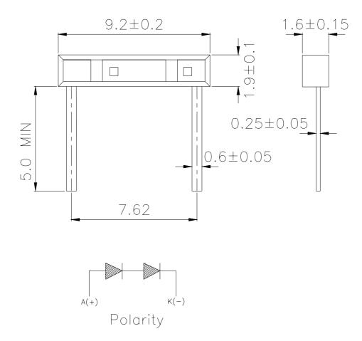
Notes: All dimensions are in millimeters. Tolerances unspecified are±0.1mm.
