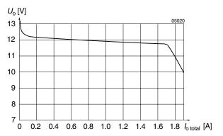
Fig. 8  $U_{01/2}$  versus  $I_{01/2}$  of double output power trains (i.e.  $2 \times 12$  V). See: Block diagram 1
