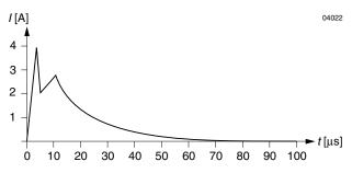
Fig. 3 Typical inrush current at  $U_{\text{i nom}}$ ,  $P_{\text{o nom}}$  versus time. Source impedance according to prETS 300132-2, version 4.3 at  $U_{\text{i nom}}$ .
