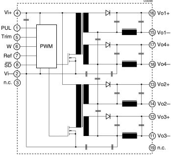
Fig. 2 :-----Block diagram 3, quadruple output types
