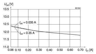
Fig. 9 Cross load regulation  $U_{04}$  versus  $I_{01}$  (typ) for various  $I_{04}$  for Vo1, Vo4 on power train 1. See: Block diagram dual output types. (IMY 35 D12D12-9)
