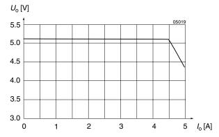
Fig. 7  $U_0$  versus  $I_0$  (typ) of units with  $U_0 = 5.1$  V.
