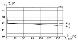
Fig. 10 Flexible load distribution on power train 1 of IMY 35 D12D12-9 (4  $\times$  12 V) with load variation from 0...150% of P<sub>01 nom</sub> on output 1 (Vo1). Output 2 (Vo4) loaded with 50% of P<sub>04 nom</sub>.
