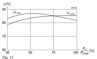
Efficiency versus input voltage and load. Typical values IMY 35 D12D12-9
