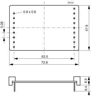
Fig. 18 Case IMY 35 open frame (option Z) Weight: 43 g
