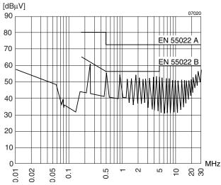
Fig. 15 Typical disturbance voltage (quasi-peak) at the input according to CISPR 11/EN 55011 and CISPR 22/EN 55022, measured at U<sub>i nom</sub> and I<sub>o nom</sub>. Output leads 0.1 m, twisted. (IMY 35-D12D12-9)
