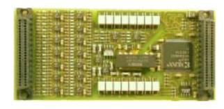
All inputs have an electronic debounce circuit. The debounce time is programmable in a range from 900µs up to 230ms in 256 steps of 900µs. The debounce circuit can also be disabled. The TIP606 is designed for an operating temperature from -40°C to +85°C.
