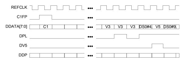
Figure 11 illustrates the operation of the SBI DROP BUS, using a negative justification on the second to last V3 octet as an example. The justification is indicated by asserting DPL high during the V3 octet. The timing diagram also shows the location of one of the tributaries by asserting DV5 high during the V5 octet.
