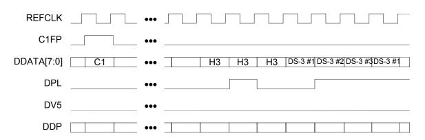
Figure 12 shows three DS-3 tributaries mapped onto the SBI bus. A negative justification is shown for DS-3 #2 during the H3 octet with DPL asserted high. A positive justification is shown for DS-3#1 during the first DS-3#1 octet after H3 which has DPL asserted low.
