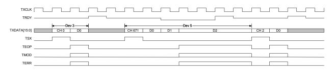
Figure 21 shows two special conditions -(1) the transfer of a one word packet illustrating how the external controller must wait until TRDY has been sampled high before the next data transfer can begin, and (2) the transfer of a packet which completes when TRDY is set low illustrating that although the packet has been completely transferred, the external controller must still wait until TRDY has been sampled high before the next data transfer can begin.
