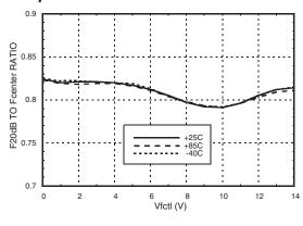
High Side Rejection Ratio vs. Temperature [1]
