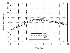
Maximum Return Loss in a 2 dB Bandwidth vs. Temperature
