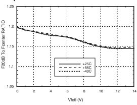
[1] Rejection ratio is defined as the ratio of the frequency at which the relative insertion loss is 20 dB to fcenter
