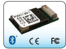
(API), antenna, *Bluetooth* transceiver, SPP Profile, FCC and IC certifications and *Bluetooth* end product listing. Using Panasonic's exclusive "tiny footprint" technology, incorporating a Surface Mount Device (SMD) Land Grid Array (LGA) package, the **PAN1321i Series** is just 15.6 mm by 8.7 mm! A fully shielded case protects the transceiver from nearby RF emitters, simplifying PCB layout. The **PAN1321i** is qualified to the *Bluetooth* 2.0 standard.
