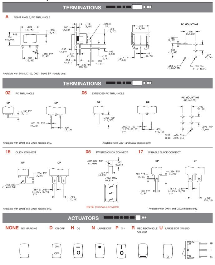
'D, H, P & U' marking options: marking color white, standard for all actuator colors except white. Black marking color, standard for white actuators. 'R & N' marking option: red marking color, standard. Consult Customer Service Center for other available marking colors.
