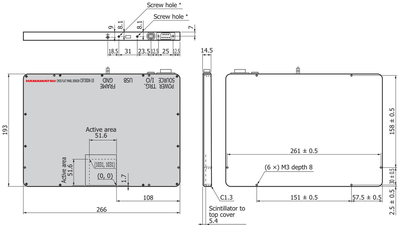
Top cover material including window is carbon fiber (1.0 mm thickness).
