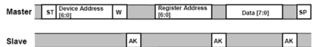
Figure 9. Single Byte Write - The Master (MCU) is writing to a single register of the MMA7450L
