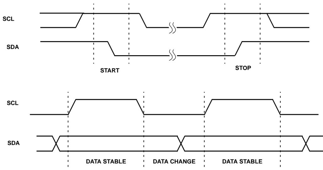
FIGURE 6. VALID DATA CHANGES, START AND STOP CONDITIONS
