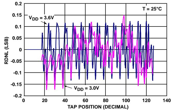
FIGURE 4. RDNL vs TAP POSITION FOR 10kΩ (W)
