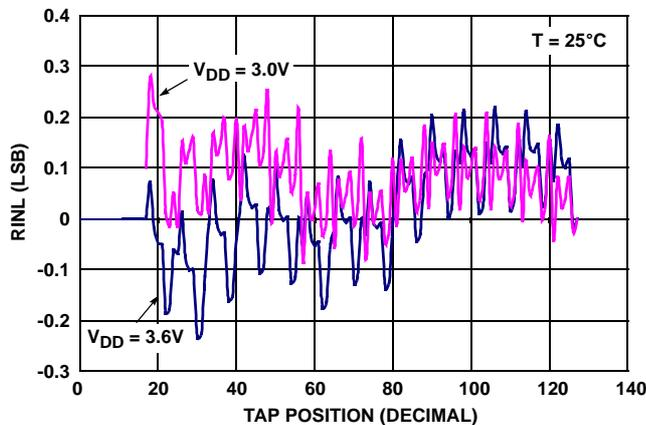
FIGURE 5. RINL vs TAP POSITION FOR 10kΩ (W)
