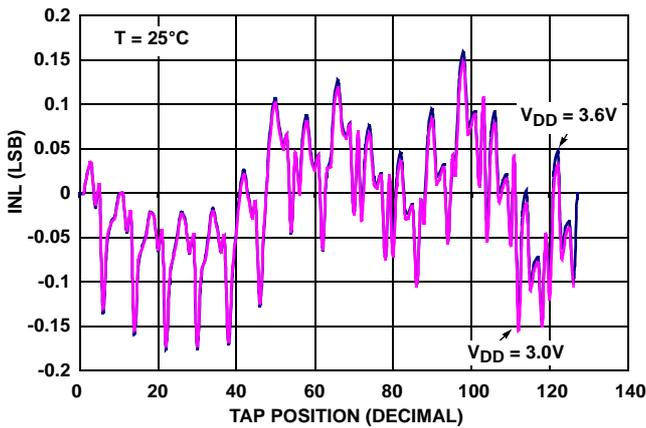
FIGURE 3. INL vs TAP POSITION FOR 10kΩ (W)
