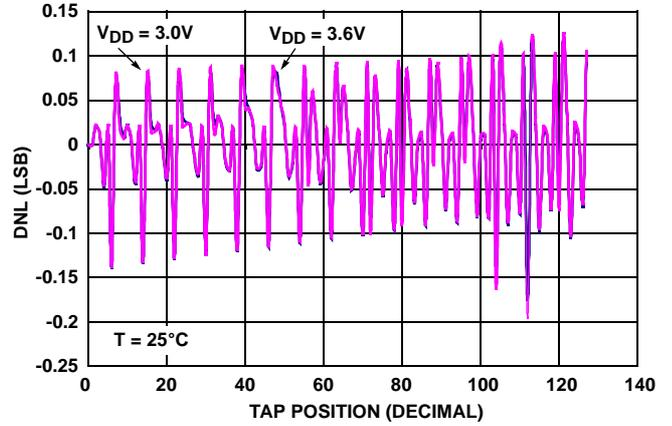
FIGURE 2. DNL vs TAP POSITION FOR 10kΩ (W)
