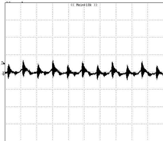
Figure 14: Output voltage ripple at nominal input voltage and rated load current ( I_o=40\text{A} ) (20 mV/div, 2µs/div) Load capacitance: 1\mu\text{F} ceramic capacitor and 10\mu\text{F} tantalum capacitor. Bandwidth: 20 MHz. Scope measurements should be made using a BNC cable (length shorter than 20 inches). Position the load between 51 mm to 76 mm (2 inches to 3 inches) from the module.
